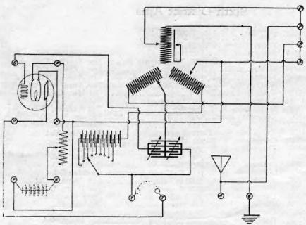
Hookup of Disc Core Receiver for Undamped Waves
