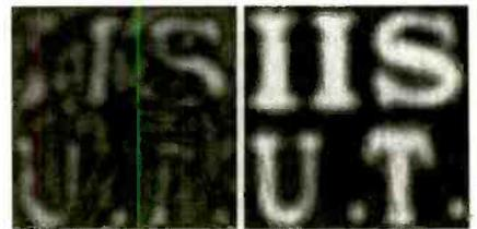
Fig. 4. The initials in the normal ultrasonic image (on the left) are distorted so much that they can hardly be read, while the initials in the time-reversal wave image on the right are clear.
