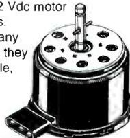
0.31" (5/16") diameter shaft is 1.2" long. No load Rating: 2200 RPM @ 12 Vdc @ 2.8 Amps. Weight: 3.25 lbs. 0.25" quick-connect terminals.
