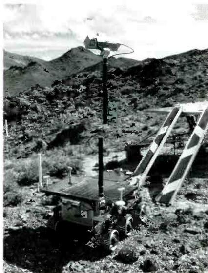
Having just rolled off his flatbed truck, FIDO is ready to explore the Nevada desert as part of an ongoing field test that simulates robotic exploration on other planets.
