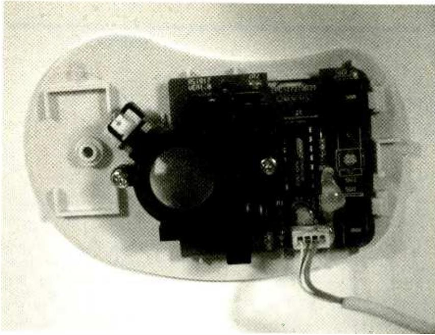
*This is a close-up view of a photodiode (labeled IR2). This photovoltaic device provides the input for the optical encoder of a standard mouse (see section on "Sensors"). Two sensors are used; one detects horizontal movement of the mouse and the other detects vertical movement of the mouse*
