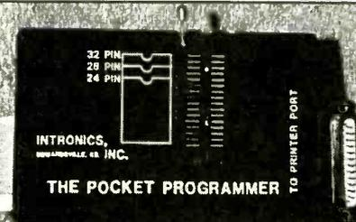
The portable programmer that uses the printer port of your PC instead of an internal card. Easy to use software that programs Eprom, EEprom, Flash & Dallas Ram. 27(C) / 28(C) / 28F / 29F / 29C & 25XX series from 16K to 8 Megabit with a 32 pin socket. Adapters available for Pic, PLCC, 5-Gang, 874X, 875X MCU's, 40-Pin X 16 & Serial Eprom's, 82/74 Prom's and Eprom Emulator to 32K X 8.
