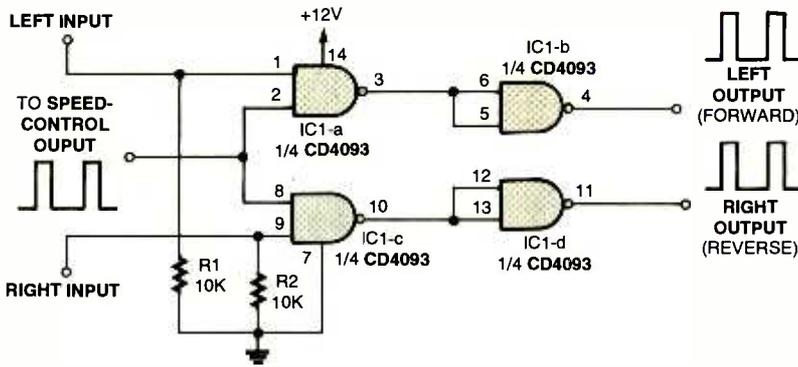
Fig. 6. Adding this circuit to the circuit in Fig. 5 lets you steer the output pulses between two different outputs—individually or together.
