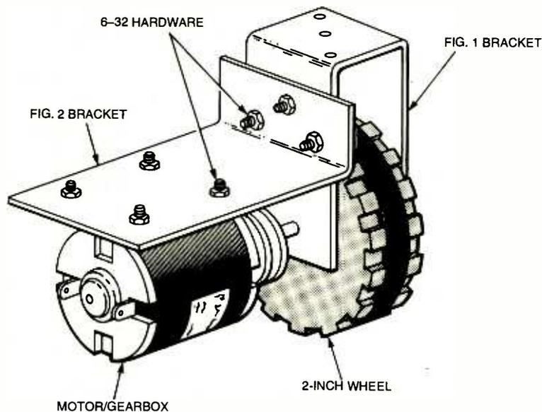
Fig. 3. Here is what the front wheel looks like when fully assembled.
