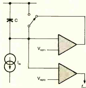
Fig. 6. This simplified model of a voltage-controlled oscillator (VCO) illustrates the principles behind the circuit built around IC3.
