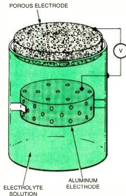
Fig. 2. An aluminum-air battery absorbs oxygen from the air through a porous electrode to enhance the chemical reaction and, therefore, the power output.
