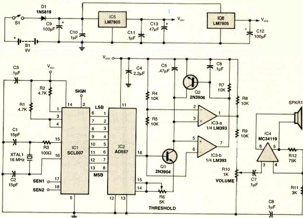
Fig. 5. The Fluxgate Magnetometer is a simple circuit, thanks to a sophisticated interface chip from Speake that handles all the messy "behind-the-scenes" work when dealing with fluxgate sensors.
