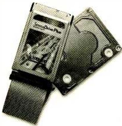
Kingston's StrataDrive Plus comes with a PC-Card interface, letting you transfer the operating system and applications to the new drive without strain or pain.
