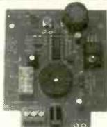
Build this kit and detect combustible gases and vapors including natural gas, gasoline, propane, and dozens more. Model GLD1000 is a local alarm only, GLD1010 includes a relay to control external alarms.
