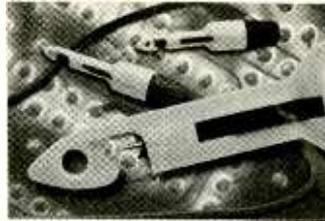
A rotating banana jack prevents the test lead from twisting while the wire is pierced. The small, easily attached clips can access individual wires within large bundles.
