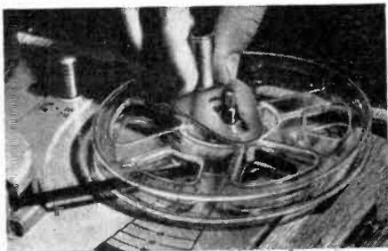
sturdy metal device holds the tape to the reel for the first few turns to get the winding started. Then, it can either be slipped off or left in position to serve as a reel
