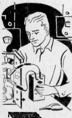
Completed substitution box in actual use to determine the best value for a replacement resistor in a receiver. Slide switch is down in the "Lo" position. The lower switch knob is being turned to put different resistors into circuit.
