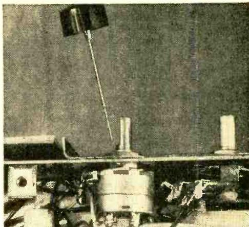
Noise in the speaker as the volume control is rotated can often be cleared up by injecting a few drops of carbon-tet. Run the carbon-tet down the shaft of the control. Rotate the control to spread the cleaner. If the noise continues, replace the control.
