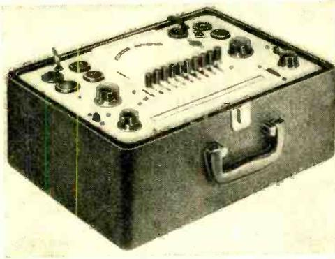
**T**HE new *Knight* tube tester kit is easy to build and measures tube performance by the cathode-emission method. It also checks for shorted elements, open elements, and heater continuity. It will test 4-, 5-, 6-, and 7-pin large, regular, and miniature
