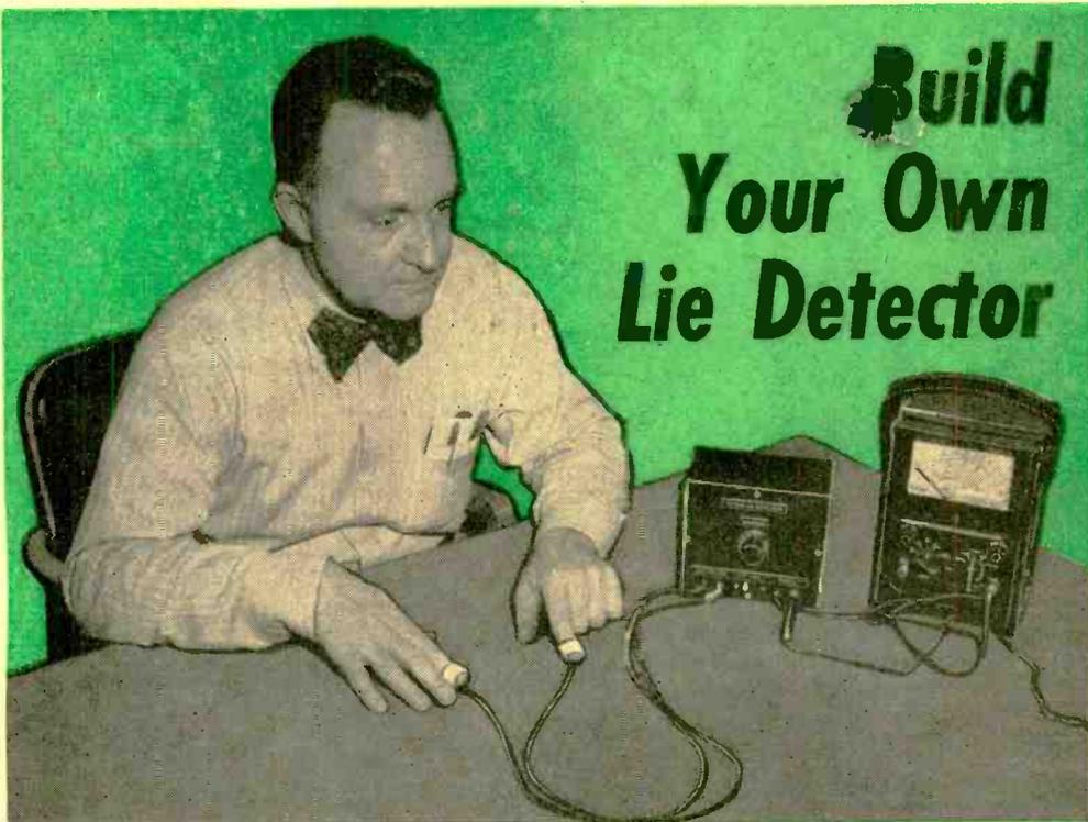
INTERESTED in a gadget to take to a party? How about something for the classroom? Studying experimental psychology? Want to see what else can be done with electronics? Then here is an interesting answer. A simple circuit consisting of one tube, three batteries, four resistors, and one potentiometer that will convert a v.t.v.m. into a lie detector.
