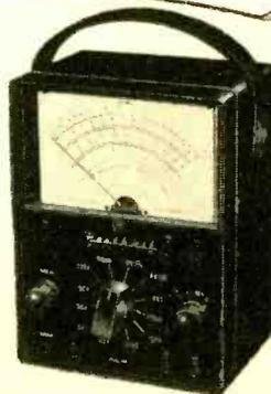
Here is an instrument packed with every desirable service feature and all of the measurement ranges you need or want. High sensitivity 20,000 ohms per volt DC, 5000 ohms per volt AC. Has the advantage of complete portability through freedom from AC line—provides service ranges of direct current measurements from 150 microamperes up to 15 amperes—can be safely operated in RF fields without impairing accuracy of measurement.
