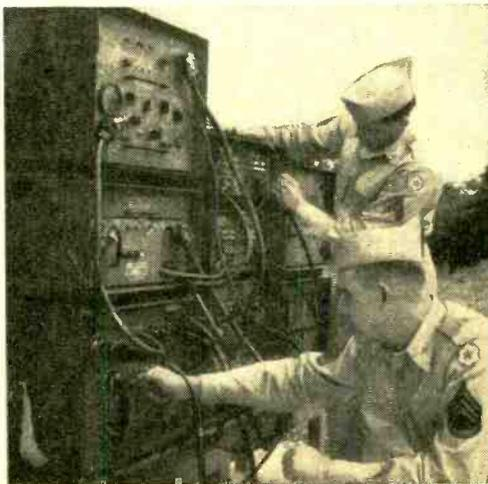
can be credited with the sharp reduction in size and weight of the new equipment. The earlier, four-channel unit, for example, weighed 475 pounds and occupied twenty cubic feet of space. Complete with its power supply, the new four-channel terminal weighs 178 pounds and occupies only five and a half cubic feet of space. The cable used for the systems can be strung on poles, laid on the ground, or buried.
