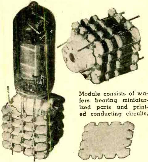
Module consists of wafers bearing miniaturized parts and printed conducting circuits.
