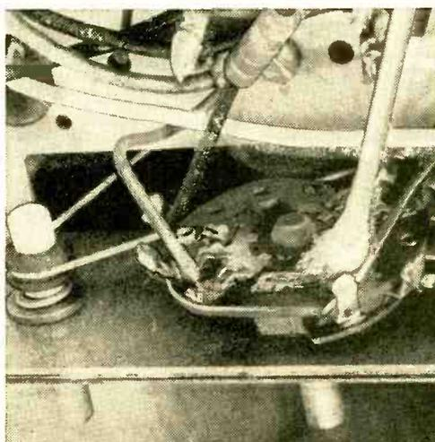
Dirt and dust may also affect the selector or bandswitch. Generally speaking, the control may be cleaned with a few drops of carbon-tet on a pipe cleaner wiped across the contacts.
