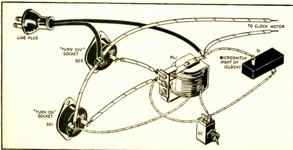
the "Turn Off" socket. It will operate there until the clock reaches the pre-set time and then be cut off. For example, an exhaust fan can be connected in this manner, with  $S_2$  set to "Hold." When the clock reaches the shut-off time, the fan is stopped and kept turned off indefinitely.
