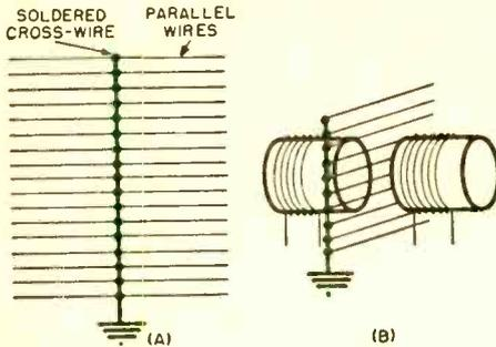
of shield is fabricated by gluing parallel wires to a cardboard sheet, spacing the wires apart by a distance equal to about two wire diameters. After the glue has set, a bare copper wire or strip is soldered across the rows at right angles; the assembly is then run to the common ground of the equipment.
