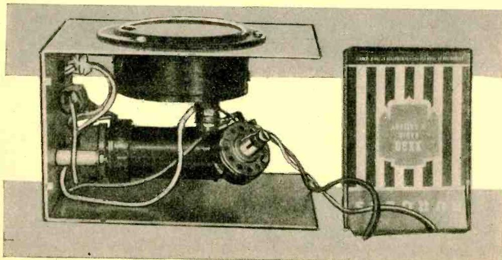
on the relay socket are used as tie points. The rheostat is supported by stiff bus-bar leads attached to the meter terminals. If this rheostat is mounted in the conventional manner with the shaft protruding through the case, the calibration may be accidentally destroyed. Be sure to knot the relay coil wires leaving the box to provide strain relief.
