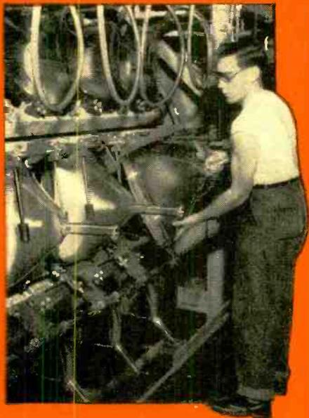
The first step in actual processing of a picture tube is screening, in which the phosphor picture screen is applied to the inside of the bulb's face. Note screens inside tubes at left. Hoses (top) pour one mixture into bulb, other comes later.
