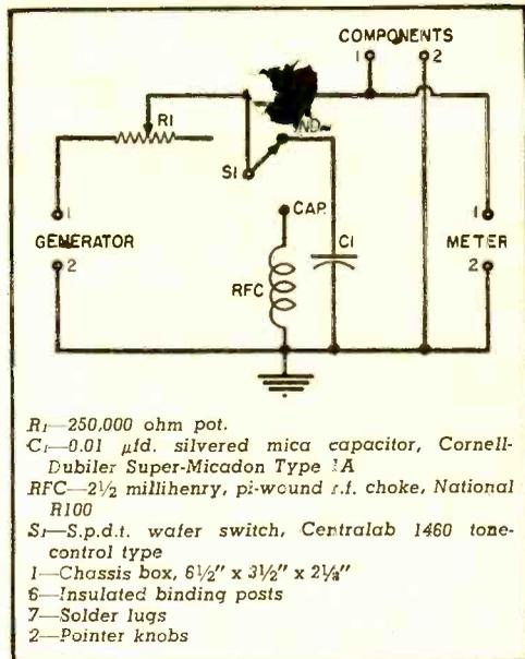
Fig. 1. (Above) Wiring schematic of the adapter. Note that capacitor C<sub>1</sub> is a silvered mica. (Below) Bottom view showing the layout of the components.
