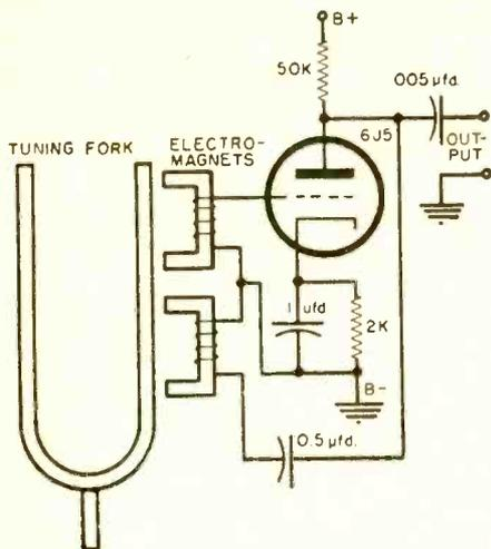
it becomes the "tank" circuit and is kept vibrating at constant amplitude by the interchange of magnetic effects in the electromagnet coils.
