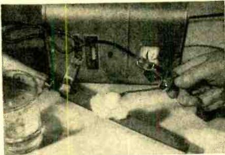
per wire. Wrap a wad of absorbent cotton around the free end of the wire and dip it into a salt solution. Apply to the file, being careful not to touch the file with any portion of the copper wire except the end wrapped in cotton. This would short-circuit the d.c. source. When contacted by the cotton, the file will be subject to a rapid release of hydrogen gas which lifts cuttings and other foreign matter from between the file's teeth. Following this, rinse, dry, and oil the file immediately.
