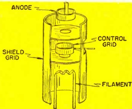
Fig. 1. Internal construction of thyatron.
