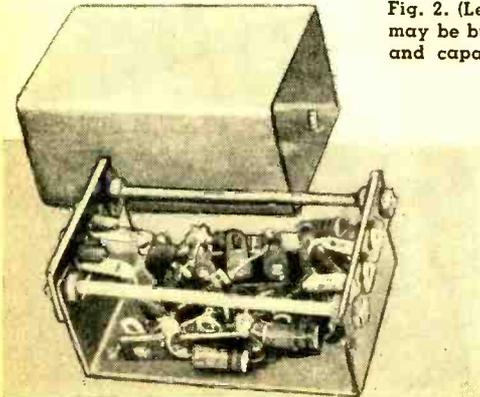
Fig. 2. (Left) The circuit shown in the schematic below (Fig. 3) may be built into an old i.f. transformer can. The resistor chokes and capacitors are mounted on five-point terminal tie strips.
