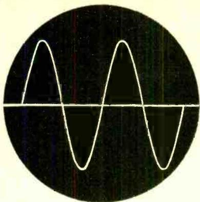
Fig. 1. Waveform of pure sine wave as seen on an oscilloscope screen.
