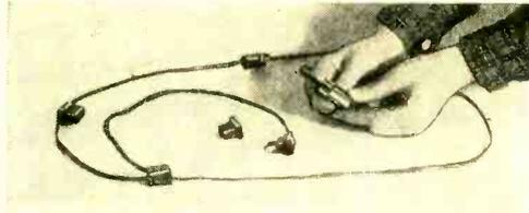
the total of the current drawn at any one time through such a multiple-outlet cord does not exceed 7½ amperes. A close-enough figure for this amperage can be obtained by dividing the power consumption in watts of each unit by the line voltage, usually 117 volts. A total of under 800 watts should be safe. In using such a cord, make sure other appliances connected to the same line elsewhere do not exceed the safe rating for the circuit.
