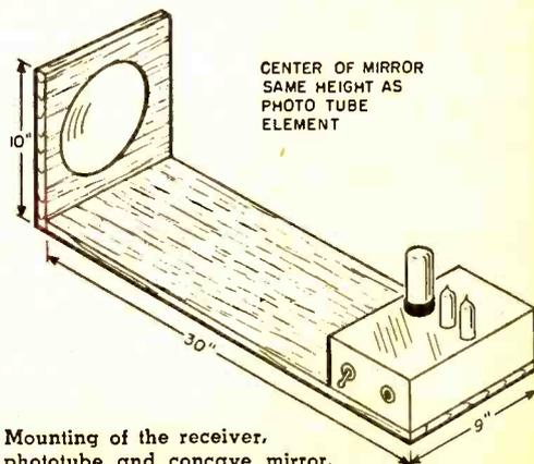
Mounting of the receiver, phototube and concave mirror.
