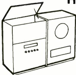
Model 80 has lift lid, removable panels. Bass reflex tuned for 12" or 15" speakers. Overall dimensions: 33½"H, 23"W, 16"D. M80 tuner section, inside: 20"H, 21¾"W, 15½"D. M8112, M8115 baffle volume: 6 cubic feet. ¾" white pine
