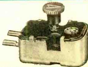
cartridge is unaffected. Ceramic cartridges have a high output and a high terminal impedance; their circuit requirements are as simple as those of crystal pickups. A ceramic cartridge designed for proper stylus compliance gives very good results with great economy of means. It is not surprising, therefore, that ceramic cartridges have steadily grown in popularity during the short time that they have been on the market.
