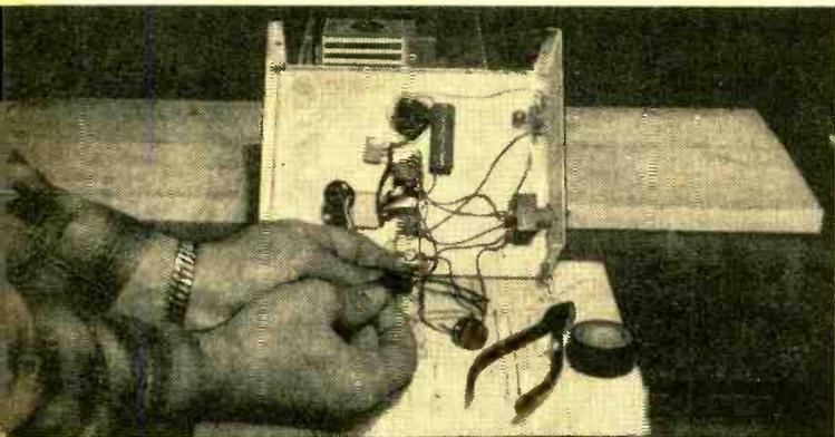
After wiring the battery plugs, cover their backs with plastic tape to prevent short circuits if the plugs should touch the cabinet. Unit is completely wired here—note the grid-bias resistor on the "B" battery plug.
