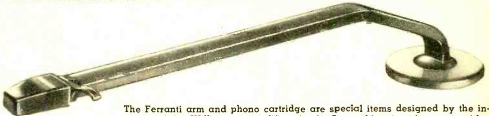
The Ferranti arm and phono cartridge are special items designed by the inventor of the Williamson amplifier circuit. A matching transformer provides about 15-mv. output. Frequency response is within  $\pm 1.0$  db from 20 to 20,000 cycles. Arm and cartridge track at recommended stylus pressure of 3 grams.
