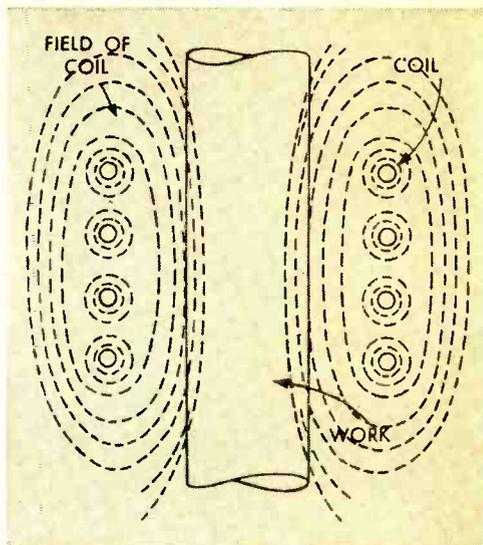
The effect of the electromagnetic field produced by loading the coil is shown above.
