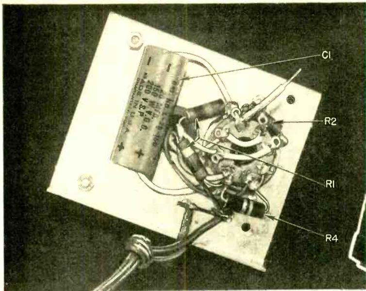
(Left) Subchassis viewed from underneath with the majority of components in place. (Below) Plug with wire soldered to one prong, forming a polarized plug.
