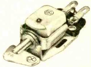
Electro-Sonic cartridges have a frequency range of 20 to 10,000 cycles with a perfectly flat response. The curve then rises gently to about + 1.5 db at 15,000 cycles and 2 db at 20,000 cycles. Output is extremely low, measuring about 1 mv. at an output impedance of 1.5 ohms. The minimum stylus force may be as low as 3 grams. Diamond or sapphire needles are available from the manufacturer.
