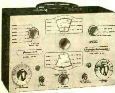
**R. F. SIGNAL GENERATOR:** The Model TV-50 Genometer provides complete coverage for A.M. and F.M. alignment. Generates Radio Frequencies from 100 Kilocycles to 60 Megacycles on fundamentals and from 60 Megacycles to 180 Megacycles on powerful harmonics.
