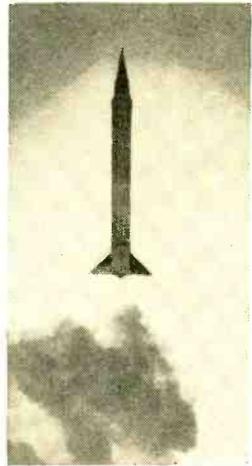
physical characteristics of the ionosphere, gathering information on how radio waves are transmitted. During its trip it took photos and conducted many experiments—with no human being on board. Made by *Martin Aircraft* of Baltimore, Md., this rocket reached a speed of about 4100 miles an hour. It weighs 7 1/2 tons and is 45 feet long.
