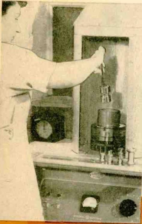
checking the physical dimensions of metal parts where only one end or side may be reached.
