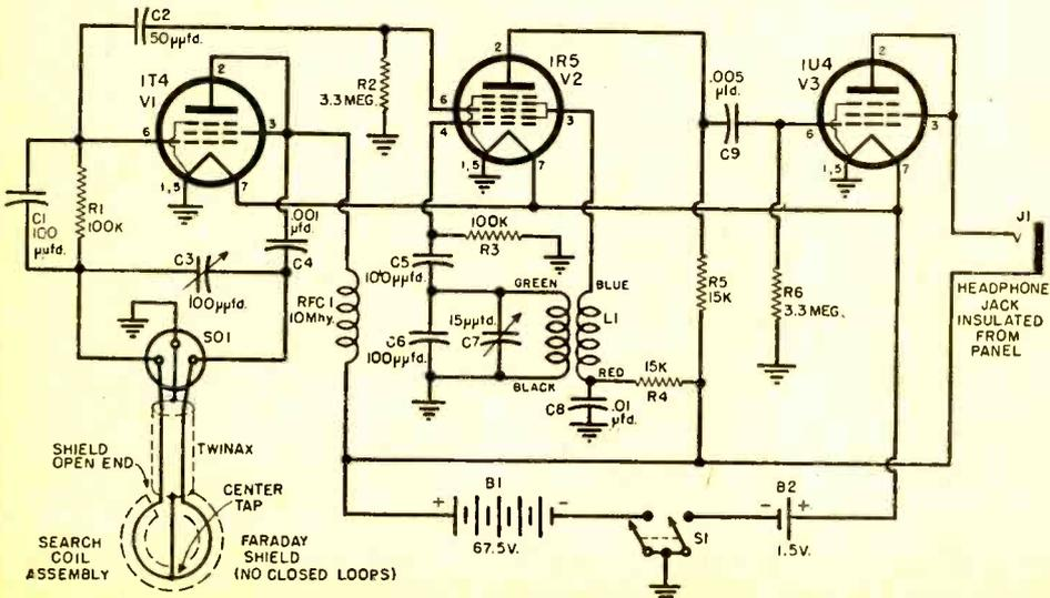
is highly undesirable, a shield must be built which permits the movement of magnetic lines of force without permitting capacitive coupling. Such a shield is called a Faraday shield; it must have no closed loops or current paths in which eddy currents can flow. Neither metal foil nor copper screening is satisfactory because these are full of closed loops which cause serious magnetic field losses, reducing the penetration of the field so that the device becomes insensitive.
