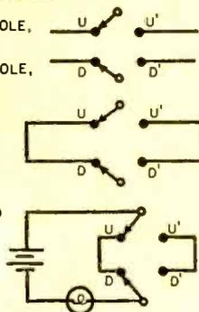
This diagram shows how Geniac solves "the problem of the hall light." Verbal statements are broken down into algebraic symbols which, in turn, indicate the number and type of circuit components required.
