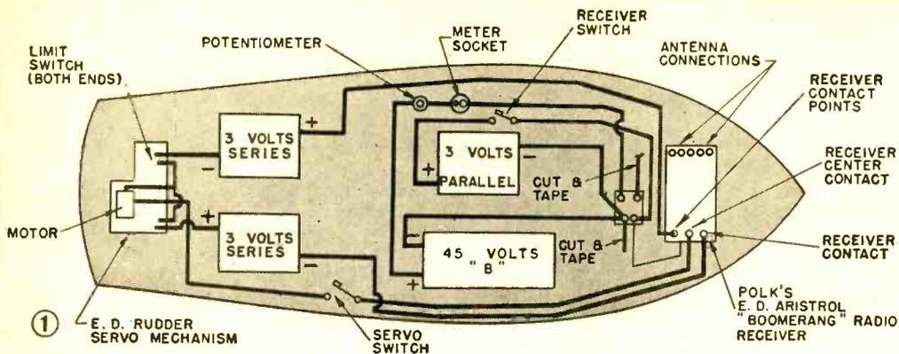
① Block diagram of E.D. radio receiver and rudder servo wiring for typical installation.
