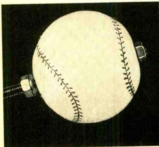
Fig. 4. A winged nut on the threaded shaft permits rotation of the clamp holding arm.
