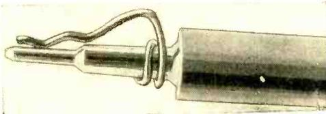
the circuit. The part that is wound around the test prod may be soldered to it, making a permanent installation. The part so used should be wound on a slightly smaller diameter prior to slipping it on the test prod; it may be expanded slightly for a tight fit.
