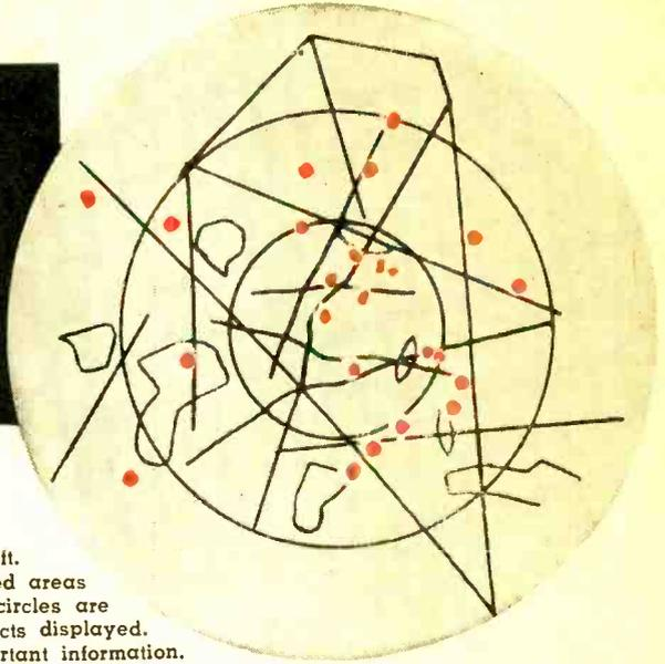
Dots represent moving aircraft. Straight lines show prohibited areas or flight paths. Concentric circles are distances from radar to objects displayed. Color distinguishes the important information. This presentation is called "Plan Position Indicator."
