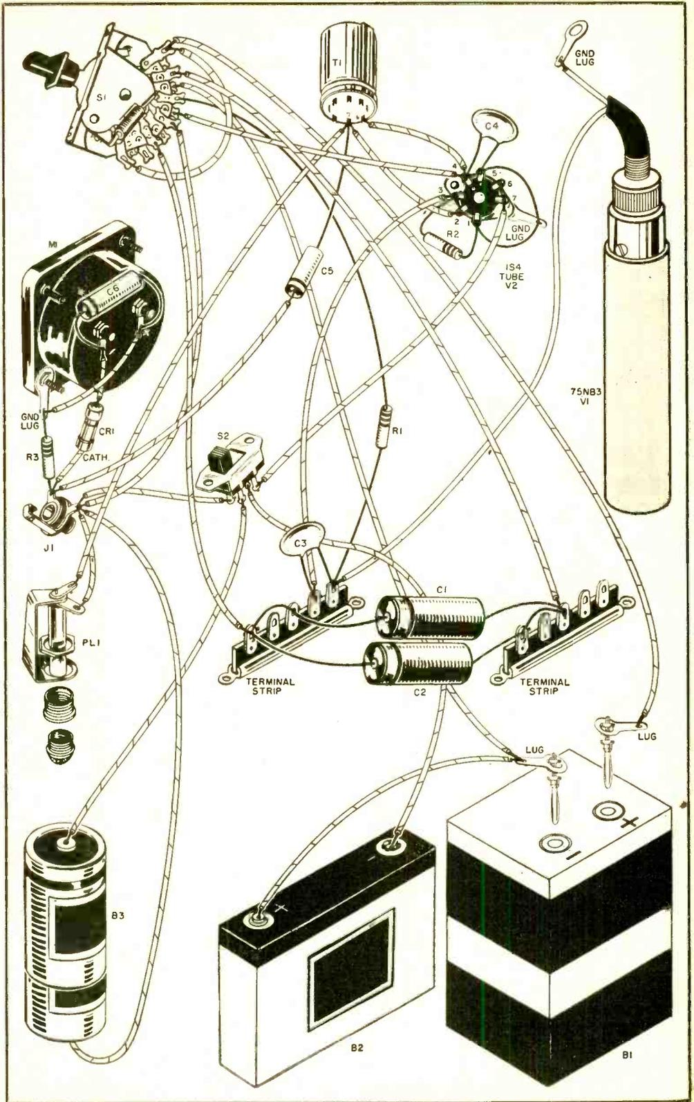
switch which charges the capacitor and upon release connects it in series with the battery. A capacity of two microfarads ( $C1$  and  $C2$  in parallel) is sufficient to operate the tube for several minutes.
