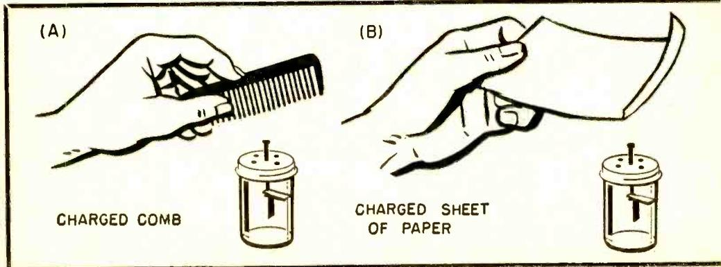
needle will show the presence of a magnetic field. When the electrode of the electro-scope is touched to an electrically charged object (or, in some cases, simply brought near it), the gold leaf will move away from the metal bracket. High voltages will swing the leaf over the greatest distances.
