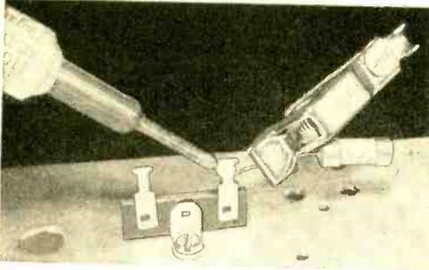
age to an expensive component. One technique is to hold the lead wire with a pair of pliers, but this requires "three hands"—one to hold the solder, one to hold the pliers, and one to hold the pliers. A good substitute method is to fasten a heavy metal clip to the lead wire in place of the pliers. A thick copper clip is best. It makes an excellent heat sink and is not only easy to use but quite inexpensive.
