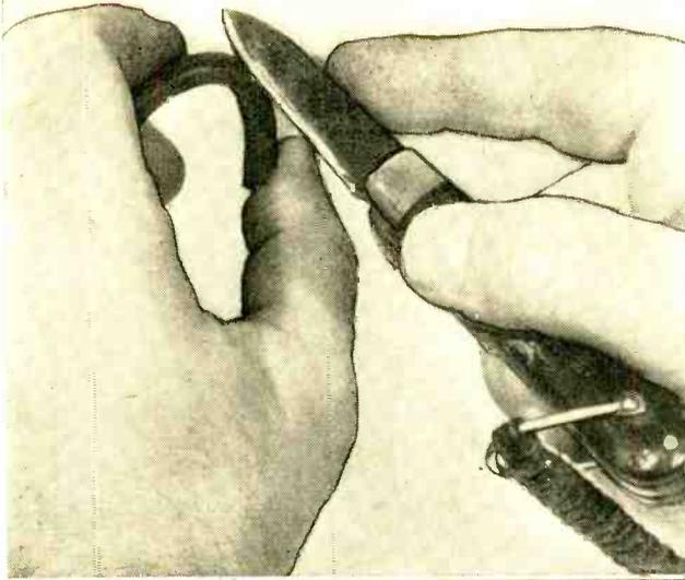
To remove cambric cover from shielded cable, carefully cut down to the metal braid completely around the cable. Grip the insulation with pliers and tear off, trimming edge if necessary. Sometimes it is easier to cut the cambric from the cable end to the circular cut and strip off.
