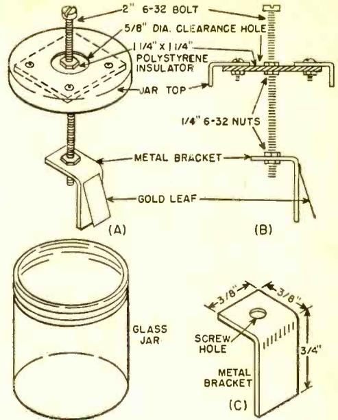
Fig. 1. In assembling the electro-scope, the author used an empty peanut jar. The cardboard insert in the lid is removed and a hole is cut in the center of the metal lid. A small square of polystyrene is then mounted under this hole and a 2"-long bolt fastened through the center. At one end, mount the metal angle bracket shown in (C). Glue the gold leaf to the bracket just beyond the bend as shown in (A) and (B).
