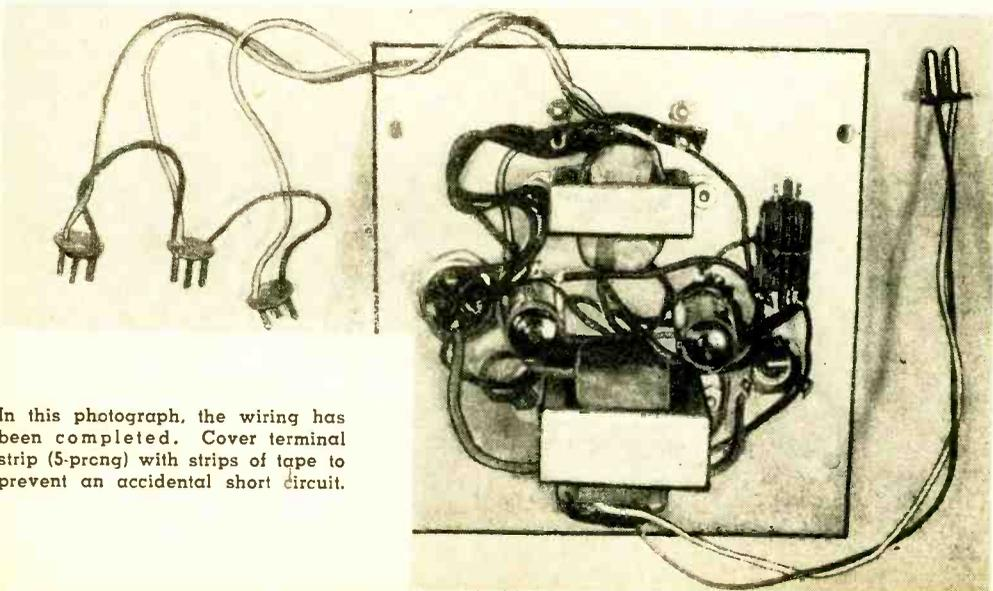
In this photograph, the wiring has been completed. Cover terminal strip (5-prong) with strips of tape to prevent an accidental short circuit.
