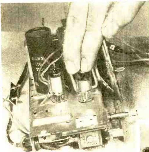
Other parts, such as capacitors and resistors, may be roughly checked with an ohmmeter by disconnecting one terminal. Try a few new components to learn about what to expect of good equipment so that you can recognize a faulty component when it turns up in your portable. —30—
