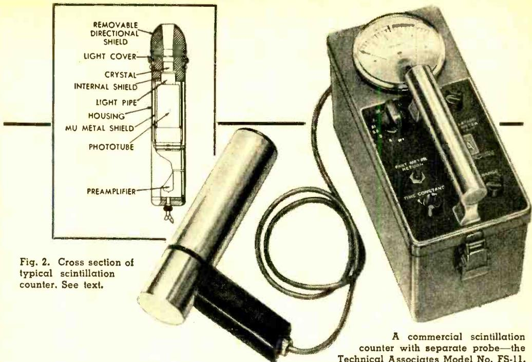
Fig. 2. Cross section of typical scintillation counter. See text.
