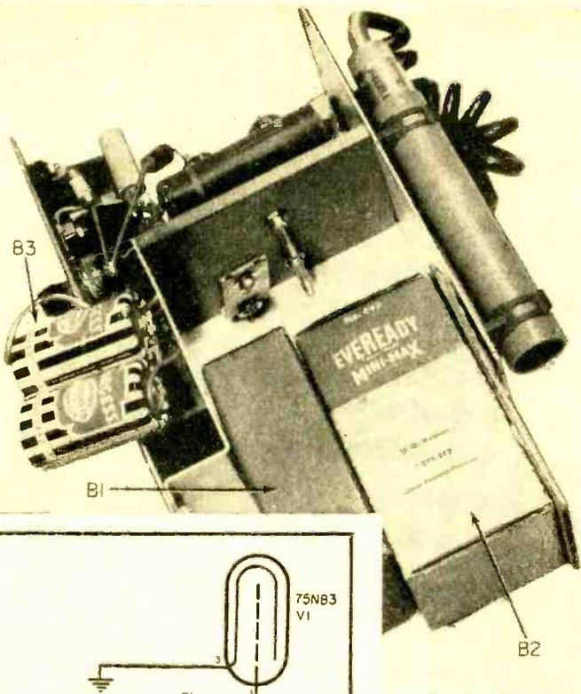
Interior view of battery compartments. A battery plug is used for B1, banana plugs for B2, and the two flashlight batteries (B3) are wired directly into the circuit.
