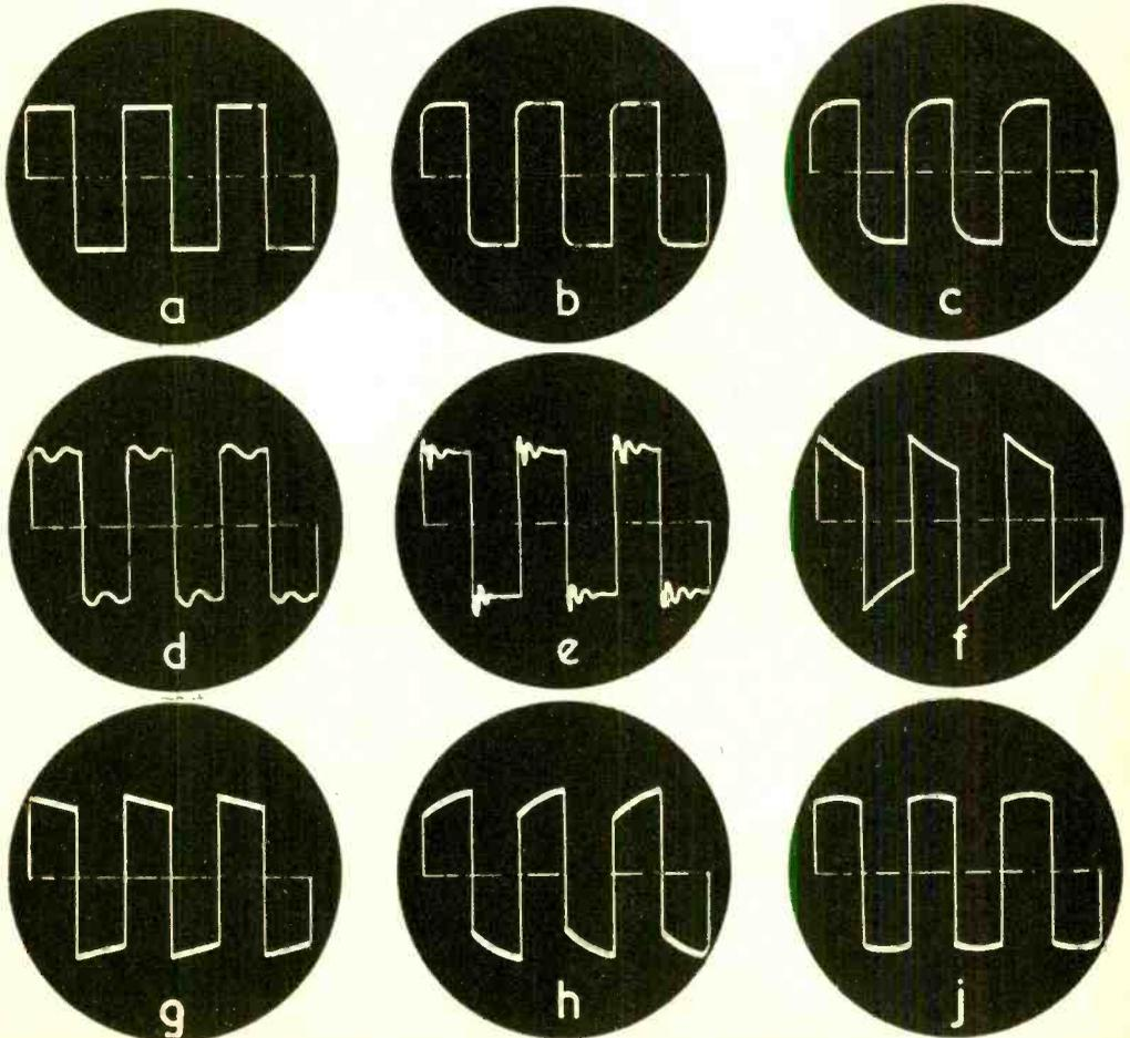
Fig. 4. To determine the presence of transient distortion, a high frequency audio wave in (a) is being switched off and on at regular intervals. The pattern is essentially square. In trace (b), the same wave pattern is shown after passage through a hi-fi system having a small amount of transient distortion.
