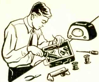
**M**INOR defects, amendable by the owner, often occur in small radios. The faults and correction techniques illustrated in the photographs on these pages can usually be handled by someone with some electronic knowledge. The radio used as the "guinea pig" is a *Sentinel* Model 335P a.c.-d.c.-battery portable with a 4½-volt "A" battery and 90-volt "B" battery, drawing 35 watts on a.c.
