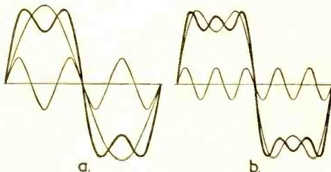
Fig. 2. This is a demonstration of phase in waveshaping. Part (a) is identical to (a) above, but in (b) of this drawing the timing, or phase, of the third harmonic has been slightly shifted. The resultant wave drawn as the heavy line is now quite a different shape and could not be classed as a useful square wave for testing hi-fi equipment.
