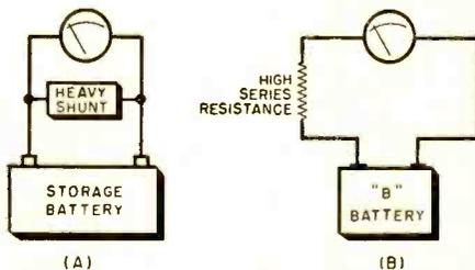
most of the standard types having three cells in series; 12 volts for batteries found in new cars) under a short-period drain of 300 amperes or more, it cannot be depended upon to start the engine, especially under the conditions imposed upon it in freezing weather. To check a battery under such a condition, an instrument like
