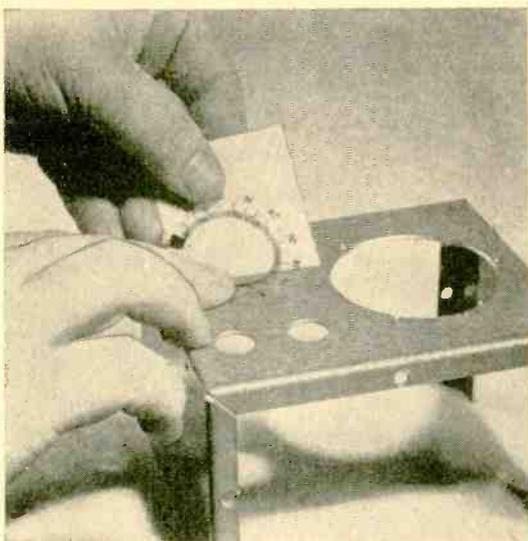
**5** In a few seconds the decals will come loose from their backings. Moisten the equipment to be labeled, then slide decals into place.
