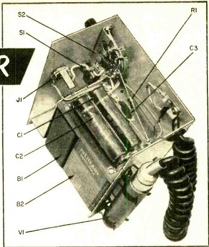
Interior view of the de luxe unit. Refer to the schematic of Fig. 2. Increased headphone volume, a neon flasher, and a meter are features of this unit. Construction is somewhat more difficult than that of the simplified counter shown above and in Fig. 1.
