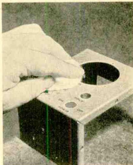
**6** Using a soft cloth, press decals firmly against panel and remove excess moisture. Be sure to remove all air bubbles.
