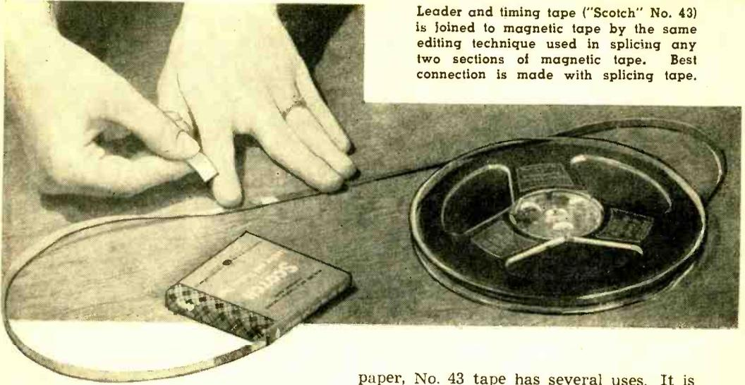
Leader and timing tape ("Scotch" No. 43) is joined to magnetic tape by the same editing technique used in splicing any two sections of magnetic tape. Best connection is made with splicing tape.
