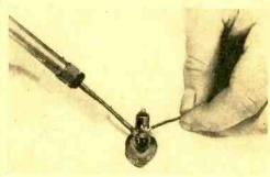
the advantage over a regular vise of not breaking brittle parts, such as those made of glass.
