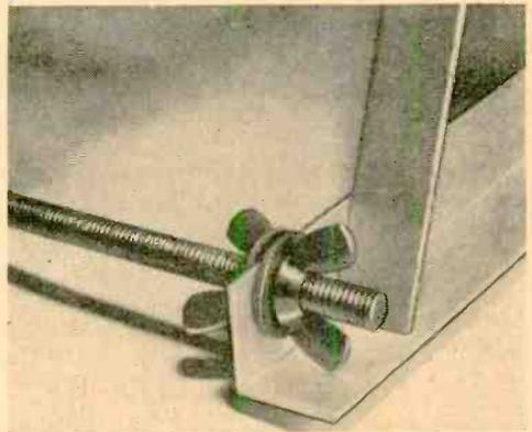
Fig. 6. A-frame and base assembly (above). Note that A-frame may be moved by loosening the wing nuts and setting them in a new position determined by the width or length of chassis held in the cradle. The use of washers under the wing nuts will prevent excessive scoring of A-frame.
