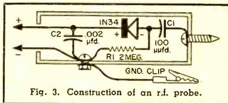
Fig. 3. Construction of an r.f. probe.
