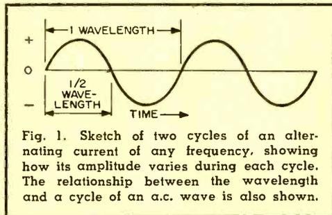
Fig. 1. Sketch of two cycles of an alternating current of any frequency, showing how its amplitude varies during each cycle. The relationship between the wavelength and a cycle of an a.c. wave is also shown.
