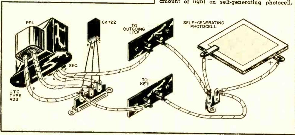
other power supply is needed. With the type of transformer shown and a B15 photocell, the tone frequency is about 2000 cycles in moderate sunlight. The frequency decreases as the lighting increases, and vice versa.
