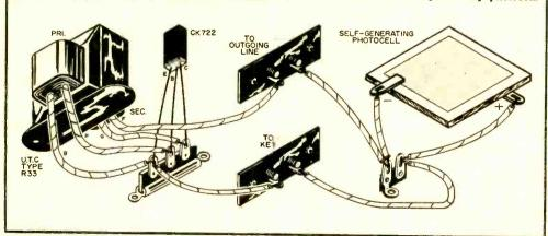
other power supply is needed. With the type of transformer shown and a B15 photocell, the tone frequency is about 2000 cycles in moderate sunlight. The frequency decreases as the lighting increases, and vice versa.
