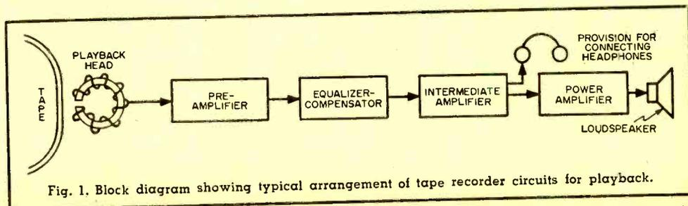
Fig. 1. Block diagram showing typical arrangement of tape recorder circuits for playback.
