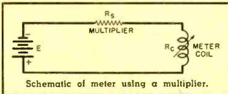
Suppose, for example, that a given meter movement is designed so that 1 ma. (.001 amp.) produces a full-scale deflection. To make it into a 0-1 volt voltmeter, a series
