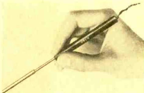
equipped with a  $\frac{5}{32}$ " pure nickel non-corrosive tip which can be easily replaced if necessary. For further details, write to the manufacturer's U. S. representatives: *Television Accessories Co.*, 1412 Great Northern Bldg., Chicago 4, Ill.
