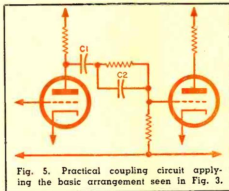
Fig. 5. Practical coupling circuit applying the basic arrangement seen in Fig. 3.
