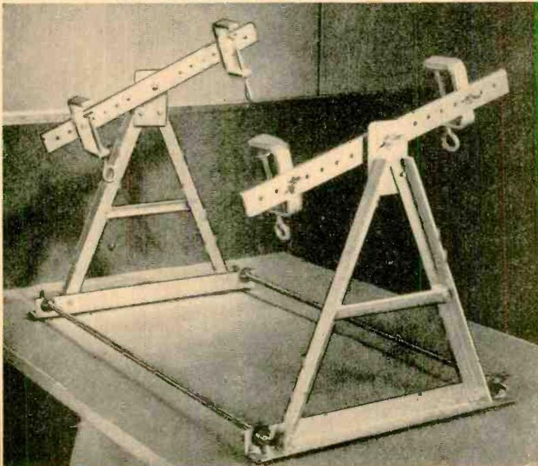
Fig. 7. Fully assembled chassis rack (left). "Handy Clamps" on the rocker arms hold the chassis, which may be swung around to permit working on either the top or the bottom. Vary the position of the A-frame on Redi-Bolts to fit different lengths and/or widths.
