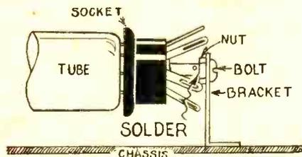
solder it into the contact. The bracket may then be bolted or soldered to the radio chassis.
