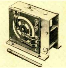
$1\frac{1}{2}$ " x  $1\frac{3}{4}$ " x  $1\frac{1}{8}$ " unit will enable you to obtain two speeds forward, stop, reverse, and start. It can handle 10 amperes at 6 volts through its rhodium-plated commutator.
