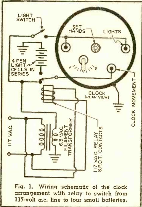
Fig. 1. Wiring schematic of the clock arrangement with relay to switch from 117-volt a.c. line to four small batteries.
