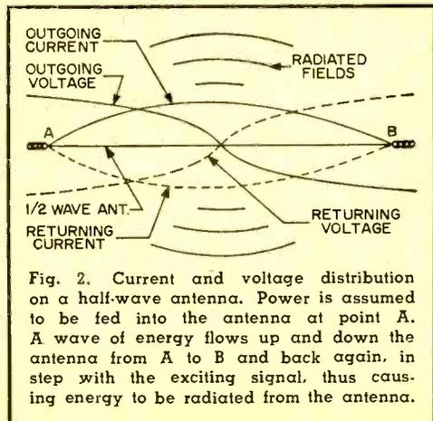
Fig. 2. Current and voltage distribution on a half-wave antenna. Power is assumed to be fed into the antenna at point A. A wave of energy flows up and down the antenna from A to B and back again, in step with the exciting signal, thus causing energy to be radiated from the antenna.
