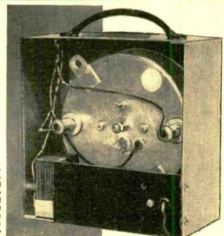
Relay, filament transformer, and four small batteries are mounted behind panel on rear of clock case. The two projections on back of clock are 6-volt lamps that illuminate the face. Such a clock can be taken on trips to isolated areas where a.c. power lines might fail.
