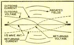
Fig. 2. Current and voltage distribution on a half-wave antenna. Power is assumed to be fed into the antenna at point A. A wave of energy flows up and down the antenna from A to B and back again, in step with the exciting signal, thus causing energy to be radiated from the antenna.
