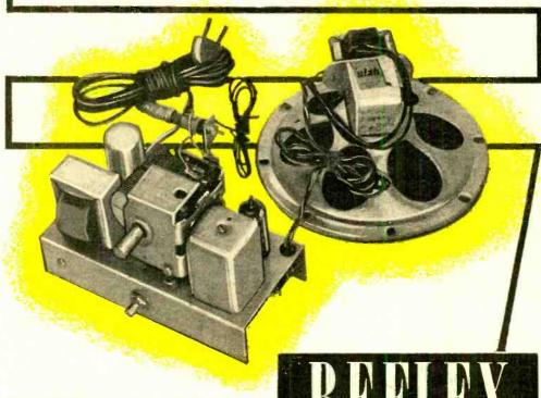
CONOMY of operation is featured in this little radio receiver. As it consumes about the same amount of power as an electric clock, continuous operation is practical. Maintenance cost should be negligible, for it has only one tube to wear out and the balance of the parts are operated at such a small fraction of their ratings that they should never require replacement.
