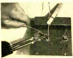
ing operation, you will appreciate this simple "kink." When you get your wire in the desired position, put some tension on it and clamp it in place with a spring-type clothespin. Use one for each wire if you are making a multiple connection.
