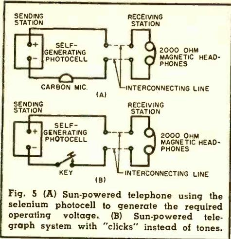
Fig. 5 (A) Sun-powered telephone using the selenium photocell to generate the required operating voltage. (B) Sun-powered telegraph system with "clicks" instead of tones.
