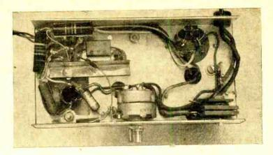
leads full length but coil them, corkscrew fashion, so that the diode just spans the distance between the coil and volume control terminals. Tin the ends gingerly, let them cool, then solder in place with a quick touch of the iron. Be sure the cathode or + end is attached to the coil terminal.
