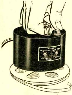
Complete erasure in a matter of minutes is provided by commercial "bulk erasers" such as those shown here. See text for details.
