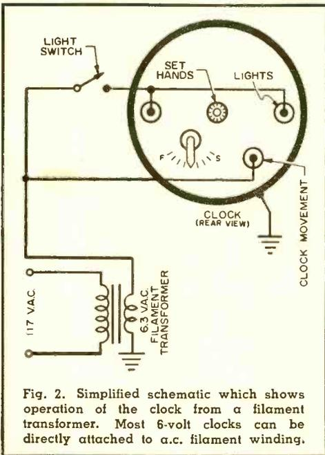
Fig. 2. Simplified schematic which shows operation of the clock from a filament transformer. Most 6-volt clocks can be directly attached to a.c. filament winding.
