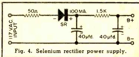
Fig. 4. Selenium rectifier power supply.
