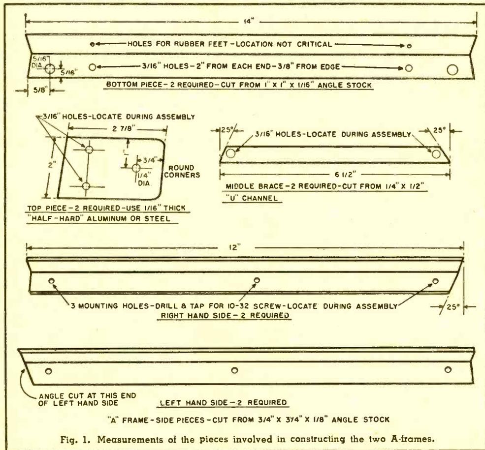
Fig. 1. Measurements of the pieces involved in constructing the two A-frames.
