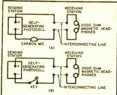
Fig. 5 (A) Sun-powered telephone using the selenium photocell to generate the required operating voltage. (B) Sun-powered telegraph system with "clicks" instead of tones.
