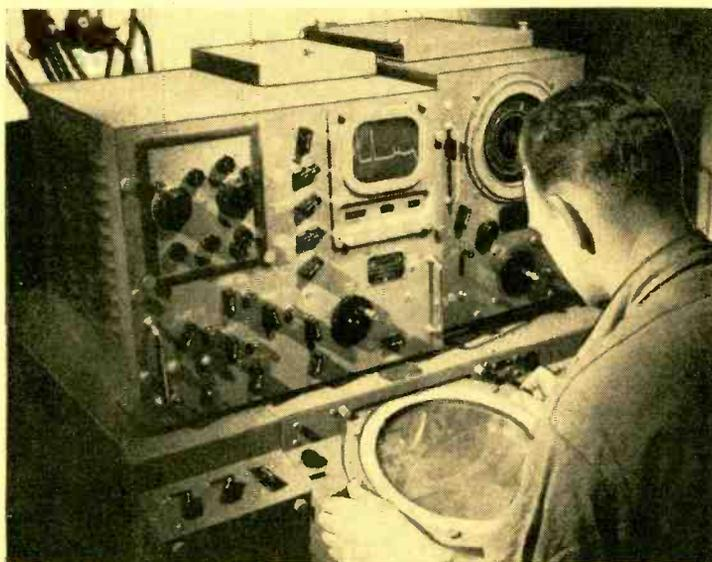
Seated at a console, the radar operator relays target data by telephone so that the rest of the fleet may be kept informed. The small square scope at top of console is called an A Scope, and the large round cathode-ray tube he is peering into is a PPI—Plan Position Indicator.
