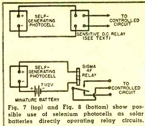
Fig. 7 (top) and Fig. 8 (bottom) show possible use of selenium photocells as solar batteries directly operating relay circuits.
