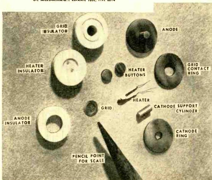
At the upper left, a G.E. technician examines the parts of the 6BY4 micro-miniature tube through the use of a shadowgraph. This optical comparator brings the parts up to a size reasonable to the naked eye. The diagram at the center is a cross-section view of the 6BY4. Individual pieces of a ceramic 6BY4 are shown in the bottom view. The extreme simplicity in constructing such tubes is obvious from this latter view.
