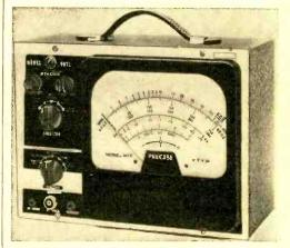
N.Y., the instrument is available as a kit for \$35.95, or factory-wired at \$49.95. The 7½" meter has readings for ohms, d.c. volts, a.c. volts, decibels, and a special scale for 5 volts a.c. only.
