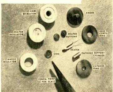
At the upper left, a G.E. technician examines the parts of the 6BY4 microminiature tube through the use of a shadowgraph. This optical comparator brings the parts up to a size reasonable to the naked eye. The diagram at the center is a cross-section view of the 6BY4. Individual pieces of a ceramic 6BY4 are shown in the bottom view. The extreme simplicity in constructing such tubes is obvious from this latter view.
