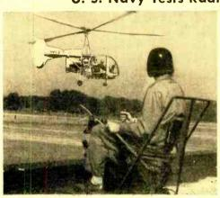
A REMOTE CONTROL HELICOPTER, the world's first successful model of this type, has been developed by the *Kaman Aircraft Corporation*. Designed for the U. S. Navy, the modified *Kaman* HTK-1 has been flying for more than a year and has over one hundred hours of R/C operation.
