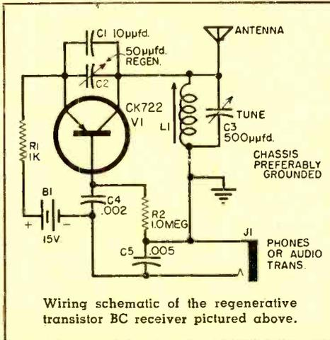
with the Vari-Loopstick. This will not completely cover the broadcast band and some experimenters may want to add a trimmer across both the coil and capacitor.
