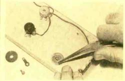
and its mounting screw by mica or plastic. The lug next to the washer is a "hot" connection; the chassis forms the other electrode.
