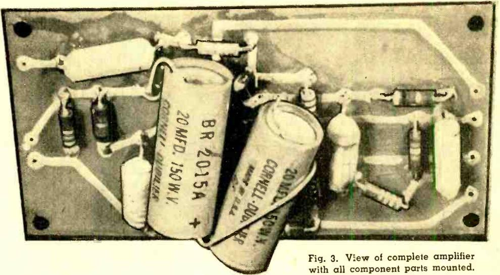
Fig. 3. View of complete amplifier with all component parts mounted.
