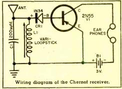
with the Vari-Loopstick. This will not completely cover the broadcast band and some experimenters may want to add a trimmer across both the coil and capacitor.
