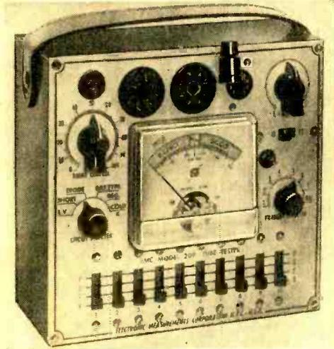
all tube base types commonly found in home sets. Accurate checks can be made for tube quality, shorts, leakages, continuity, and opens between tube elements. Featured is a meter with a 3½" scale printed in three colors.
