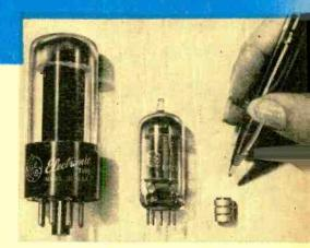
At top of page, James E. Beggs of the General Electric Research Laboratory holds a miniature ceramic vacuum tube designed by him and a group of his associates following extensive research. The photograph below shows various milestones in radio and television receiving tube development: at left is a conventional glass type with a plastic base, in the center is a miniature-type tube, and at right is the ceramic micro-miniature tube.
