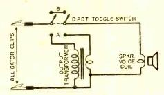
sets, the connection will have to be made directly to the voice coil; for others, an output transformer will be needed.
