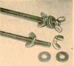
Detail view (above) of the mounting for one of the "Handy Clamps," which are manufactured by Stanley and are available from most hard ware stares. To compensate for varying chassis weights, the clamps may be moved along the rocker bar to new pre-drilled positions.
