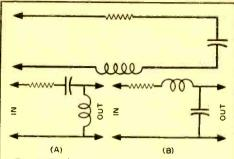
Fig. 6. (Top) Basic form of a series resonant circuit. Fig. 7. (Bottom) Part (A) is an arrangement for low-frequency roll-off and part (B) is a circuit to provide high-frequency roll-off as seen below.
