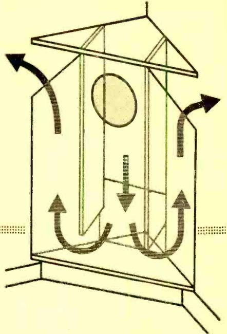
Phantom view of the enclosure shows sound paths from rear of the speaker.
