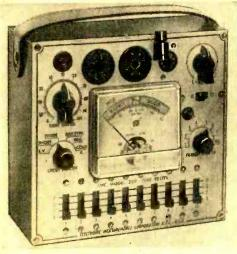
all tube base types commonly found in home sets. Accurate checks can be made for tube quality, shorts, leakages, continuity, and opens between tube elements. Featured is a meter with a 31/2" scale printed in three colors.
