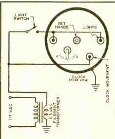
Fig. 2. Simplified schematic which shows operation of the clock from a filament transformer. Most 6-volt clocks can be directly attached to a.c. filament winding.
