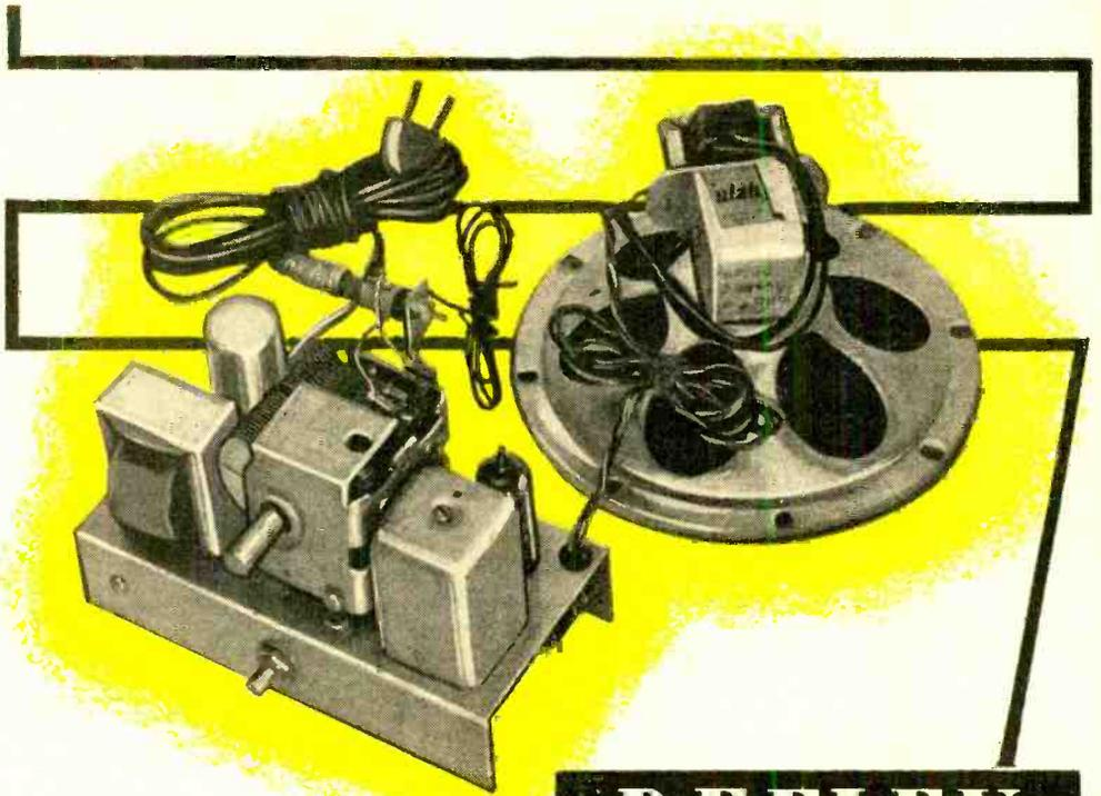
**E**CONOMY of operation is featured in this little radio receiver. As it consumes about the same amount of power as an electric clock, continuous operation is practical. Maintenance cost should be negligible, for it has only one tube to wear out and the balance of the parts are operated at such a small fraction of their ratings that they should never require replacement.
