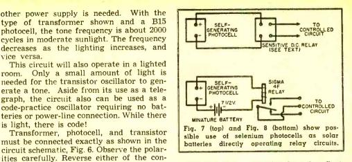
Figure 7 uses a sensitive d.c. relay. Such relays as the Weston "Sensitrol" and Barber-Colman "Micropositioner" can be obtained to close on currents of a few microamperes. They will operate easily from the photocell, even with small amounts of light.
