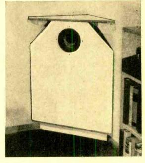
Only the labyninth remained as the baffle which was least critical and, because of less internal sound pressure, also adaptable to cheap building material. This one sits unobtrusively back in a corner, a position which fortuitously improves the bass response.
