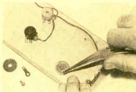
and its mounting screw by mica or plastic. The lug next to the washer is a "hot" connection; the chassis forms the other electrode.
