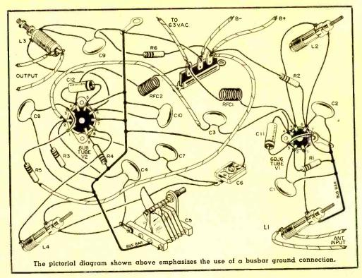
mc., and L3 to 4000 kc. Apply voltage to the tuner and check with the grid dip oscillator to see that the oscillator circuit is oscillating at 45 mc. Final tuning can be completed on received signals.
