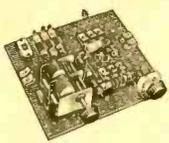
This regenerative two Transistor Radio has given more than ample earphone volume on broadcast stations located several hundred miles away. When used with 60 ft. outside antenna well beyond 1000 miles have been repeatedly heard. Kit comes complete with two transistors, Argonne transistor audio transformers, condensers, resistors, masonite board, etc.; schematic diagram plus 115 page book, showing more than 50 practical transistor circuits and "How-to-do-it-Instructions".
