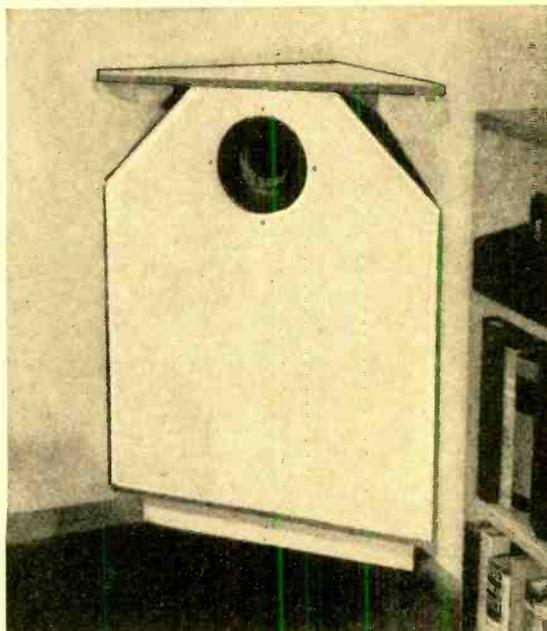
**T**HIS SPEAKER BAFFLE (it can hardly be called a cabinet) is admirably suited as a temporary or extra installation because of its low cost and ease of construction. The six functional parts can be cut and fitted together in about an hour. It doesn't require a finished cabinet maker either, the design is not critical, and the material allows for some tolerances in measurements. In fact, anyone who can recognize a saw and a hammer should have no trouble with the carpentry.
