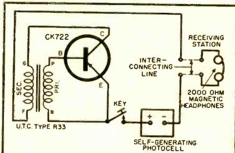
Fig. 6. Transistors enable solar batteries to be used where the voltage demands are very small. This circuit is that of the audio tone generator which is pictured on page 66. Experimenters can also use it as a code practice oscillator. Frequency of tone from the oscillator will vary according to the amount of light on self-generating photocell.
