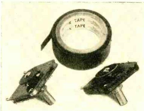
rators. To prevent this, seal the four open sides. The capacitor at the left is shown as it came from the factory. The capacitor at the right was sealed on all four sides with a 1/2"-wide strip of Mystik tape. Any type of pressure tape could have been used instead.
