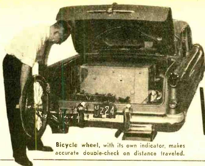
Bicycle wheel, with its own indicator, makes accurate double-check on distance traveled.
