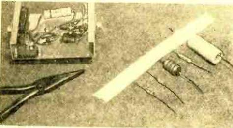
available at most hardware stores. This tape will adhere to virtually any surface but does not make a permanent bond. Nor will it leave a sticky residue on either the workbench surface or parts themselves.
