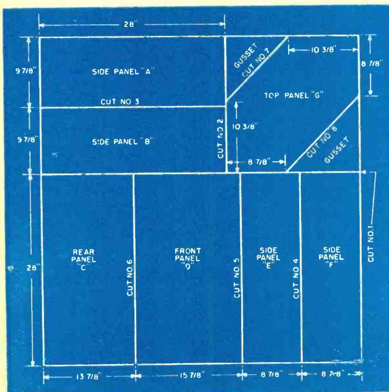
**How to lay out a sheet of 4' x 4' plywood to provide all the panels needed for building the enclosure. For best results, follow numbered cutting instructions. Dimensions shown are correct and allow for cutting waste resulting from saw's groove. Plywood's good surface should face up during all cutting operations. Your best bet is to have cuts made at lumber yard. If you cut the wood yourself, the best single tool is a crosscut handsaw.**
