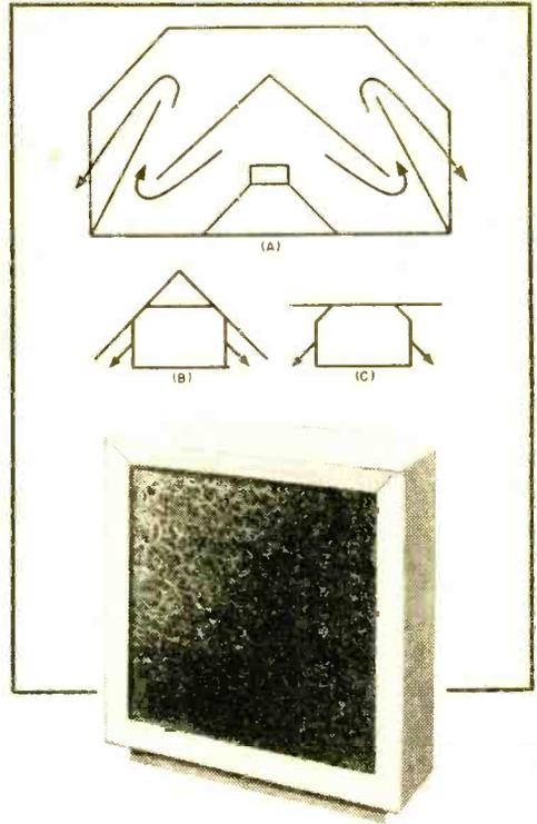
**Sound path** in Stephens enclosure (above) is shown by arrows. Horn is formed by the cabinet's internal paneling which permits placement against wall if corner is not handy. Below, Cabinart's Model KR-3, which depends on corner placement for proper horn loading. Sound path provided by KR-3's structure is somewhat shorter, needs room walls. In both types, highs radiate from front of speaker, bass from rear via the path of the folded horn.
