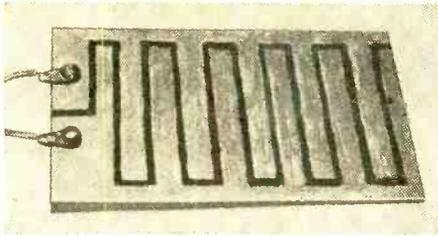
Rain "sensor" can be made by etching copper-clad plastic as above, or by painting or cementing conductive strips on a non-conductor.
