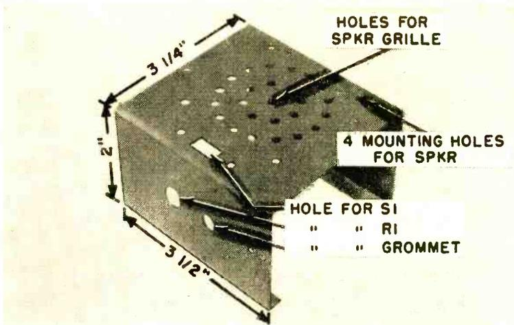
Enclosure is cut down from standard aluminum chassis. Exact hole sizes and spacings must be determined from the specific components which you use in building this unit.
