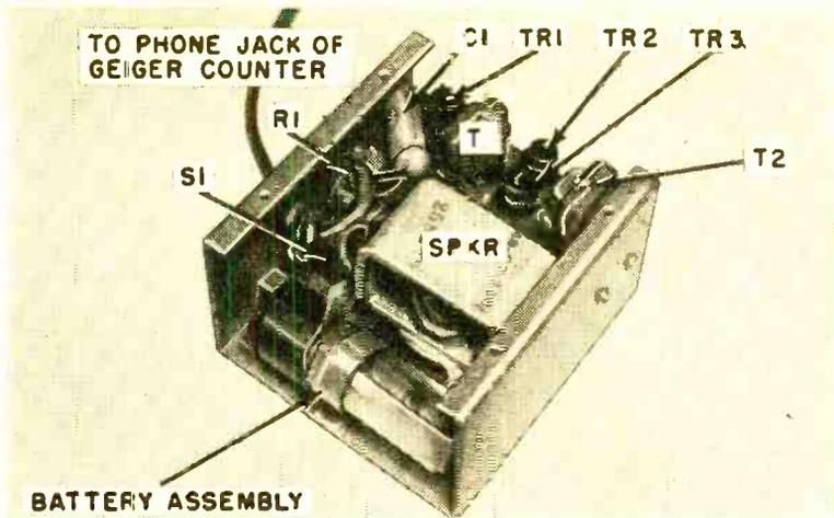
Although assembly is very compact, all components can be easily mounted with a little care. A larger chassis would simplify wiring without affecting performance adversely.
