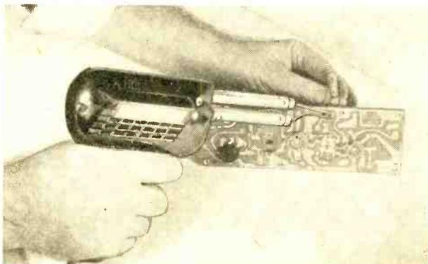
**Joining wires**, or making connections to tie lugs, pigtail leads or terminal strips, is accomplished efficiently with a 100-watt gun. Instant-heating feature of electric gun is useful for work on printed circuits.
