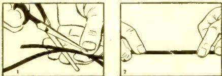
overlap the two ends of the recording tape and cut them at a 60° angle. FIG. 1. Then bring the ends together so that they just touch. Align them with their uncoated sides up. FIG. 2. (The uncoated side of plastic tape is always the shiny surface).
