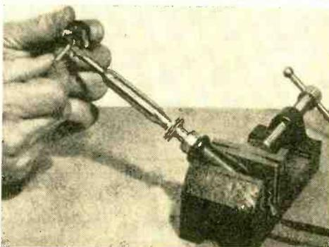
photo. Clamp the iron in a bench vise. This frees both hands for holding parts and applying flux and solder. Parts should be
