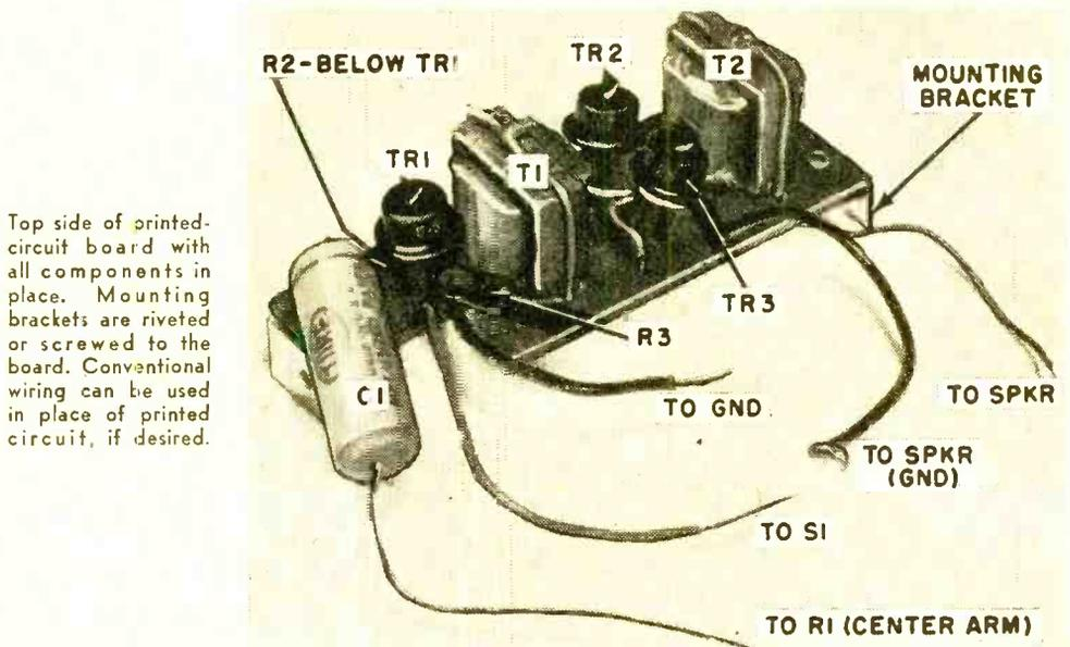
Top side of printed-circuit board with all components in place. Mounting brackets are riveted or screwed to the board. Conventional wiring can be used in place of printed circuit, if desired.
