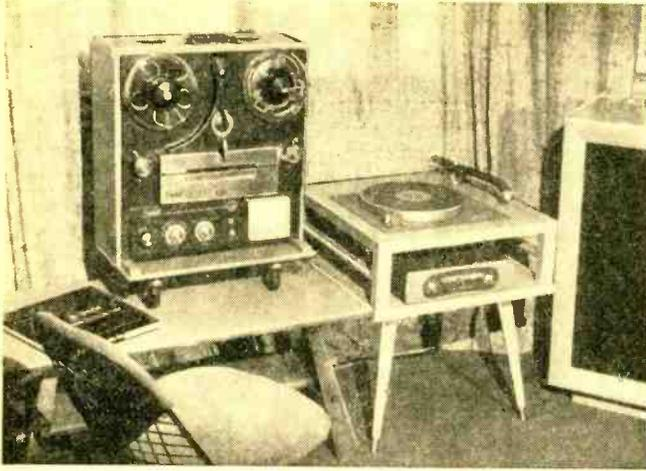
Berlant "Broadcast Recorder" is one of many top-quality tape machines requiring an external amplifier and speaker for playback.
