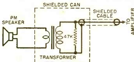
ed leads. For better frequency response, load the high impedance winding of the transformer with the 47,000-ohm resistor, as shown.
