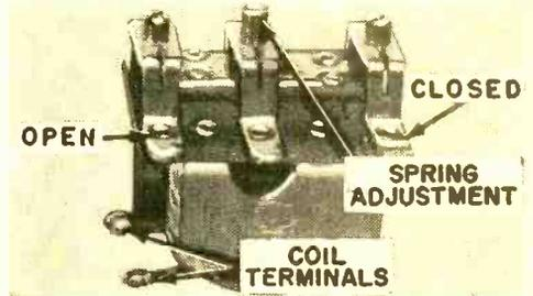
**Screw adjustments** vary the relay's sensitivity. Center screw alters spring tension; outer ones change gaps on "open" and "closed" contacts.
