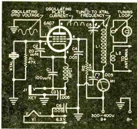
Fig. 1. Diagram of a typical, crystal-controlled oscillator. With power supply and antenna, this oscillator forms a practical, low-power c.w. transmitter, operation of which is discussed in the text.
