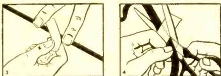
**For Best Results** join the ends of your magnetic tape with a good quality splicing tape. "Scotch" Brand Splicing Tape No. 41 is specially made to give a tight, noise-free joint. Apply it diagonally, covering the ends of the magnetic tape. FIG. 3. Then, trim off the excess Splicing Tape, cutting into the recording tape slightly. FIG. 4. Detailed and illustrated splicing instructions come with every box of "Scotch" No. 41 Tape.
