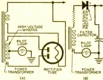
shown in the diagram (A), will act as both a pilot light and a fuse. The lamp should have a current rating approximating the amount of current drawn from the supply. For instance, a 60-milliampere lamp may be used if a current of 50 to 60 milliamperes is being drawn.
