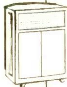
**THE CENTURION KIT.** Four-way system folded-horn, corner enclosure. Uses exclusive E-V "W" type single-path indirect radiator for propagation of extended bass. Sealed cavity behind 15 in. low-frequency driver cone promotes superlative transient response, subdues cone excursions, lowers distortion. For use with E-V Model 105 or Model 117 package of driver components. Finished size: 42½ in. high, 29 in. wide, 22½ in. deep. Shpg. wt. 75 lb.
