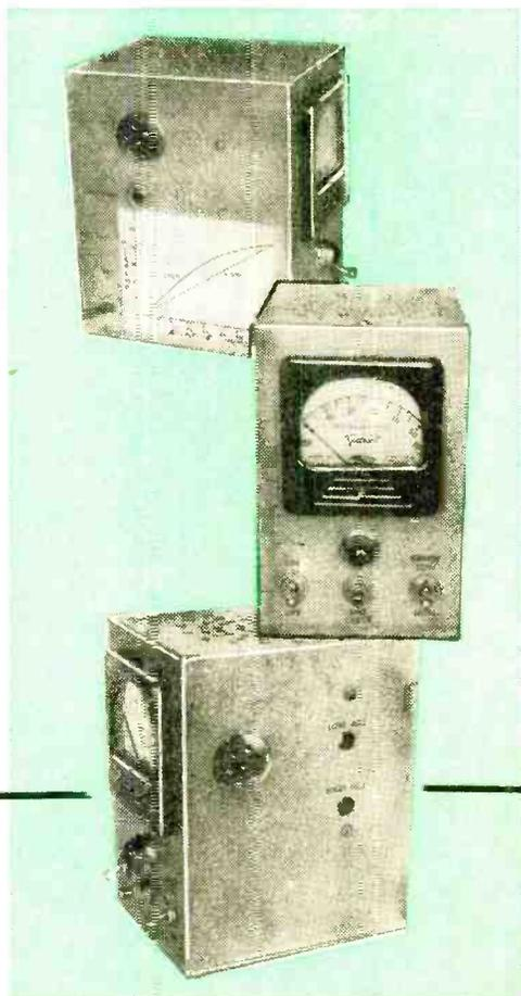
Three separate views of the author's model. The sensing element is inside the metal case and provision has been made to plug in a second element for external use. Note the vent plugs on both sides of the case, and the many small holes drilled in the top and bottom of the housing which are essential for quick and reliable action.
