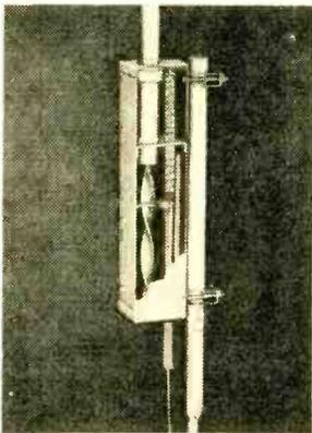
A slotted crossarm within the housing is moved downward by an easy pull on the manually operated steel cable with a direction indicator which may be mounted inside the house, outside, or on a porch. As the arm moves down, the antenna is rotated clockwise through 360°. The design of the
