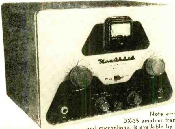
Note attractive appearance of assembled Heathkit DX-35 amateur transmitter. The complete kit, less crystals, key and microphone, is available by mail from the Heath Company for \$56.95.
