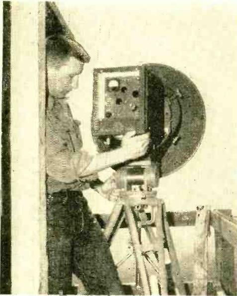
**Portable antennas** like the one at left can be easily and quickly set up in different mountain locations for fire spotting.
