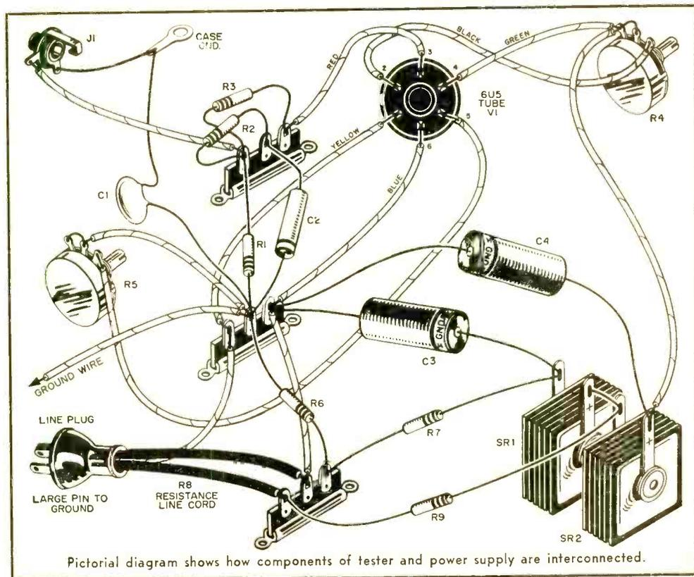
Pictorial diagram shows how components of tester and power supply are interconnected.
