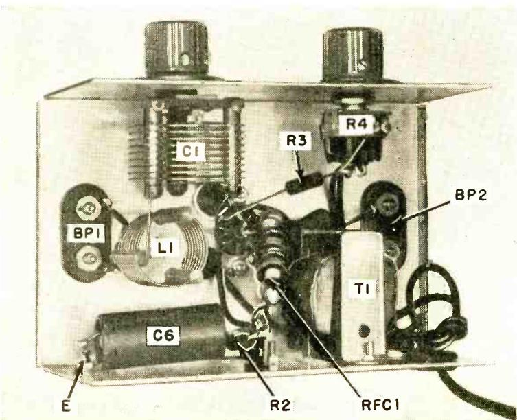
Major parts of the "Lucky 15" are identified in under-chassis photo at left. For ease in assembly, the components should be mounted in the order specified in the text.
