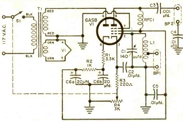
**Fig. 2.** Schematic diagram of the "Lucky 15." A single 6AS8 multi-purpose tube serves as both r.f. amplifier and power supply rectifier in this unit, which will provide substantial gain over the 12-mc. to 33-mc. frequency range. See parts list below.
