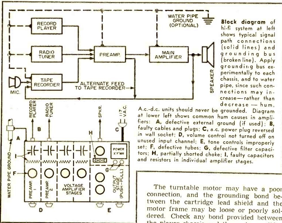
**Block diagram of hi-fi system at left shows typical signal path connections (solid lines) and grounding bus (broken line). Apply grounding bus experimentally to each chassis, and to water pipe, since such connections may increase—rather than decrease—hum.**
