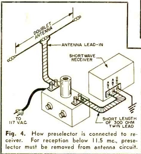
**Fig. 4.** How preselector is connected to receiver. For reception below 11.5 mc., preselector must be removed from antenna circuit.
