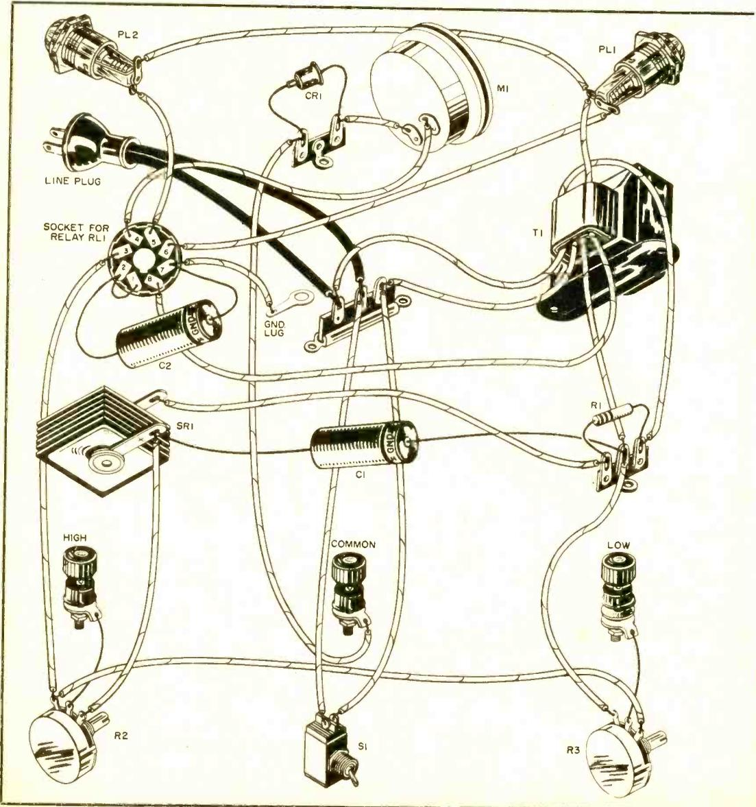
are connected between *low* (+) and *common* (-), those from 22½ volts to 90 volts between *high* (+) and *common* (-). You should be able to run the current from a small value to 5 milliamperes or more.
