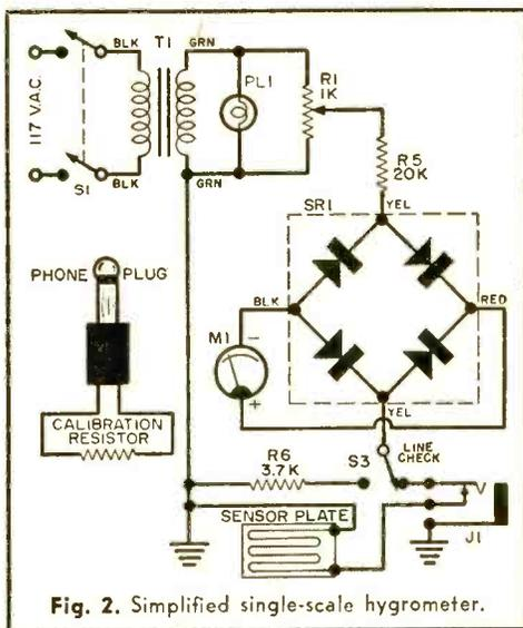
Fig. 2. Simplified single-scale hygrometer.
