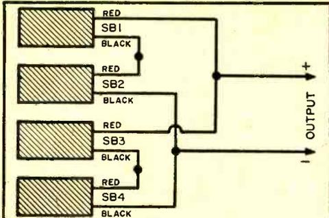
**Fig. 1.** Four-cell battery with series-parallel connection. The two upper cells are connected in series to form one string, and the two lower cells form a second string. The two strings are connected in parallel. Lead color-coding shown applies to B2M selenium cells.
