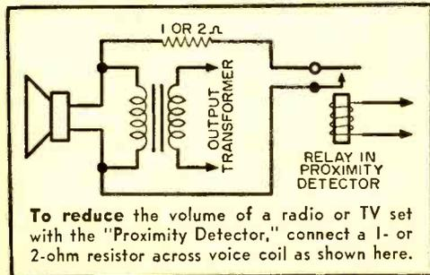
To reduce the volume of a radio or TV set with the "Proximity Detector," connect a 1- or 2-ohm resistor across voice coil as shown here.
