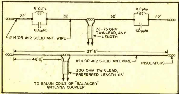
Two popular types of "all-band" amateur antennas for the 80- to 10-meter bands which are discussed in the text. At top is a "multimatch" antenna, while below it is one version of the Windom antenna.
