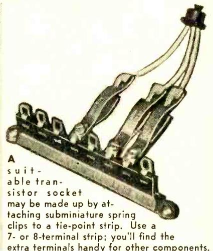
**A** suitable transistor socket may be made up by attaching subminiature spring clips to a tie-point strip. Use a 7- or 8-terminal strip; you'll find the extra terminals handy for other components.
