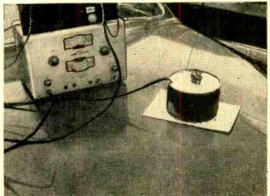
**To locate** a rattle on the outside of your car, place the speaker in the general vicinity of the rattle. A sheet of paper under the can (above) prevents speaker itself from rattling and protects the finish.
