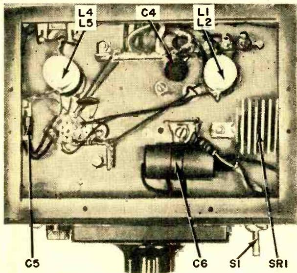
Below-chassis view of unit (at left) shows placement of coils on opposite sides of chassis. Adequate isolation must be maintained between coils L1/L2 and L4/L5. The "RF Tune" control is located at the left of the main tuning dial; when you adjust the dial, this control must be adjusted simultaneously.
