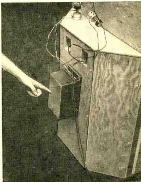
**The Sherwood SFX35** shown here is being used experimentally with a Heathkit 3-way speaker system. The crossover frequencies are 300 and 5000 cycles, separating the three speakers in the system.
