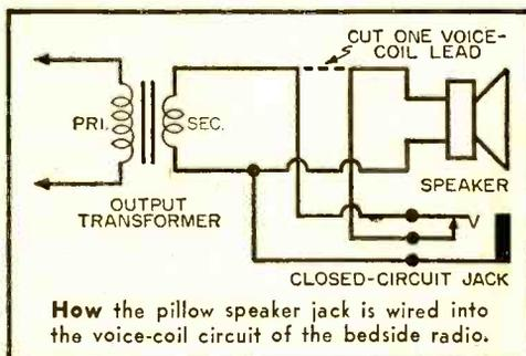
How the pillow speaker jack is wired into the voice-coil circuit of the bedside radio.
