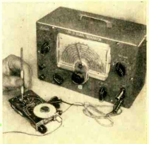
To align the superhet, you'll need a signal generator and an insulated alignment tool.
