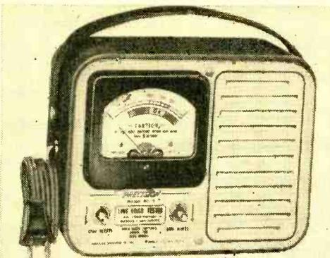
power lines to handle loads imposed by a wide range of electrical appliances, such as air conditioners, broilers, etc. It has a wide-vision meter with a scaleplate in three colors. Line-load conditions are indicated directly as "LOW," "OK," or "HIGH."
