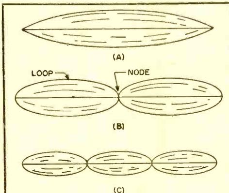
**Fig. 2.** Analogy showing relation of overtones to fundamental: (A) a string producing its fundamental tone by vibrating in one part; (B) first overtone or second harmonic of the string; (C) second overtone or third harmonic.
