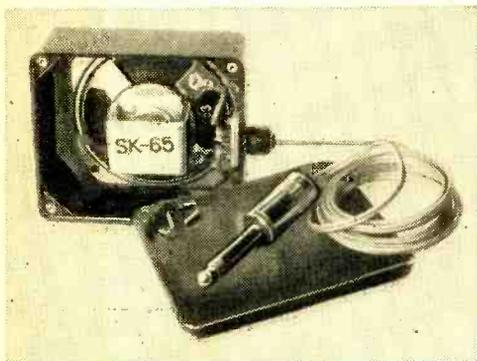
speaker to be plugged into a closed-circuit jack installed on the radio. (Mount the jack on the radio cabinet or back panel, making sure that it is insulated from the radio's chassis.) The jack is wired into the voice-coil circuit in a manner that mutes the radio's speaker when you plug in the pillow speaker.
