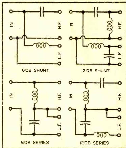
**Crossovers** consist simply of a coil and a capacitor wired in shunt or series as shown. By using two coils and two capacitors, the attenuation rate is increased from 6 to 12 db, four times less power.
