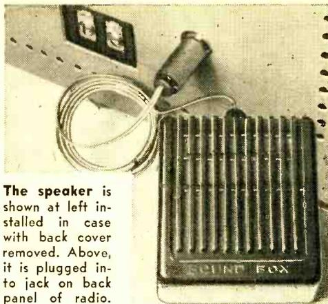
The speaker is shown at left installed in case with back cover removed. Above, it is plugged into jack on back panel of radio.
