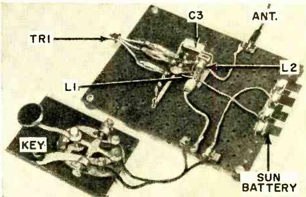
through *R1*. The "load" is connected in parallel with the primary winding of *T1*; because of its relatively high impedance, the earphone has a negligible effect on circuit operation. The common-emitter circuit configuration is used.
