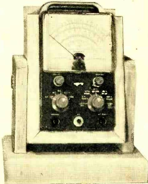
the top-back of the handle holds the meter in place and still permits it to be removed with ease.
