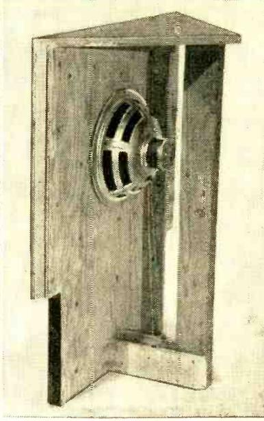
"Sandwich" (far left) is formed by bonding sheet of Celotex between two plywood panels. Photo directly at left shows how top piece, back brace, and speaker are fitted to complete the baffle.
