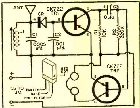
"Shirt-Pocket" transistorized receiver built by POP'tronics reader Elton V. Stolberg. Schematic diagram appears above; below is a view of the receiver removed from its case. You'll find the construction details on the following page.
