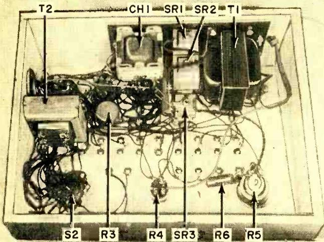
**Bottom** view of the tube tester (at left) indicates placement of major parts. Filament supply is at far left. The plate and grid voltage supply, shown at the top of the photo, is constructed on a separate chassis—in this case a piece of 8" x 3 1/2" scrap aluminum.
