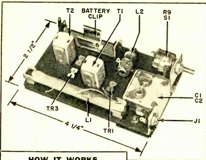
**Top view** of the receiver chassis shows location of all major components. The transistors are not in their respective sockets. Screw adjustments of C1b and C2b are visible on the top of C1/C2. Antenna coil L1 is held in place with a pair of fuse clips.
