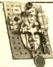
For those interested in mastering the international code, an audio tone oscillator is essential. The circuit of this transistorized feedback oscillator has the simplicity of the neon glow, the signal strength of the vacuum tube, and requires only two penlite cells for weeks of service. It may be used for solo practice, or two may send and receive with the same unit. Kit comes complete with Transistor, Telegraph Key, Resistors, Condensers, Masonite Board, etc., and Schematic Diagram.
