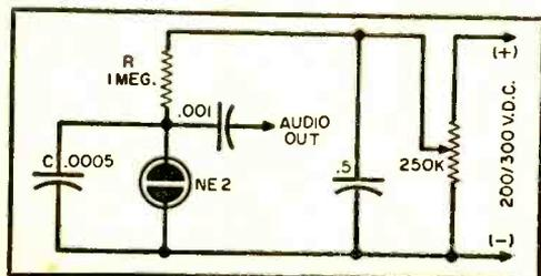
shown in the diagram will work to approximately 3000 cycles before oscillation ceases. At this "drop-out" point, the NE-2 will glow brightly, indicating that it is completely ionized.
