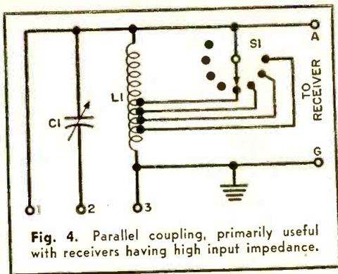
Fig. 4. Parallel coupling, primarily useful with receivers having high input impedance.
