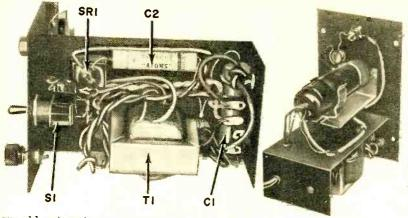
Major parts are identified in the under-chassis view at far left. Use of full length transformer leads gives chassis a somewhat crowded appearance but makes for better soldering. Top view directly at left shows overall placement of the various parts.
