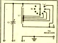
Fig. 3. Series coupling between "Peaker" and receiver. Extra tap on switch, marked "X", may be added to short out coil LI entirely.
