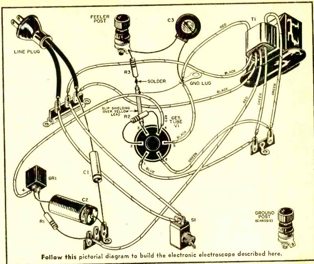
cord into a suitable 117-volt a.c. receptacle and trip the toggle switch to the "ON" position. After a 15-second warm-up, the face of the tuning eye should exhibit its characteristic green glow with a shadow angle of about 25°. The edges of the shadow should be quite sharp and clear. If they are fuzzy or if the angle is smaller than 25°, reverse the line plug. This will clear up the trouble.
