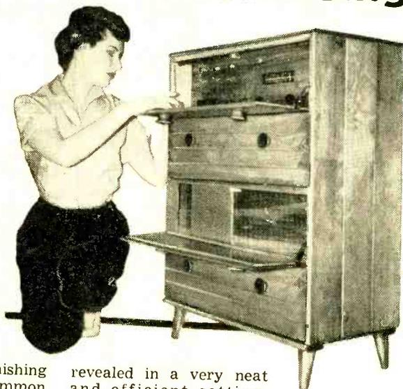
**Y**OU CAN GIVE your hi-fi gear a home—without mortgaging your own, or letting the chassis and wires drive you right out of it. As illustrated in the photos, an unpainted chest—priced at \$15.75—can be harnessed to serve as an equipment console. All it takes is a little additional hardware, some finishing materials, and basic skills with common hand tools.
