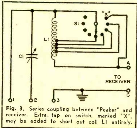
Fig. 3. Series coupling between "Peaker" and receiver. Extra tap on switch, marked "X", may be added to short out coil L1 entirely.
