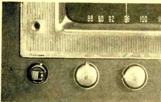
**Dual** concentric knobs at far left symbolize newly installed loudness control. White dots on knobs help recall positions.
