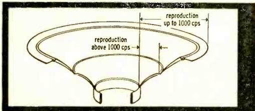
This compliance serves as a mechanical cross-over providing the single voice-coil with the area of the entire cone for propagation of the lower frequencies and reducing this area and mass for the more efficient reproduction of the higher ranges above 1000 cps. Proper phasing between the two cone sections is assured by the controlled mechanical resistance provided by the viscous damping applied to the compliance.
