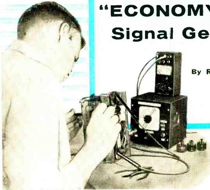
Testing a radio is an easy job with this versatile signal generator. Using only one tube, and plug-in coil construction to keep the cost down, it will cover the 375-kc. to 65-mc. frequency range.
