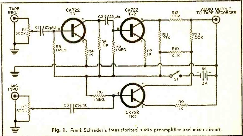
Fig. 1. Frank Schrader's transistorized audio preamplifier and mixer circuit.
