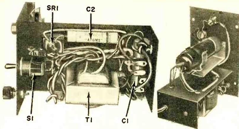
Major parts are identified in the under-chassis view at far left. Use of full length transformer leads gives chassis a somewhat crowded appearance but makes for better soldering. Top view directly at left shows overall placement of the various parts.
