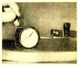
Checking stylus pressure, the Scherr precision gage indicates exact readings on clearly legible dial. An extra hand marks the maximum weight and keeps its position on the dial after the measurement is completed. An automatic record of the stylus pressure is thus retained.
