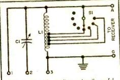
Fig. 4. Parallel coupling, primarily useful with receivers having high input impedance.
