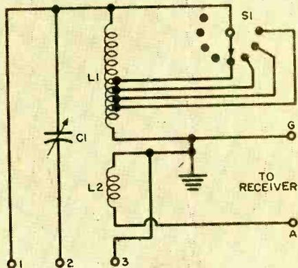
Fig. 1. Circuit of the "Peaker," which uses link coupling. Parts values are given below.
