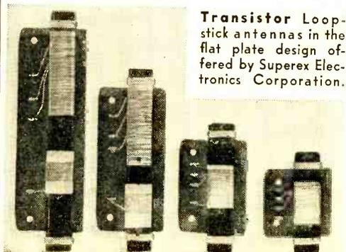
**Transistor Loopstick antennas in the flat plate design offered by Superex Electronics Corporation.**
