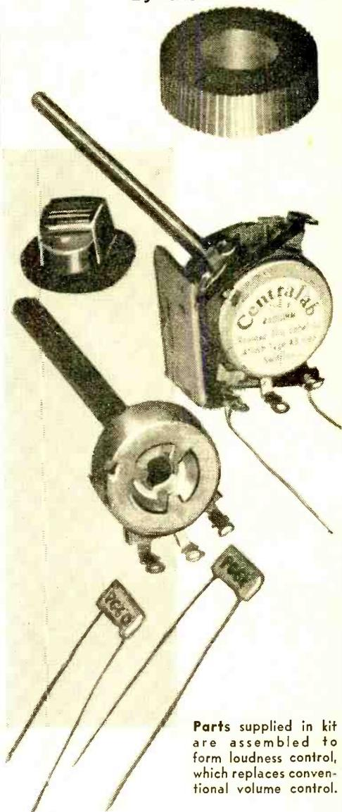
Parts supplied in kit are assembled to form loudness control, which replaces conventional volume control.
