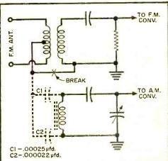
Schematic diagram of antenna input circuit most commonly used in AM-FM tuners. Dotted lines indicate changes around C1 and C2.
