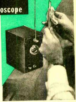
Rubbing an insulator with soft cloth and bringing it near the feeler antenna of the electroscope will close its "eye." This unit can take a 100,000-volt discharge safely. The chassis is welded to front panel of case, shown below.
