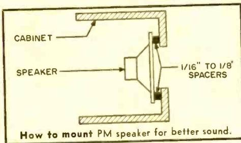
Eliminate this objectionable condition by locating the speaker slightly behind the front panel of the cabinet to provide a small air space between the panel and the speaker.
