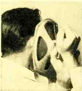
This sharp blow will set the cone vibrating at its natural resonant frequency, and the voice coil will vibrate in the air-gap at the same time. If the voice coil has free movement in the air-gap, you will hear a clear *boing* with no muffling and rattles. If the voice coil and cone sound free but you hear some rattling anyway, chances are that it is coming from some other spot.
