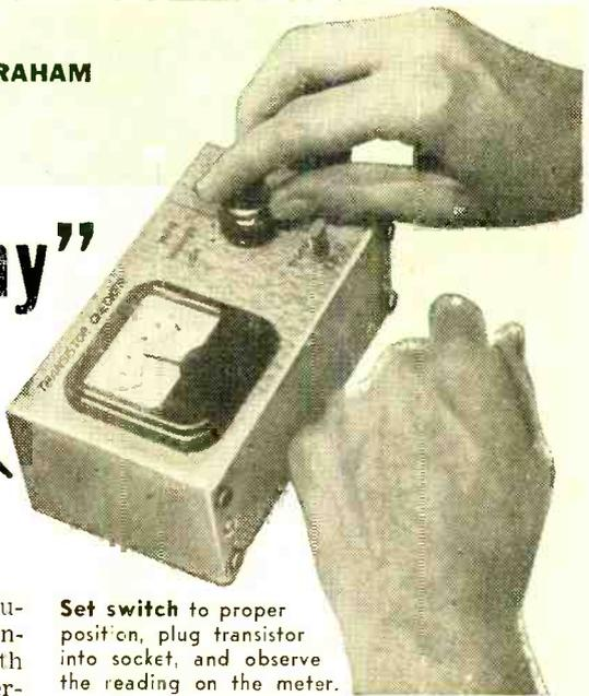
IT DOESN'T TAKE LONG to accumulate a small but varied stock of transistors once you start experimenting with these little gems. Fortunately, to determine whether a transistor is good or bad requires a tester of extreme simplicity. The "Economy" Transistor Checker performs two sensitive tests which will quickly tell you if a transistor has been damaged due to overload or contamination of the germanium, whether the transistor is shorted or open-circuited, or if it is just excessively leaky.\*
