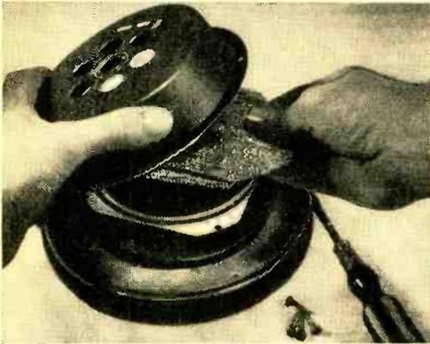
with a chassis punch—to form an attractive pattern of holes. Coat the inside and outside of the plate with an air-dry wrinkle varnish. Back the perforations with several thicknesses of bronze window screening. The mounting board may be simply a piece of wood to which the pie plate is screwed, or, preferably, it can be a disc of wood turned on a lathe to accept the lip of the pie plate.
