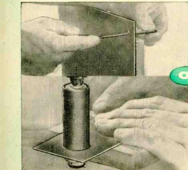
**Rat-tail files** are a good substitute for a reamer on small-diameter holes. Half-round files are used for larger holes. Be careful to keep hole as round as possible. Cut on forward stroke of file only. . . .
