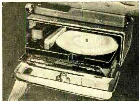
"Highway Hi-Fi" was Chrysler's slogan for 16-rpm phonographs fitted under the dashboard. Actually, the "fi" was no higher than that of the car radio through which the music was reproduced.
