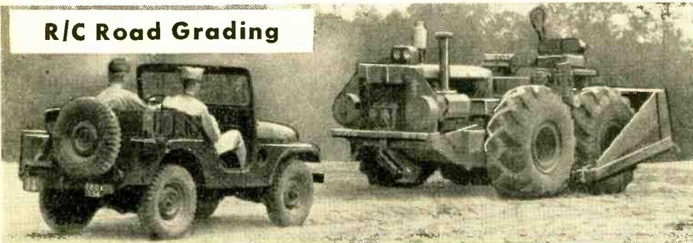
**Push-button construction work** is on the way. A standard U.S. Army "Touredozer" equipped with standard military radio equipment (above) can be put through its paces by helicopter or jeep with transmitter and special control box up to a distance of 15 miles. It's under test at Fort Belvoir, Va.
