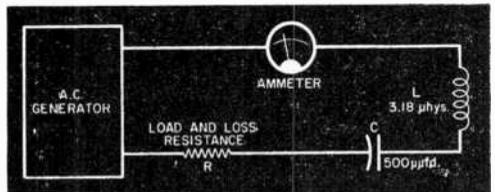
Fig. 1. Series resonant circuit.
