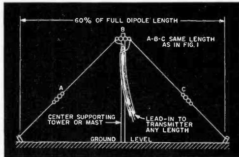
**Fig. 2.** Only one supporting mast is needed with this antenna.
