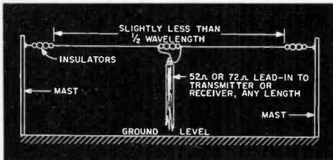
**Fig. 1.** "Old Faithful" dipole is large for the 80-meter band.
