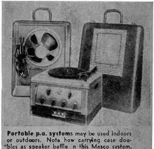
**Portable p.a. systems** may be used indoors or outdoors. Note how carrying case doubles as speaker baffle in this Masco system.
