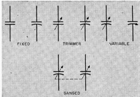
lead to the ground side of circuits—but don't confuse this with the polarity marking of an electrolytic capacitor.
