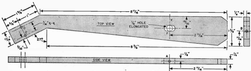
Template and construction details of the home-made arm are given above. A choice of material is available for the body of the pickup arm. The lettered points in the diagram refer to specific construction details which are covered in the text.
