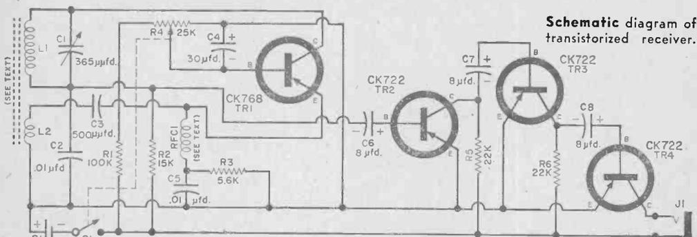
Schematic diagram of transistorized receiver.
