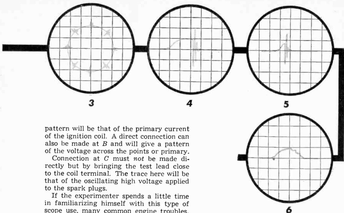
pattern will be that of the primary current of the ignition coil. A direct connection can also be made at *B* and will give a pattern of the voltage across the points or primary.
