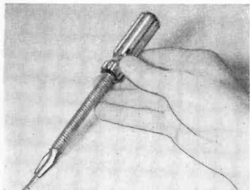
tend the solder to the contact where it's needed. Solder carried this way in a tool kit will conserve valuable space, as well as keep it from getting lost. —J.A.C.
