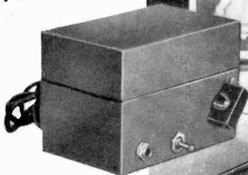
Completed transmitter mounted in file case. Note horizontal mounting of its single tube.
