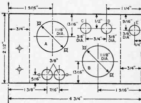
**Fig. 1. Chassis template, top view.** See text for explanation of details.
