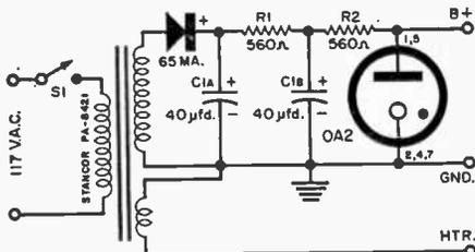
Fig. 3. Power supply for use with audio oscillator. Any supply delivering about 100 volts will do.
