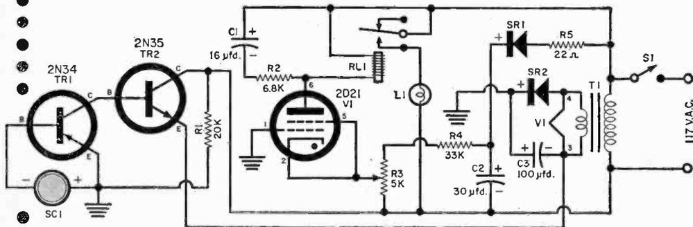
Pictorial and schematic diagrams of the light target. Several different makes of relays will operate properly. A 1N48 or equivalent diode may be substituted for the selenium rectifier (SR2) which is used as the low-current power supply for the two transistors.
