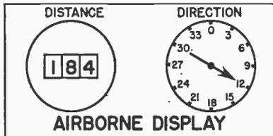
CAA. He next tunes in the frequency of the selected station by means of a dial, and checks the coded or voice call of the station with that given on the chart. The magnetic bearing of the station from the aircraft is set into the system by means of a selector wheel; the bearing of the station is thereafter retained at all times until changed to a new station.
