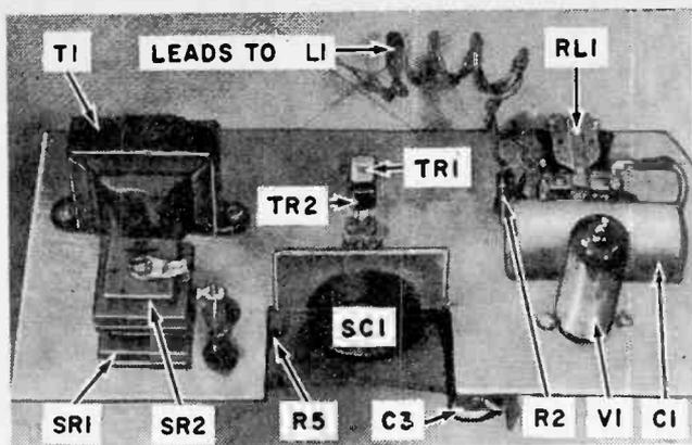
Top and bottom views of the chassis of the photocell unit at left show the uncrowded parts placement. The solar cell (SCI) may have screw mounting terminals or pigtail leads; characteristics of both of these types are similar.
