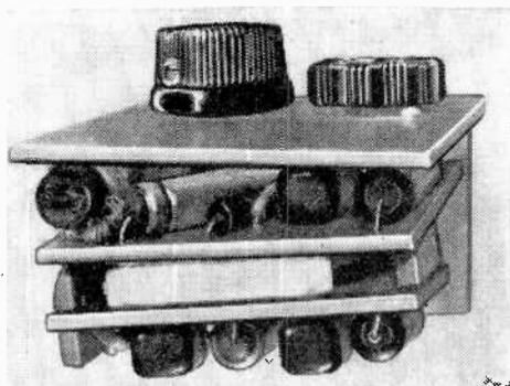
Side view of the completed assembly. Note the small wooden spacers glued between the two printed-circuit chassis boards. The three sides and the bottom of the chassis are installed later.
