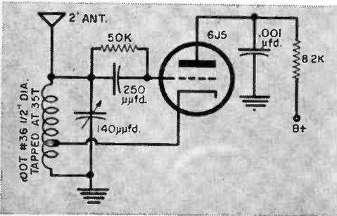
be made that uses a radio receiver having a beat-frequency oscillator (BFO). You will also need a simple r.f. oscillator (as shown in the diagram) whose output signal can be tuned in on the receiver. About 100 volts is okay for B+.
