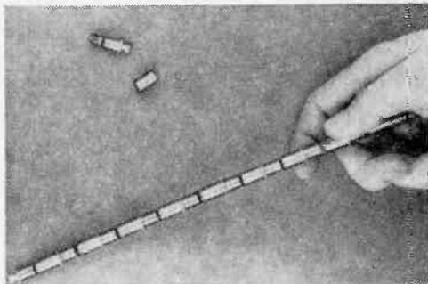
inverse rating of 4000 volts. For higher ratings, additional rectifiers can be connected. Threaded units with current ratings up to 5 amperes are also available and can be similarly assembled. (Audio Devices, Inc., 620 E. Dyer Rd., Santa Ana, Calif.)
