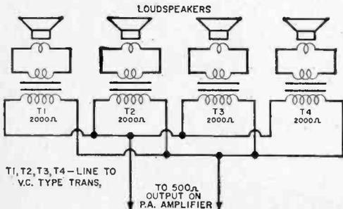
**Line-matching transformers** are necessary in some multiple speaker setups. This diagram shows such a hookup.
