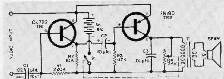
**Two-transistor audio amplifier** submitted by reader Albert Brooks is assembled on plastic base.
