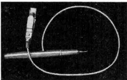
that will show the frequency of discharge at spark plug points and also the comparative strength of the fire—without removing the shield which is over the plugs. It consists of a NE-2 neon bulb, one 2-megohm,
