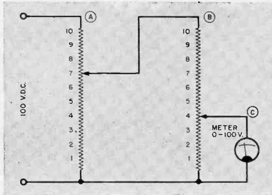
Fig. 1. Circuit showing connection of two standard potentiometers and a sensitive meter for basic arithmetical calculations. See page 118 for details of technique.
