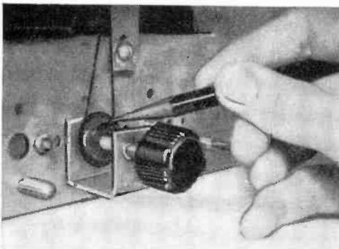
used where a power cord passes through a metal chassis. Slip a tight-fitting grommet over the tuning shaft and restraining the dial cord. If faster tuning is desired, cement a larger grommet over a smaller one as shown. It may be necessary to use a touch of Duco cement to fix the grommet to the shaft. —J.A.C.
