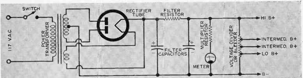
Basic power supply circuit, showing typical uses for components discussed in Part 1 and Part 2.
