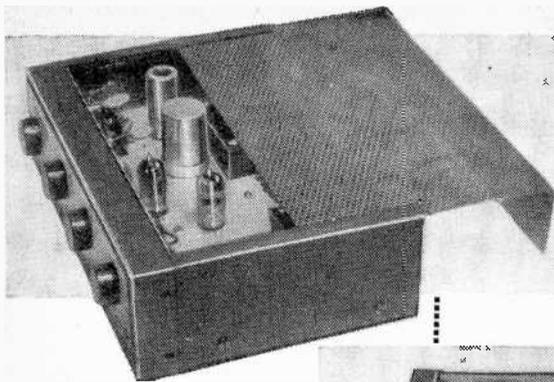
Note how perforated cover slides out (above) to allow for tube checking. At right is the completely wired amplifier chassis as it appears from the underside. Pictorials help in making point-to-point connections as well as placement of components to eliminate the introduction of hum and spurious couplings.
