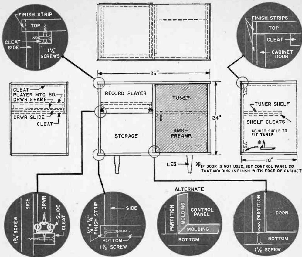
Construction details above should be followed faithfully to obtain best results on the finished cabinet. Note the alternate detail shown for the use of a fixed control panel rather than a door; instructions are given in text for fitting either one. Also, bottom piece is butted inside the side pieces—finishing strips make it appear otherwise.
