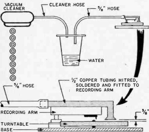
You can build this chip remover easily from a vacuum cleaner, inexpensive hose and copper tubing (details on p. 105).
