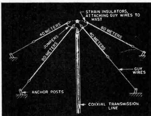
quency. This means that a dipole cut to 3.7 mc. is again resonant and capable of good operation at 11.1 mc., and the 7.15-mc. dipole is resonant at the third-harmonic frequency of 21.45 mc. This is very close to the Novice 21-mc. amateur band. If the 40-meter dipole is cut a bit shorter than optimum, the third-harmonic resonant frequency will fall within the 15-meter (21-mc.) Novice band.
