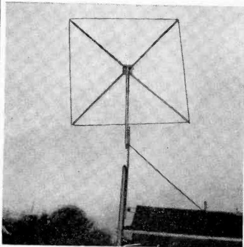
results were amazing. During the first couple of nights I logged all the continents. I used 300-ohm twin lead for my lead-in instead of the 52-ohm coaxial line. Enclosed is a photograph of the antenna.
