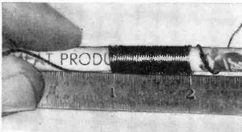
indentations on a wooden pencil exactly 1" apart. Wind a single layer of the wire in question between the two marks, count the number of turns, then refer to the lineal turns per inch column of the copper wire table found in every radio or electrical handbook. For the smaller sizes, a  $\frac{1}{2}$ " layer will give just as accurate results in less time. —R. B. K.
