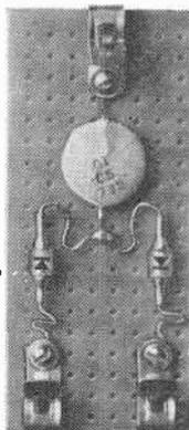
The various parts of the detector are mounted and wired on a piece of Bakelite or other insulating material. Use two general-purpose diodes of the same type, and wire them with the polarities shown. The leads can be bent to reduce the danger of damaging the diodes when you solder them to the capacitor. The 0.01- $\mu$ fd. capacitor will eliminate any possible shock hazard.
