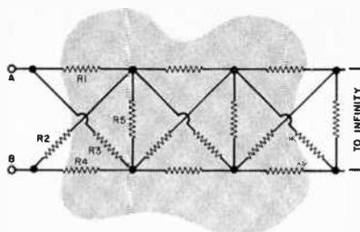
**2** Without stopping to rest, Joe went to work on *this* network of one-ohm resistors, and came up with the wrong answer. Can you do better?
