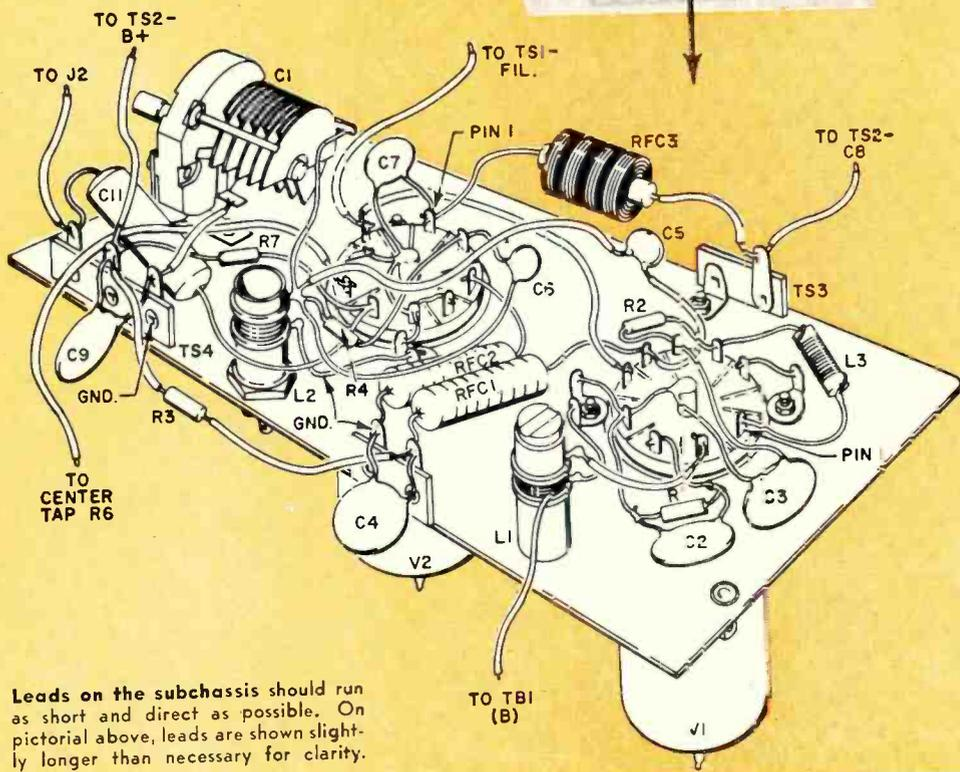
Leads on the subchassis should run as short and direct as possible. On pictorial above, leads are shown slightly longer than necessary for clarity.
