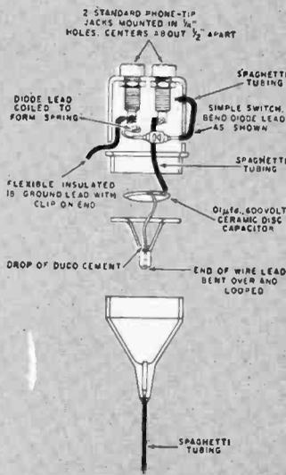
**T**HIS simple signal tracer works like a crystal detector radio. It needs no power supply and can be used for trouble-shooting in r.f., oscillator, i.f., detector, and audio stages in radio receivers, and in audio amplifier systems.
