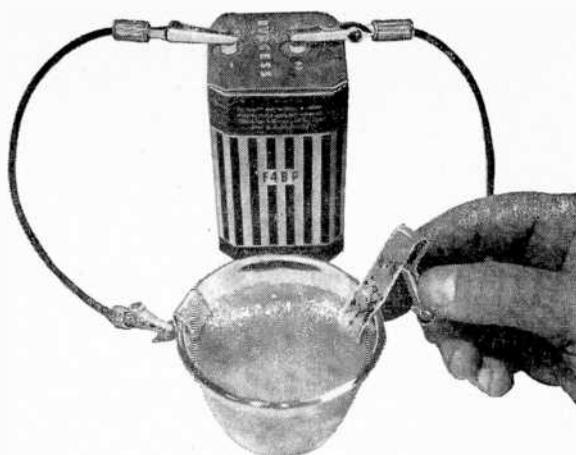
supply circuit is just the same as with battery voltage: if there is a difference of potential between points A and B underwater, no matter if the voltage is from a generator, battery, or a voltage drop in a wire, trouble can result. Use large wire for power leads to keep voltage drop close to zero. In addition, it is a good idea to connect grounded objects together inside the boat with a "bonding" wire of at least No. 10 gauge, and also bond in the engine frame and radio ground plate, if any.
