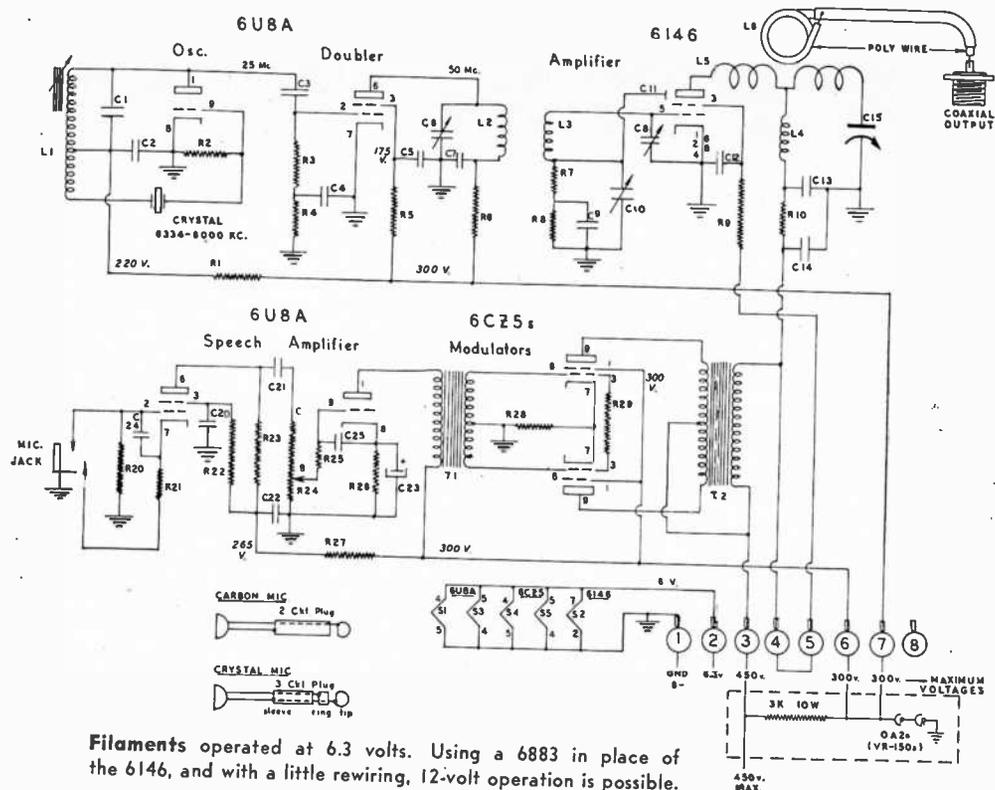
Filaments operated at 6.3 volts. Using a 6883 in place of the 6146, and with a little rewiring, 12-volt operation is possible.
