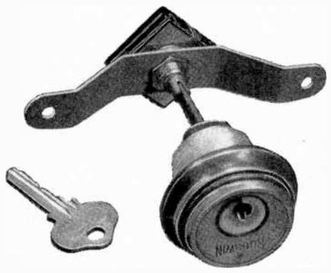
IT IS often necessary to add a lock switch to an electrical device to prevent its unauthorized use, but sometimes it is difficult to obtain such a switch. An inexpensive substitute can be made from a discarded five-pin tumbler lock of the type used on doors. These locks are of a much better quality than those in most com-
