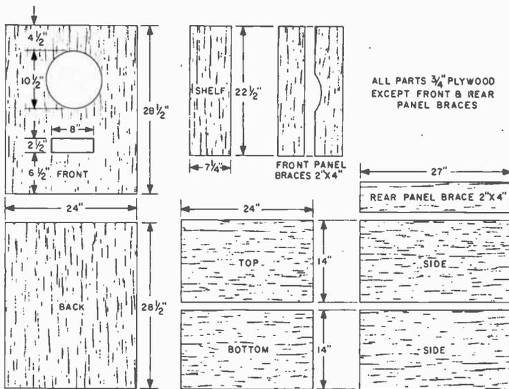
Construction of the Reflex 12 is simple since all joints are butted. At left, wooden parts are shown cut to required dimensions. Below is an exploded view of the enclosure's construction.
