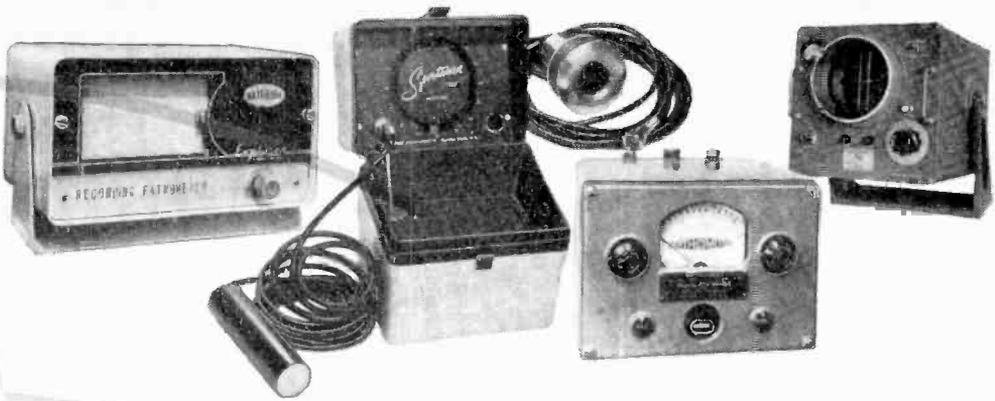
both. Others use an oscilloscope or a direct-reading meter. Depth recorders use a paper tape on which the distance to submerged objects and an outline of the contour of the bottom are recorded.
