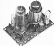
**A** RF Converter Unit (Printed circuit prewired) Two-tube crystal controlled converter. Converts Citizens frequencies to range of tunable IF. Can be used with IF unit (B) or any communication receiver. 6BA6 RF and 12AT7 mixer-oscillator. Shipping weight 2 lbs. \$14.00
