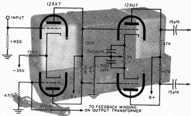
response in the front end of the power amplifier are: (1) the grid-to-plate capacitance of the tubes which acts as a bypass around the tube at high frequencies; and (2) capacitance from tube elements and wiring to ground. Obviously, the fewer the stages, the fewer the bypass points; hence, reducing the number of stages to a minimum helps the high end as well as the bottom end.
