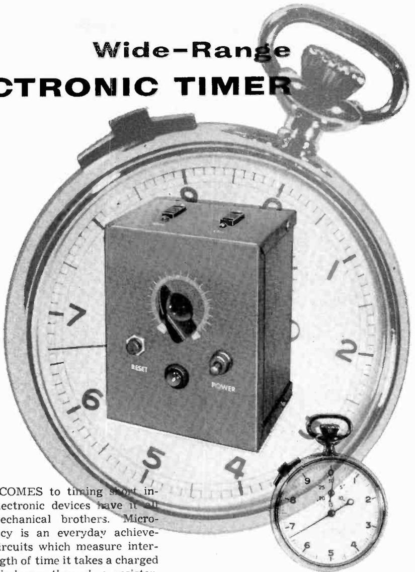
WHEN IT COMES to timing short intervals, electronic devices have it all over their mechanical brothers. Micro-second accuracy is an everyday achievement of *RC* circuits which measure intervals by the length of time it takes a charged capacitor to discharge through a resistor. However, stray current leakage paths in electronic timers can (and do) limit the timing intervals to 60 seconds or less.
