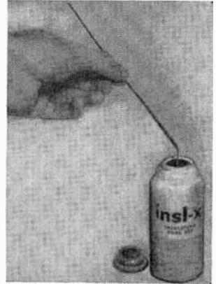
220 volts. Use a small brush to paint the insulation on wire splices that can't be dipped. A can of tool dip can be obtained at any radio parts store.—*James A. Clifford, Detroit, Mich.*
