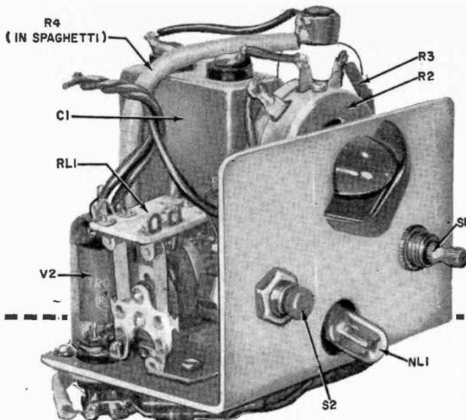
Construction of the timer is facilitated by the use of an L-shaped chassis. Unit fits into a 4" x 5" Minibox.
