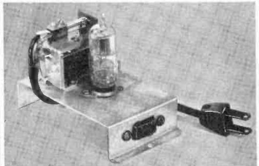
moisture, the photoelectric cell is hermetically sealed in a vacuum tube. Power-handling capacity, 1000 watts. \$9.95.
