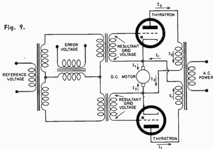
As soon as the error signal appears, the resultant grid voltage undergoes a shift of phase, possibly to the condition given in Fig. 6(C), so that a small current now flows through the motor. This current will drive the motor in the direction which reduces the error signal. If the error signal is larger, the phase shift is correspondingly greater, the conduction interval increases, and the motor turns farther and faster to correct the larger error.
