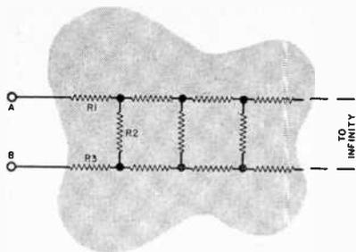
**1** Here is a tricky network consisting of one-ohm resistors with the ladder continuing out to infinity. Joe Horn computed the network's resistance at points A and B in five minutes. Can you?
