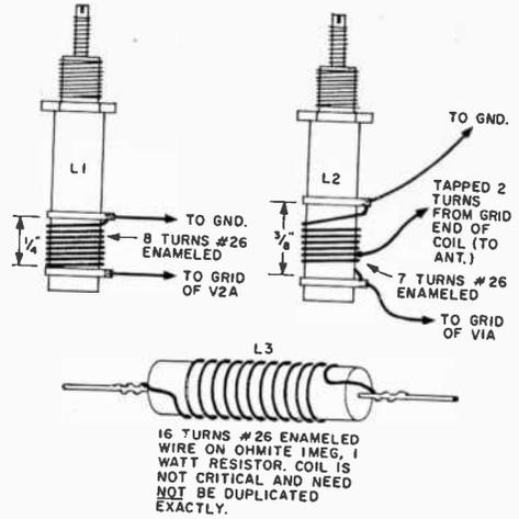
The coil forms used for L1 and L2 are Cambridge Thermionic  $\frac{3}{8}$ " ceramic slug-tuned units (Type LS-3).
