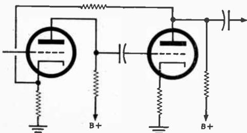
distortion of the amplifier. Although it's never possible to eliminate distortion entirely, if we use enough feedback we can come very close to it. For example, we can take an amplifier that delivers 15 watts with 2.5% distortion and, by adding 20 db of feedback, we can theoretically reduce the distortion to 0.25%.
