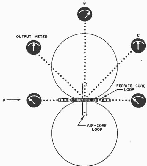
**Directional radio reception pattern of a loop antenna.** The meters show signal strength in various directions from the plane of the loop.
