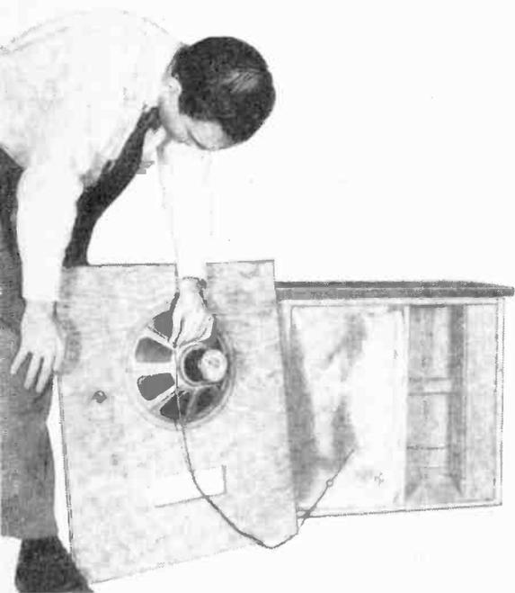
**6** Speaker is mounted on front panel with four 1/2" bolts and nuts. Speaker cable is attached to the binding posts on the speaker frame and comes out through a small hole drilled in the back panel of the enclosure.
