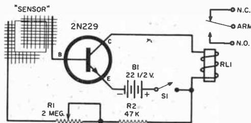
perimentation this year. Chuck has submitted a simplified photoelectric relay circuit (Fig. 1) with only five electrical components.
