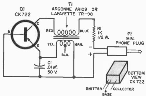
Various transistors and transformers can be substituted in the GDM modulator circuit. Changing the value of the capacitor will vary frequency of oscillation.
