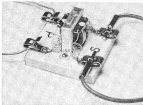
to your heart's content without worrying about broken leads. If you have miniature transformers with no screw-hole mounting brackets, simply use household cement to attach them to the wooden bases. Primary and secondary windings and impedances can be lettered on the bases in pencil or ink.—Art Trauffer, Council Bluffs, Iowa.
