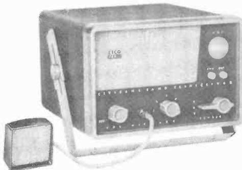
features include a 5-watt crystal-controlled transmitter, a superhet receiver with r.f. stage and noise limiter, and sealed oscillator circuit elements. Prices: Model 760 (117 volts a.c.) \$89.95 wired, \$59.95 kit; Model 761 (117 volts a.c. and 6 volts d.c.) \$99.95 wired, \$69.95 kit; Model 762 (117 volts a.c. and 12 volts d.c.) \$99.95 wired, \$69.95 kit.
