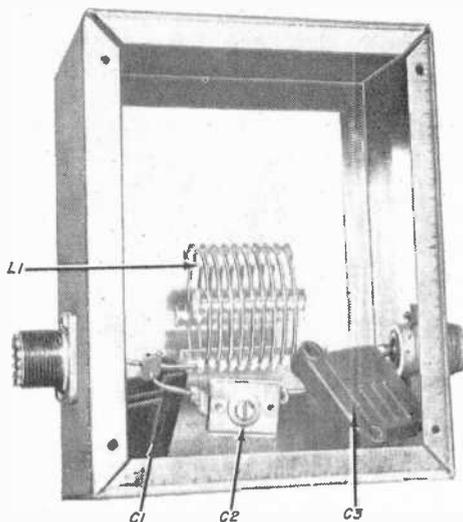
Simple filters suppress harmonics on the 80- and 40-meter bands. Chassis for 80-meter unit is large enough to hold the 40-meter filter as well.
