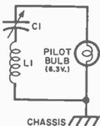
**Fig. 3.** Simple absorption frequency “meter” uses pilot lamp as indicator. The values of L1 and C1 are the same as in Fig. 1.
