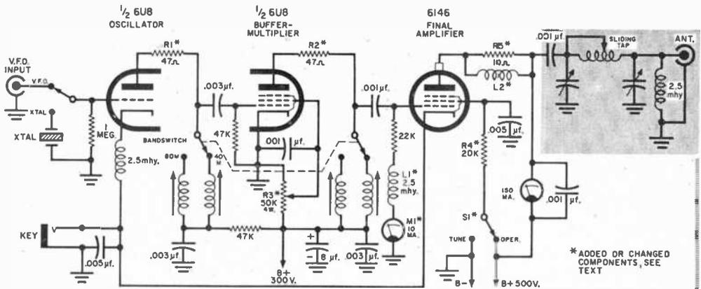
Fig. 1. Resistors R1, R2, R5, and choke L2 added to circuit of typical transmitter eliminate parasitic oscillations; increasing the value of R4 reduces screen voltage to proper value. Final tank circuit (shaded area) is modified as described in text.
