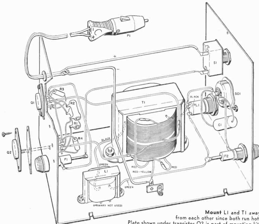
**Mount *L1* and *T1*** away from each other since both run hot. Plate shown under transistor *Q2* is part of mounting kit.
