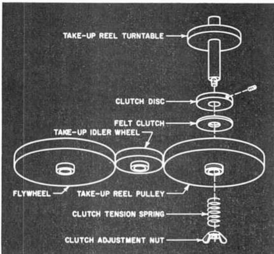
Fig. 4. Slipping-belt method for achieving a slipping drive.
