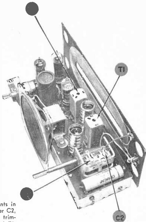
**Major alignment** adjustments in a.c.-d.c. set are mixer trimmer C2, oscillator trimmer C5, and trimmers on transformers T1 and T2.
