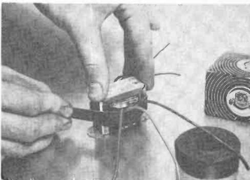
strip of tape around the transformer as shown. This will also help prevent the leads from breaking off or coming loose.—*John A. Comstock, Wellsboro, Pa.*
