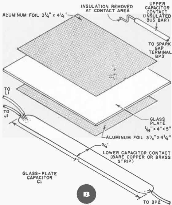
**Wiring** the unit is simple once components are assembled on 8 1/2" x 12" breadboard (see pictorial, opposite page). Detail "A" (below the pictorial) gives data on the Tesla transformer primary and secondary windings L1 and L2. Detail "B" (left) shows how to construct glass-plate capacitor C1. Wiring is point-to-point, using No. 14 insulated hookup wire.
