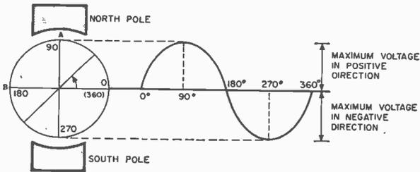
"The circle on the left," he said, "is another view of the generator. The diagram on the right represents the value of the generated voltage for any coil position. For example, in the 0° position, the coil is parallel to the magnetic field between the two poles and no lines of force are being cut. Since a voltage is generated only when the coil cuts through the magnetic field, the voltage at this point is zero. That's the way it's shown on the diagram.
