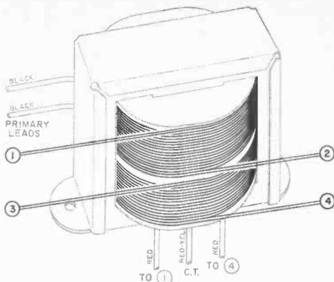
**Transformer *T1*** needs two additional windings to raise converter's output voltage. Secure windings with plastic tape.
