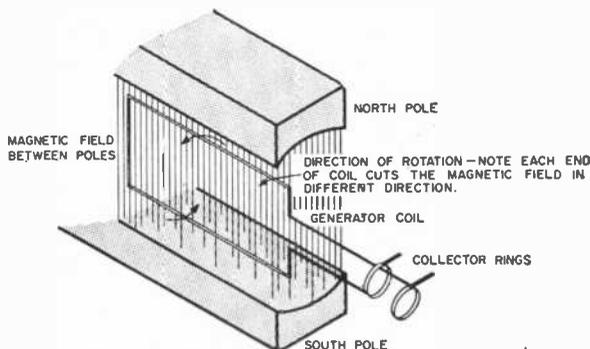
tween the two poles. Since each of the pole pieces is a magnet, one a north and the other a south pole, there is a magnetic field between them. As the coil revolves, it cuts the field and a voltage is generated in it. Current flows through the coil and is taken off at the collector rings."
