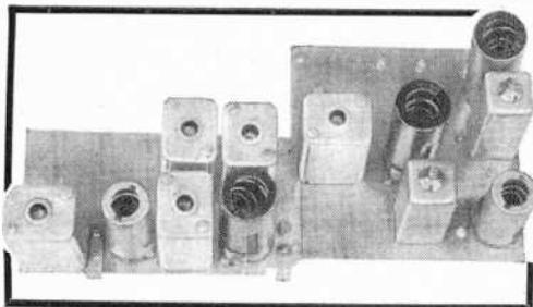
mixer, a 6BA6 second i.f. at 455 kc., and a 12AU7 infinite-impedance second detector and a.v.c. circuit.
