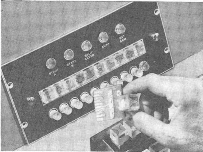
**Up to 154 effects** can be produced with this RCA special-effects generator. One of the most advanced units available, it uses plug-in modules that tell the switching amplifier when to switch camera inputs.
