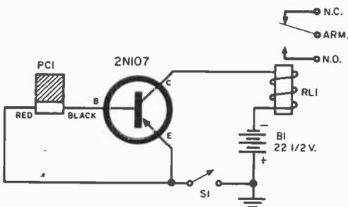
**Fig. 1.** Submitted by Chuck Van Dusen of the Fremont Junior High Radio Club, this photoelectric relay uses only five components.
