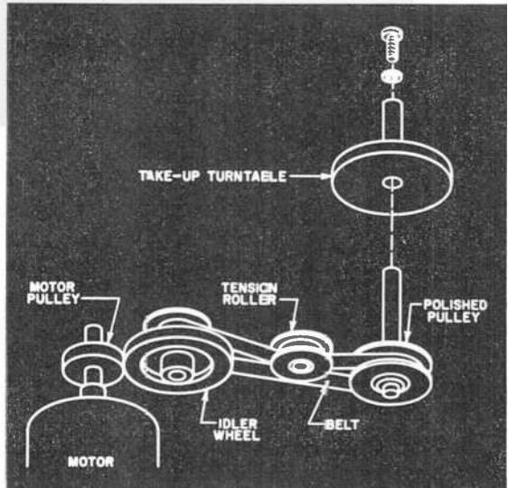
Fig. 4. In this case, the take-up reel turntable is securely fastened to a pulley which has a highly polished surface. When the load on the take-up reel increases beyond a certain point, the belt begins to slip on the pulley, reducing the speed of the take-up turntable. An adjustable tension roller maintains the correct tension on the belt. Back-tension on the supply reel is supplied by similar slipping-clutch or slipping-belt systems.
