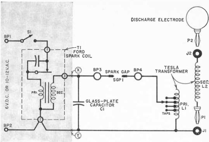
Spark coil T1 can be replaced with vibrator and ignition coil combination if desired. Parts required for vibrator supply appear as optional items in parts list; use alternate shaded schematic at lower left.
