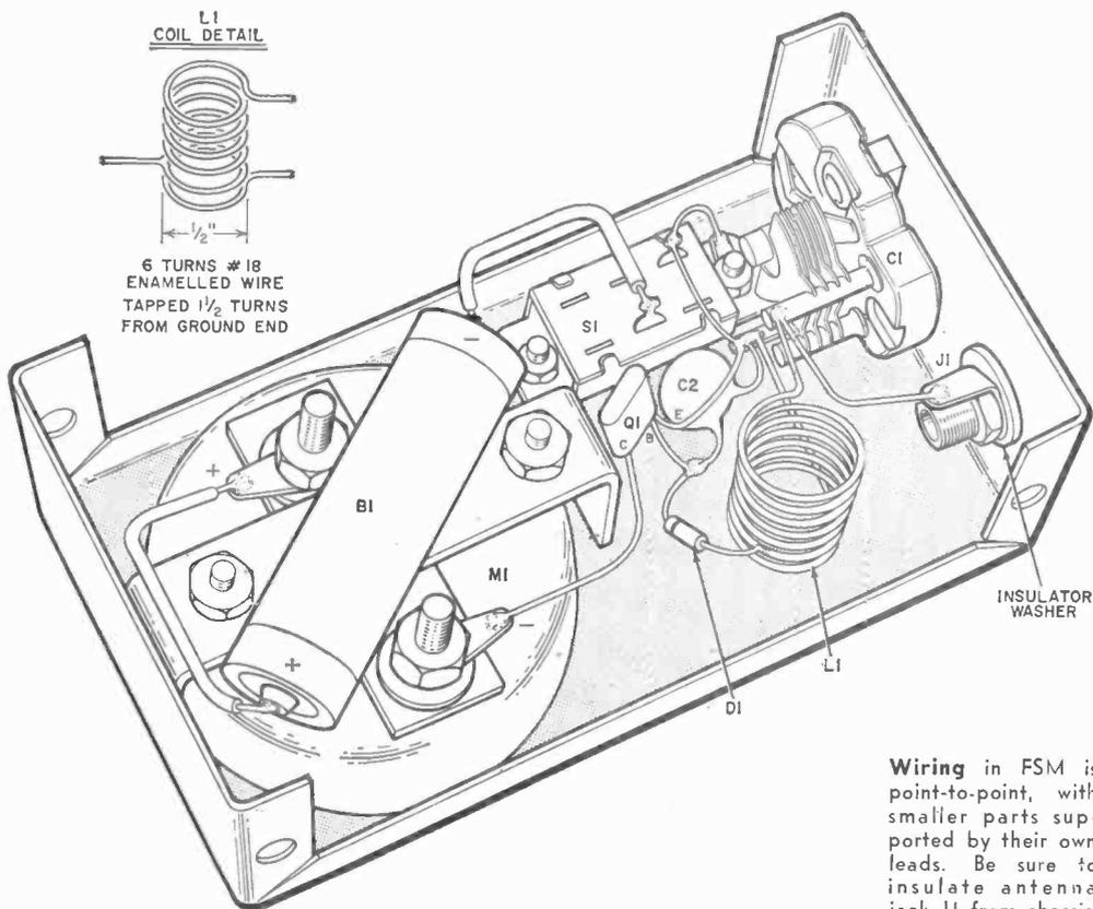
**Wiring** in FSM is point-to-point, with smaller parts supported by their own leads. Be sure to insulate antenna jack J1 from chassis.
