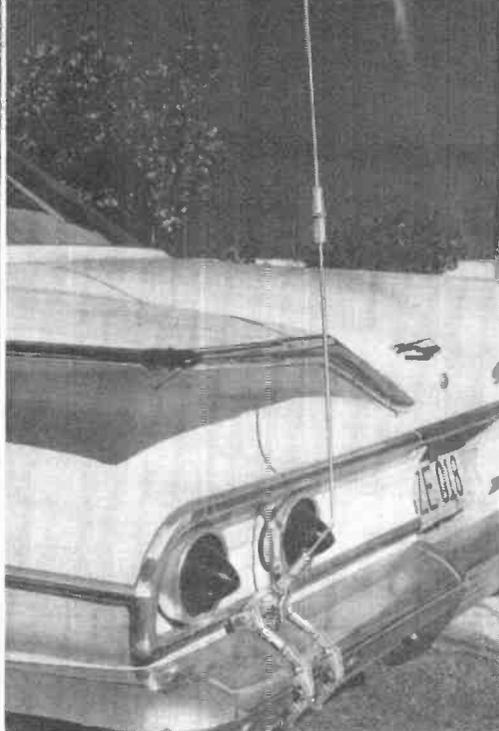
**Rack holds transceiver** (above left) at convenient distance from driver; note antenna change-over switch and field strength meter on top of dash. **Antenna bumper mount** (right) is easy to install.
