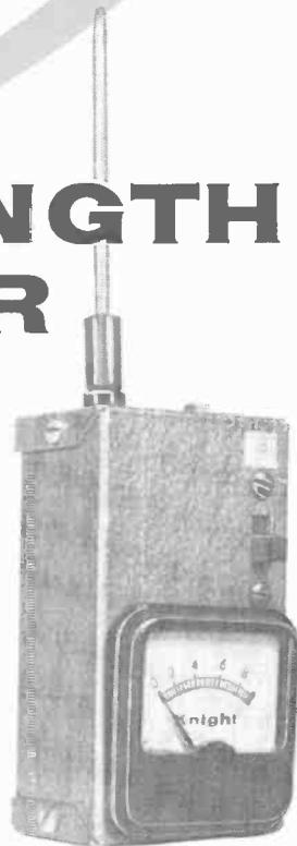
***Inexpensive device checks radiation pattern of your CB or ham antenna system***
