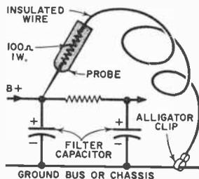
lead of the resistor to the other end of the wire. Then connect the remaining resistor lead to the probe tip. When you have turned off the equipment, fasten the alligator clip to the unit's chassis or ground bus. Then discharge all filter capacitors by touching the probe to their positive terminals for a few seconds—Clifford Marshall, Edmonton, Canada.
