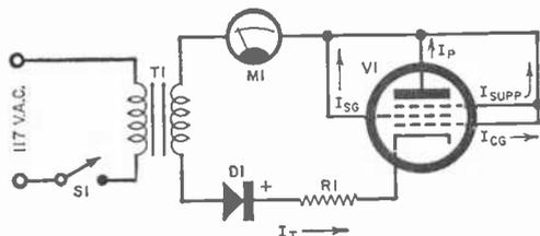
Fig. 1. Emission-testing circuit in Paco Model T-60 tester will also check for open tube elements.
