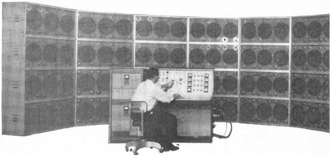
and control. Each baffle contains three low-frequency "woofers" and 12 high-frequency "tweeters." All the transducers are specially designed to deliver high-fidelity sound for sustained periods at high power levels.
