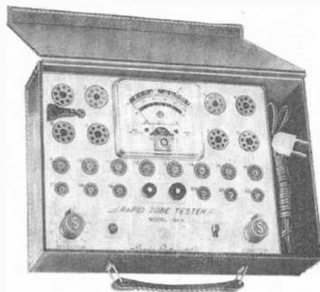
**"Quick" tester** manufactured by Superior Instrument Co. has several sockets with pin connections permanently wired to reduce pre-test adjustments.
