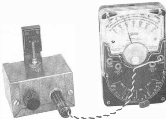
Tunnel-diode transmitter is adjusted with external millimeter to determine the diode's negative-resistance region.
