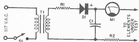
**Fig. 3.** Inter-electrode resistance measuring circuit in Heath TT-1 tester. Circuit functions as an ohmmeter to measure inter-electrode resistances to 20 megohms; external ohmmeter may be used instead.
