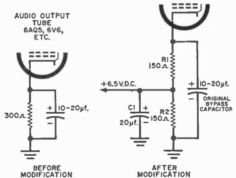
and *R2* serve as a voltage divider, and capacitor *C1* insures that no audio variations will appear in the output voltage. Any cathode-biased output tube can be used, but the output voltage will of course depend on the tube's bias and the ratio between *R1* and *R2*.—*James Romelfanger, Baraboo, Wis.*
