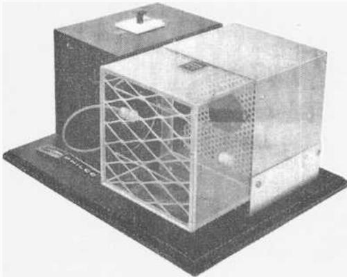
**Clinical-type** ionizer made by Philco is used in experimental work to relieve hay fever sufferers and patients with severe burns.
