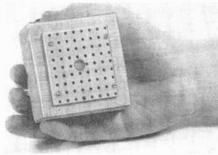
The Sentinel (above) feeds signal through power line to the pickup unit (coil on top of radio at left).
