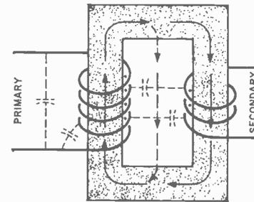
**Fig. 2.** Capacitances inherent in transformer effectively reduce high-frequency response.
