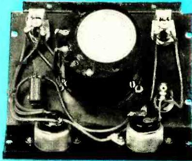
Shielded wire is used for interconnections; shields are grounded to cabinet.
