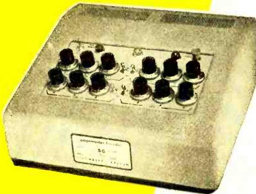
is because the signals match the vibrating reed decoder in your pocket receiver and close the circuit that actuates the "beep." When you hear the "beep," you know someone wants you on the phone. So you simply go to the nearest telephone booth and call the *mobile service operator* or a prearranged number.
