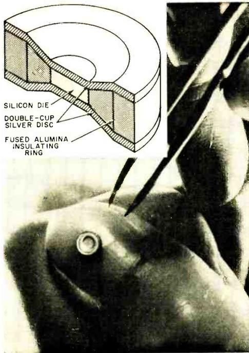
**Fig. 2.** Cross-sectional view of the "Sildisc" diode developed by Controls Company of America. It features a new type of construction that provides maximum heat dissipation. Photo shows a typical unit.
