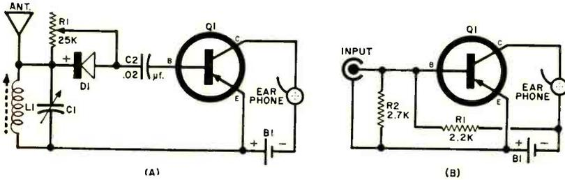
**Fig. 1.** Simple circuits evolved by reader Richard Bond using low-cost "experimenters'" transistors: (A) broadcast-band receiver; (B) general-purpose amplifier; (C) code practice oscillator.
