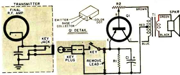
**Keying monitor** draws its power from the cathode circuit of the transmitter's final; setting of potentiometer R2 controls the tone of the note. The unit can also be employed as a code-practice oscillator if resistor R1 and capacitor C1 are replaced with a 1/2-volt battery as described in text.
