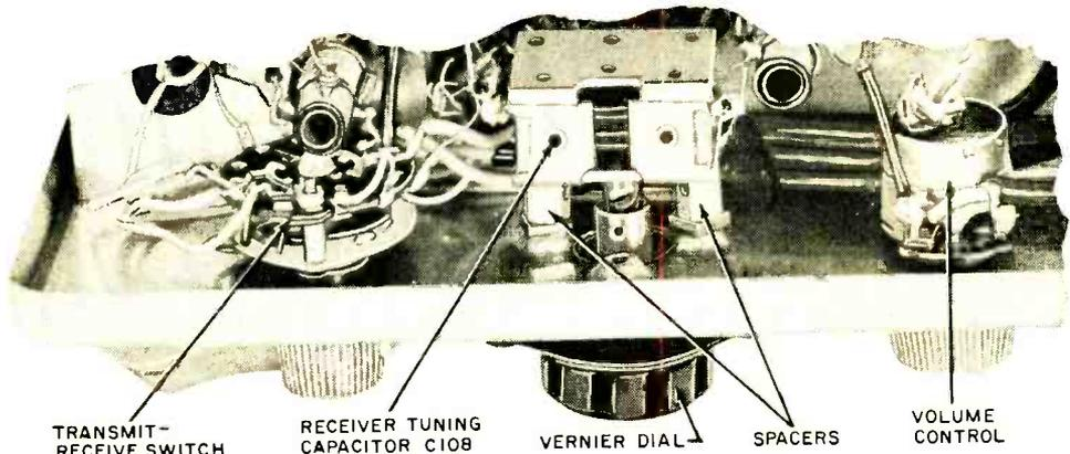
Tuning capacitor C108, above, is remounted to front panel with spacers; shaft is modified to fit vernier dial.
