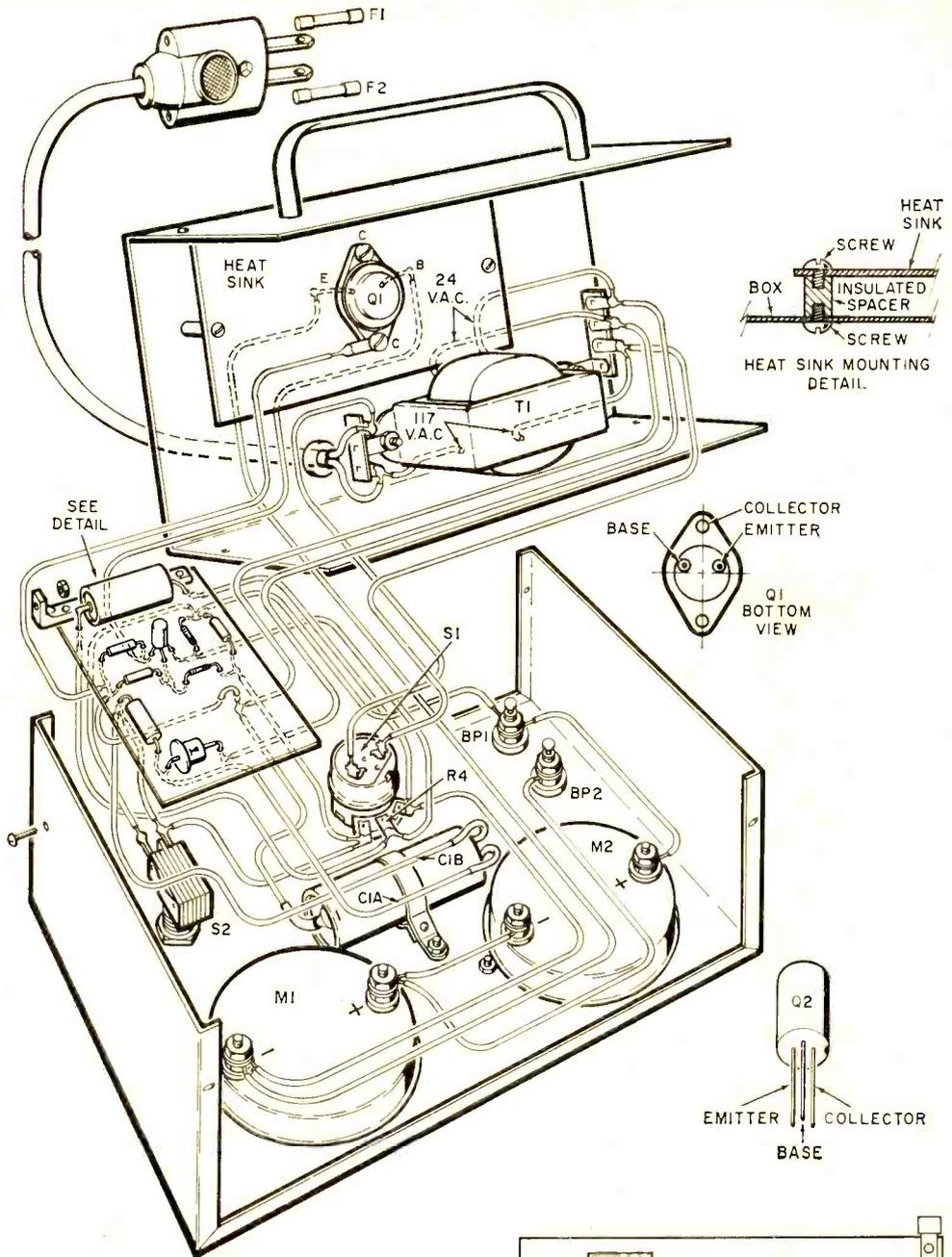
The power supply is built into both halves of the aluminum box. Power transistor Q1 mounts on heat sink which is insulated from box. Perforated phenolic circuit board (detail at right) mounts small components and is fixed to the chassis by means of an L-bracket.
