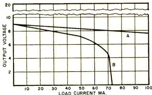
**Regulation** with guard circuit out is maintained within 2 volts from 0 to maximum load (A); with guard circuit in, regulation falls off above 70-ma. load (B).
