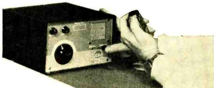
“Phase detector of the Moving Target Indicator receiver misaligned on the FPS-3...realignment procedure must be followed.”
