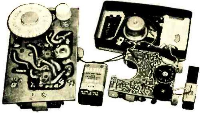
substance called a "resist" is applied to the copper wherever conductors are to be located on the final board. The entire sheet is then dipped into an acid bath which eats away the copper not protected by the resist.
