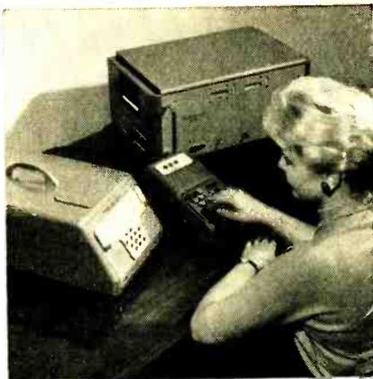
**Three-part** psychomotor skill trainer of Rheem Manufacturing Company includes: (1) a program display unit; (2) a standard IBM keyboard; (3) a computer control unit.
