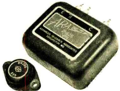
"Composite" transistors, introduced by Advanced Research Associates, have extremely high gain. Note size of unit at left compared with a conventional power transistor.
