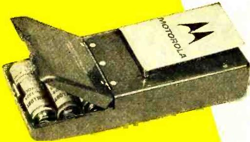
**Radio paging receiver** is carried by each individual in a remote paging system. This completely transistorized superheterodyne unit, made by Motorola, delivers 1/2-watt output to built-in speaker.
