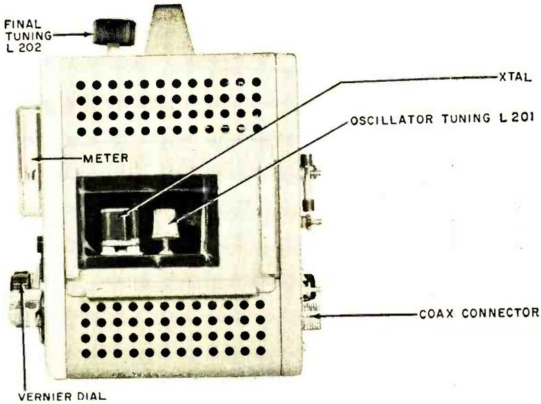
Side hole in cabinet permits rapid crystal change; oscillator and final tuning controls peak transmitter on new crystal frequency; meter indicates plate current. Vernier dial and coaxial connector jack are optional.
