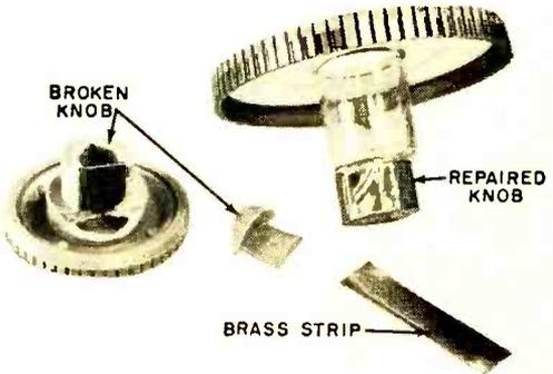
around the broken portion and solder the ends of the strip together. Use a minimum of heat when soldering to prevent damage to the knob. Flat strips of brass can be obtained from automobile parts dealers who sell this material for shimming purposes.—*H. L. Davidson, Fort Dodge, Ia.* —30—
