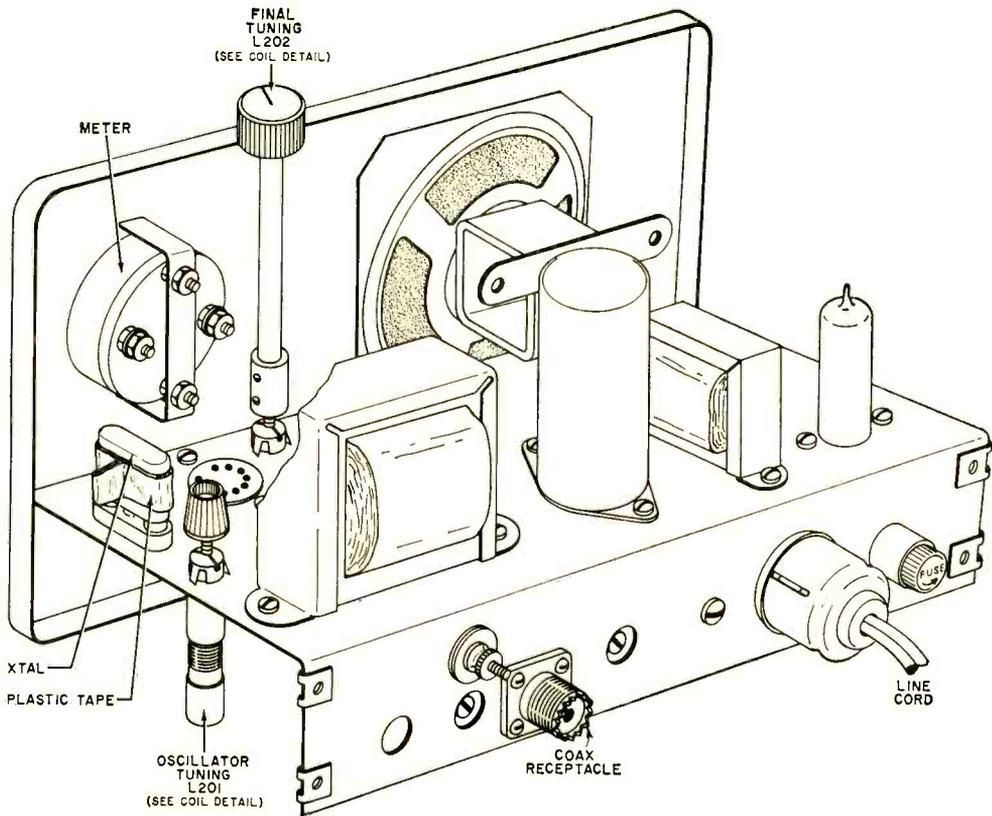
Use very small knob on coil L201. Shaft coupling set screw tightens on the nut soldered to the top of coil L202.
