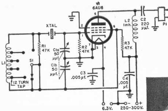
**Unusual oscillator** is crystal-controlled, yet offers features of VFO. Entire circuit can be assembled on front panel of a small metal box.
