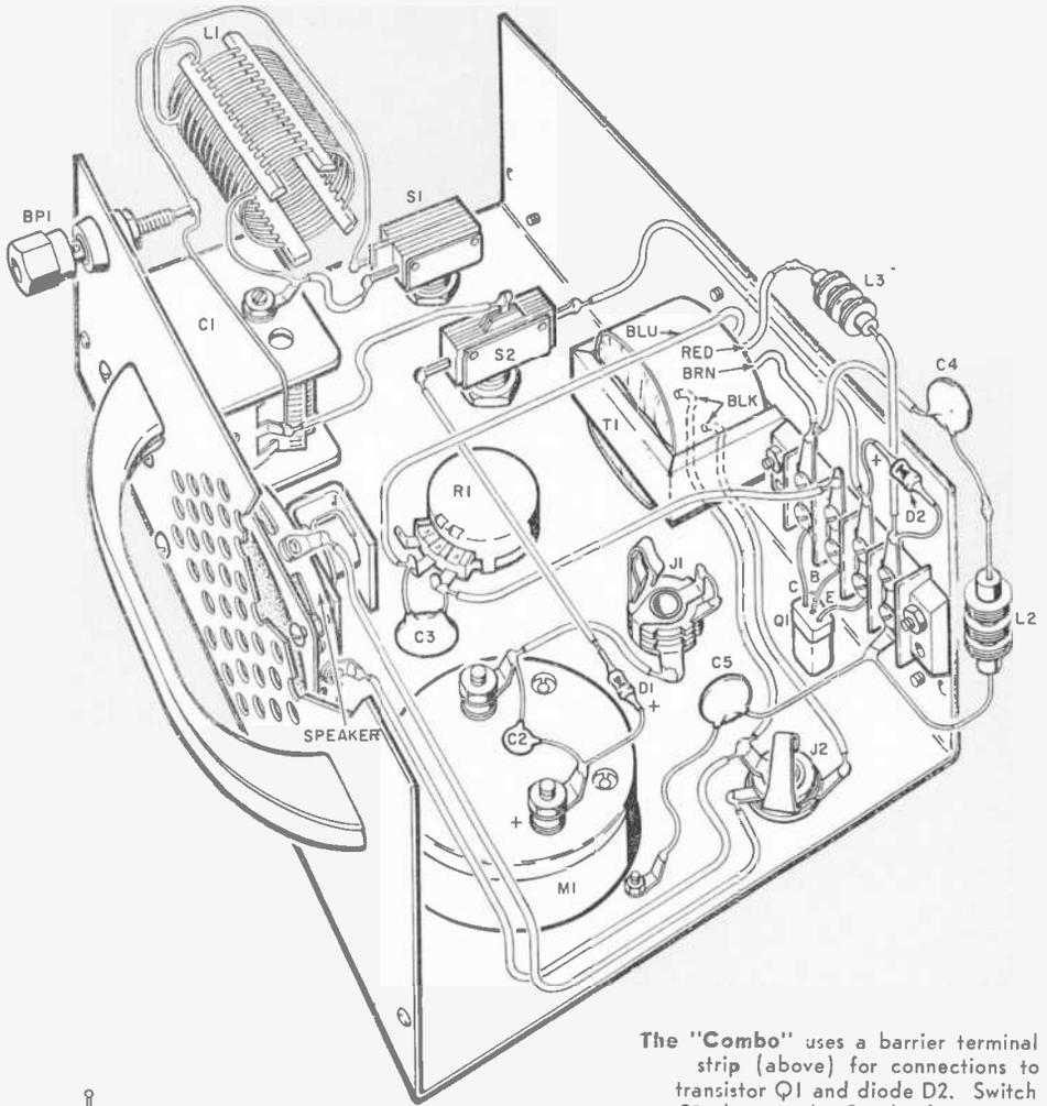
The "Combo" uses a barrier terminal strip (above) for connections to transistor Q1 and diode D2. Switch S2 changes the Combo from a c.w. monitor to an F.S.M. and phone monitor; S1 is a bandswitch.
