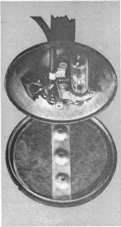
**Wiring** for the time delay relay is hidden in the base of a desk-type telephone stand. Thermostatic delay relay *K1* (glass bulb) mounts in nine-pin miniature tube socket to right of on-off switch *S1*.
