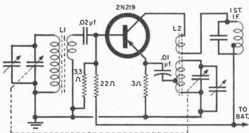
**Converter stage** of typical portable makes use of a ganged tuning capacitor, with separate trimmer capacitors paralleled across the oscillator (coil L2) and the mixer (coil L1) sections.
