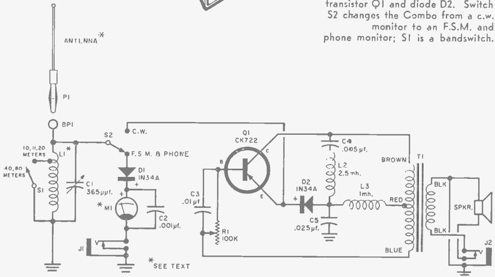
from the coil stock as purchased and unwind two turns on each end of the cutoff section (leaving 18 turns). The lengths of wire on either end of the coil will make wiring easier: Now solder a 2" length of bare hookup wire to the third turn from one end of the coil. To make the tap easily, push in the second and fourth turns on either side of the tapped point, then solder the bare wire to the desired turn.
