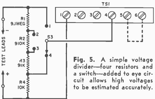
**Fig. 5.** A simple voltage divider—four resistors and a switch—added to eye circuit allows high voltages to be estimated accurately.
