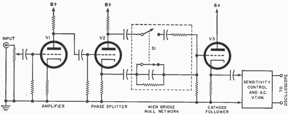
**Simplified schematic** of Heath HD-1 distortion analyzer. Heart of unit is the Wien bridge null network between tubes *V2* and *V3*; it cancels equal but out-of-phase signals, leaving only distortion component.
