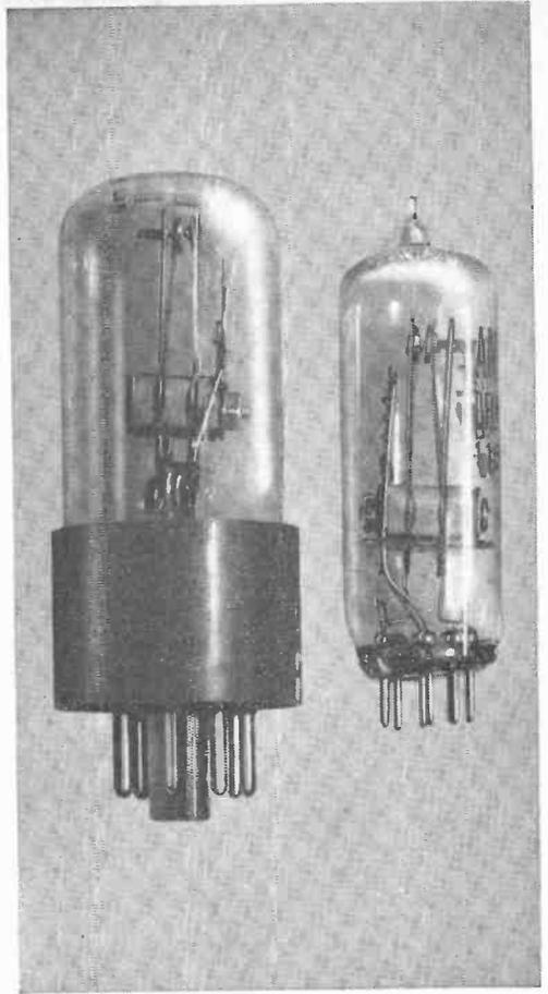
Thermostatic delay relays are available in several models. Amperite relay with octal base (at left) has 3-amp. contacts; nine-pin miniature model (right) used here has 2-amp. contacts. See text.
