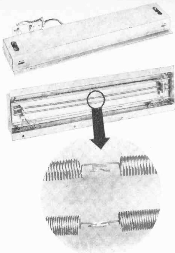
**Mechanical delay device** produced by the Hammond Organ Co. is basic component in artificial reverberation units. Signal is fed to ferrite transducers at one end of box, through special springs, then on to another pair of ferrite transducers. To minimize uncontrolled reverberation—footsteps jarring springs into extra action, for example—each spring consists of two sections wound in opposite directions and coupled at the center.
