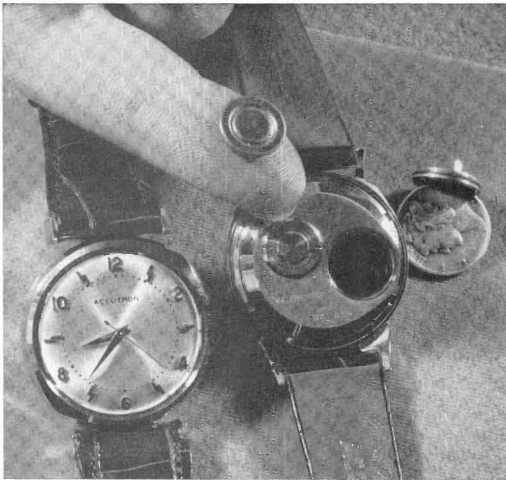
**A** NEW sound of time—a "microsonic" tone to replace the centuries-old ticking sound—is given off by a new Bulova Watch Company timepiece called the "Accutron." Guaranteed accurate to plus or minus one minute per month, this transistorized device is about ten times as accurate as a conventional fine-quality wristwatch.
