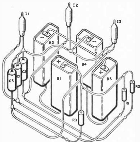
circuit to the battery should cause all of the bulbs to start flashing, with a different flashing rate for each bulb.
