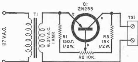
**Setting** of potentiometer R2 governs rectifier's output voltage and polarity. Voltage can be increased by moving R2 toward either end of range.
