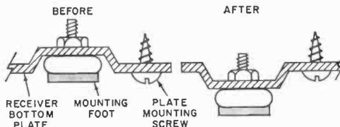
in the same holes, as shown. This process will raise the bottom plate screws at least 1/4" and prevent further scratching.
