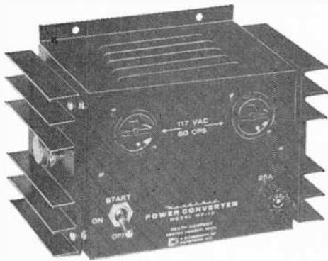
volt, 60-cycle a.c., and can feed two appliances simultaneously through its two outlets. Power rating with a 12-volt battery is 175 watts continuous, 240 watts maximum; with a 6-volt battery, 120 watts continuous. The entire unit is fused. Price, \$29.95.
