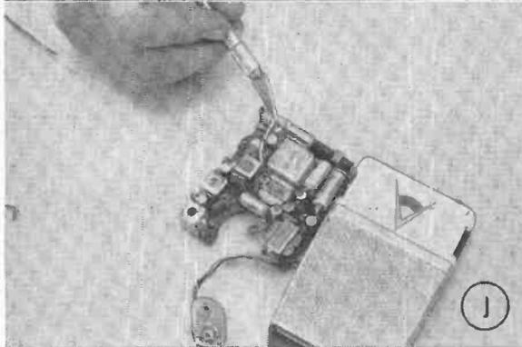
tenna. Coat the soldered connections with fingernail polish so that they don't short to any other components (I). Finally, replace the loop in its plastic clips and reassemble the radio (J).
