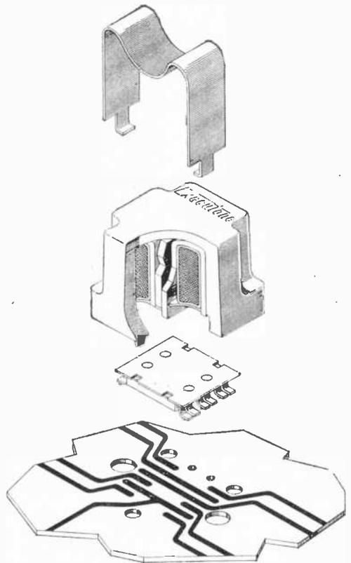
"Printact" relay snaps onto printed-circuit board (as shown in exploded view). Printed conductors form stationary contacts.
