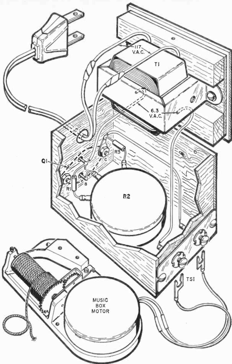
Housed in a small wooden box, the current reversing rectifier makes an ideal power source for a 1.5-volt d.c. music box motor. Metal reed assembly on music box movement can be removed so that drum may be used as winch for model toys.
