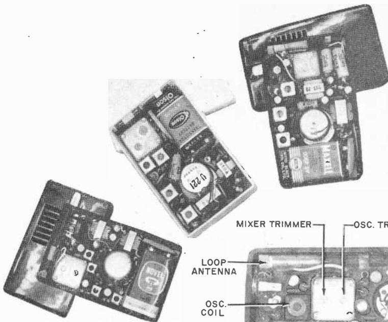
A variety of miniature receivers, all having the same general layout, can be modified to pick up the 2182-kc. frequency. Shown above, left to right, are the Olson Radio RA-373, Radio Shack "Petite," and Lafayette Radio FS-208. Call-outs at right apply to Lafayette's FS-91.
