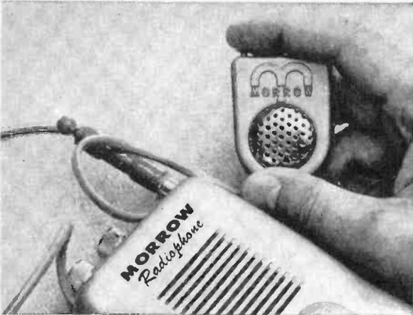
The microphone of the Morrow VP-100 can be clipped to a shirt pocket, the main unit attached to operator's belt.
