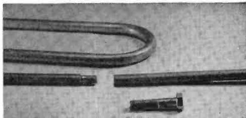
and push it into one end of the broken rod; the other end of the broken rod fits on the protruding portion of the bolt. Crimp the broken ends with a pair of pliers, and, if possible, solder the joint, using a good brand of aluminum solder. Then wrap a few turns of plastic tape over the repaired portion.
