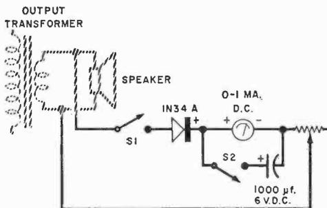
milliammeter or substitute a 0-100 volume unit (VU) scale. The potentiometer should be about 20,000 ohms for audio outputs of 30 watts, and a correspondingly smaller resistance should be used for lower power outputs. Adjust the potentiometer to give maximum meter deflection at full output.
