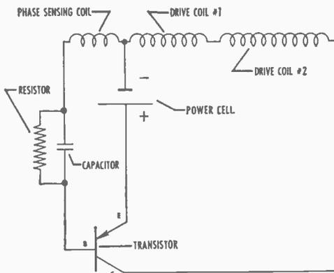
is at a maximum and opposite in polarity to the power-cell voltage. If the tuning fork's amplitude is high and the induced voltage equals the power-cell voltage, no current will flow and the amplitude will drop. If the fork's amplitude is low, the induced voltage will be low—more current will flow in the drive coils and bring the amplitude up to normal.
