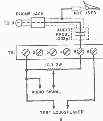
Fig. 3. Setup for using the receiver as a code oscillator (A); and as an audio signal source and test loudspeaker (B).
