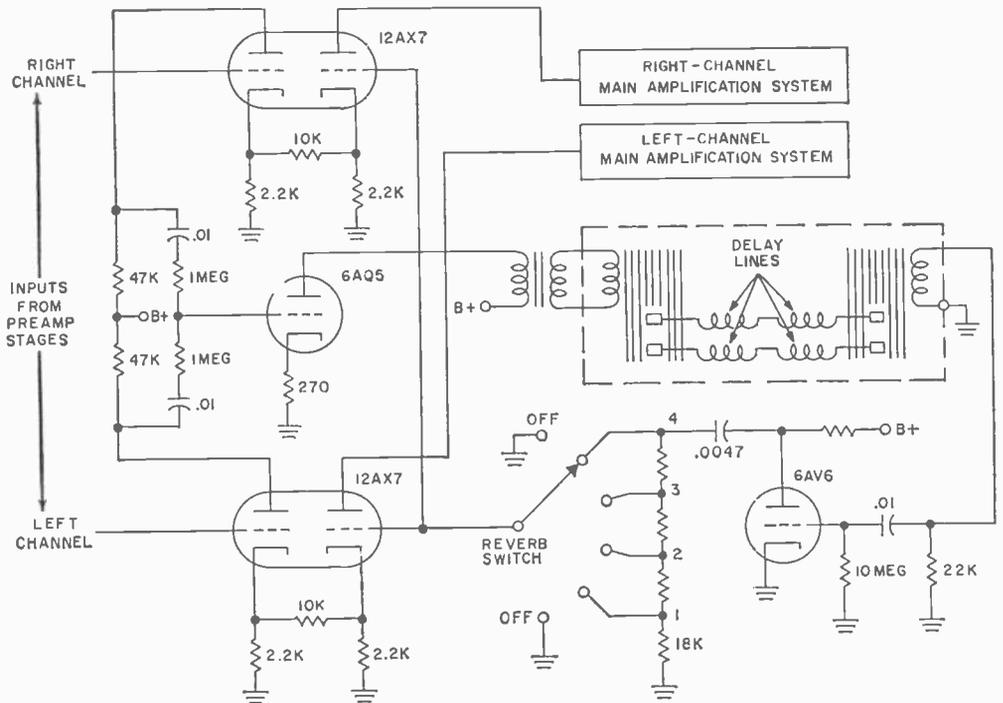
**Circuit diagram** of Philco's "reverbaphonic sound system" is typical of electronic control devices employed with the Hammond mechanical delay unit. Switch controls degree of reverberation in 6-db steps.
