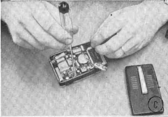
the board by sliding it out of its plastic retaining clips (E). Cut the lead connecting the single-wire end near the coil (F), and remove 44 turns from this end of the loop. Then scrape carefully (G) and tin both the cut-end of the antenna wire and the original yellow lead.
