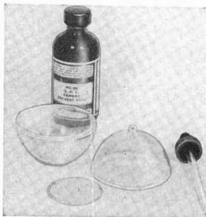
**Plastic hemispheres** are cemented together to form satellite's body. Pip on lower hemisphere fits into matching hole in base.
