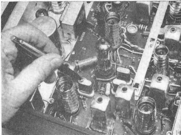
Printed-circuit wiring (left) in C-27 simplifies assembly; pen points to 22.61-mc. crystal in first oscillator of double-conversion receiver. Pres.-to-talk bar (below) coupled to relay switches speaker for use as microphone.
