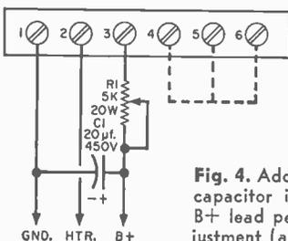
**Fig. 4.** Adding a resistor and capacitor in series with the B+ lead permits voltage adjustment (as well as filtering).
