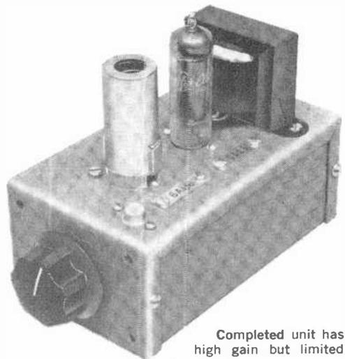
Completed unit has high gain but limited frequency response, a useful combination for signal tracing and speech amplification.
