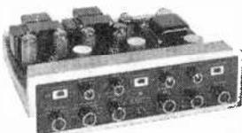
**LK-72 72 Watt Integrated Stereo Amplifier Kit**
