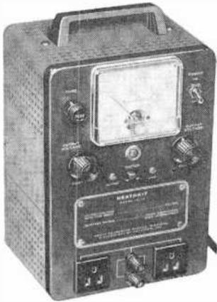
(300 watts continuous duty, 500 watts intermittent), improved meter accuracy ( $\pm 1$  volt), and new styling. The IP-10 completely isolates equipment under test from the a.c. line. Output is variable from 90
