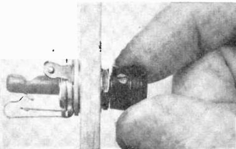
the other end with a file. You'll find that pushing the rod all the way into the jack will open the contacts, pulling it out slightly will close them. For a rotary
