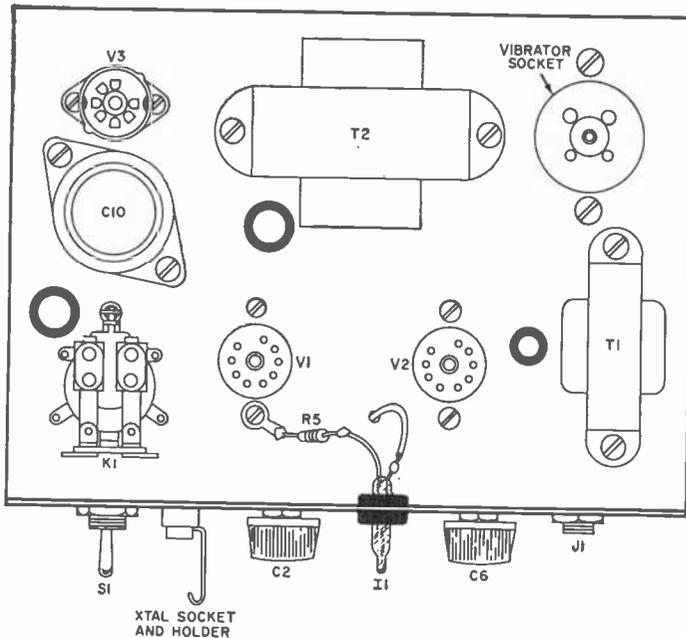
Drawing of top of chassis, with case removed. Neon bulb *V1* serves as a tuning indicator and is held in place by a rubber grommet; *R5* is soldered directly to one lead and attached to a solder lug under a screw at *V1*'s socket.
