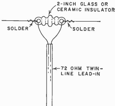
Fig. 5. Install 72-ohm line as you would a TV twin-lead. Fix lead-in to mast a few feet below the connections, to prevent wire's weight from bending loop.
