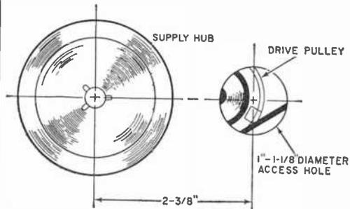
chassis punch, positioning the hole as shown in the diagram. To change speeds, turn off the motor and place the mechanism in the "rewind" position. Slowly rotate the supply hub to turn the drive pulley while using a hook bent from a stiff iron wire to guide the belt into the proper groove. During operation, the hole is covered by the supply reel and does not detract from the appearance of the machine.
