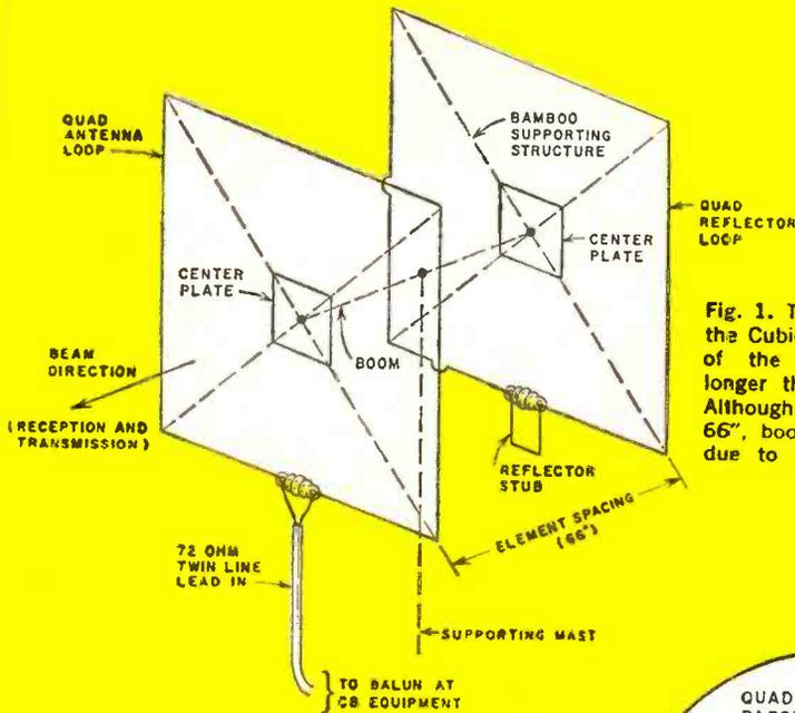
Fig. 1. The designer's "eye view" of the Cubical Quad antenna. Each side of the square loops is slightly longer than one-quarter wavelength. Although spacing between loops is 66", boom will be about 1" shorter due to thickness of center plates.
