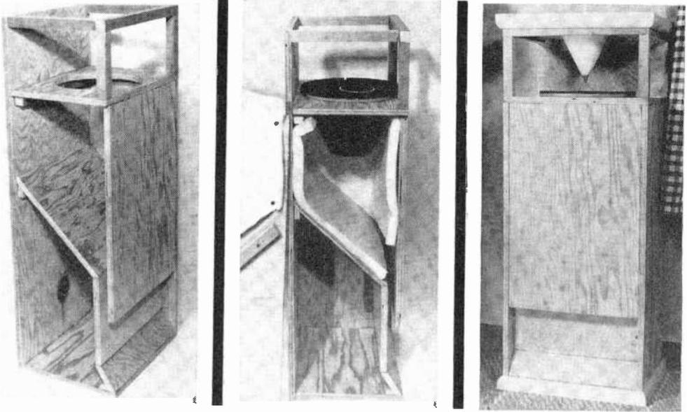
Constructing enclosure is actually rather simple, if you follow the step-by-step instructions outlined in text. One side was removed (left and center) to show the internal layout better.
