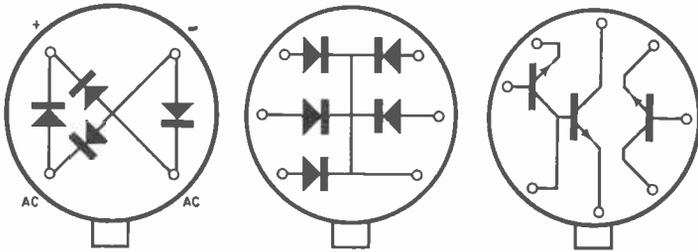
Fig. 1. Schematic diagrams of typical circuit packages produced by Fairchild Semiconductor Division. Four diodes at left are connected in bridge rectifier circuit, while five diodes in center have common cathode connection for use in logic circuits; three transistors at right (two in cascade) are intended for use in subminiature amplifiers. Diodes at left are assembled in a TO-18 package, other two circuits in TO-5 case.
