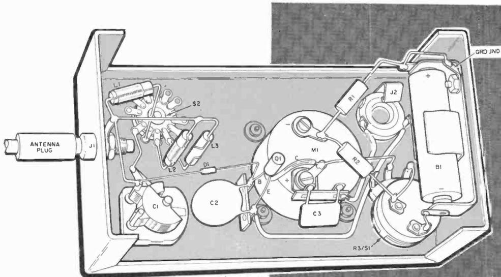
Small metal utility box houses and shields FSM parts. The leads of coils L1, L2 and L3 should be as short and direct as possible. Notice that the polarity of mercury battery B1 is unusual; the casing is positive and the insulated center disc is negative.
