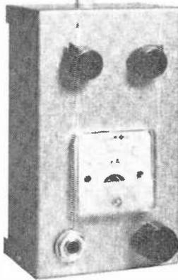
The FSM has headphone output jack for use in checking transmitter's audio quality. Plugging in headphones does not change sensitivity of instrument.
