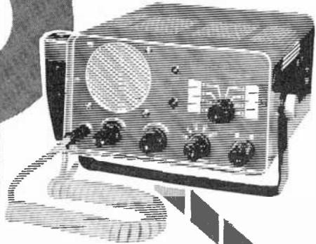
8-channel transmitter with 8-channel crystal-controlled or tunable receiver; universal power supply (117, 12 and 6 volts); 8-tube function receiver (one r.f. and two 455-kc. i.f. stages)—plus 2 diodes; series noise limiter; adjustable squelch; un-metered; ceramic mike; 9 lb.; 4 $\frac{3}{4}$ " x 9 $\frac{1}{4}$ " x 11 $\frac{1}{4}$ ". 5-meter available as accessory (\$24.95).
