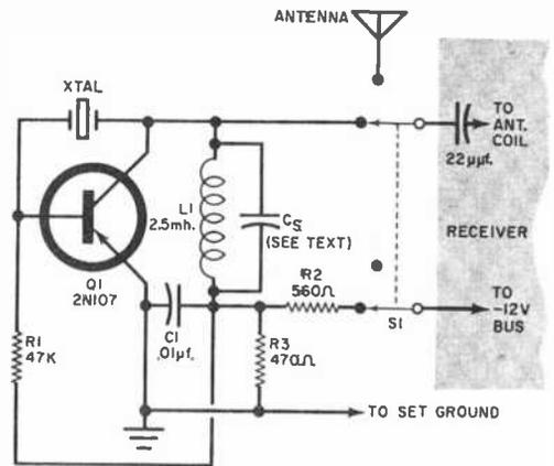
Fig. 2. Circuit of 1-mc. crystal calibrator submitted by reader B. E. Henry. Power for the device is supplied by the receiver, as explained in text.
