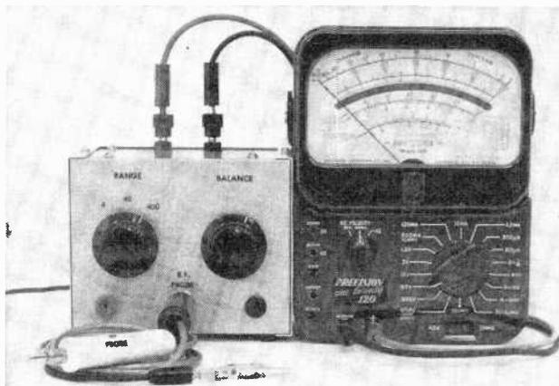
The adapter connects to the multimeter's existing input jacks as shown at left. It can be removed at any time if you want to use the multimeter in the normal way.
