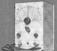
A "must" for aligning and trouble-shooting receivers. Build it for your own use. 170 KC to 50 MC fundamental frequencies for all radio and TV work.
