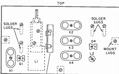
Detail of circuit board, showing location of parts. Coil L1 (dotted lines) is located underneath board.
