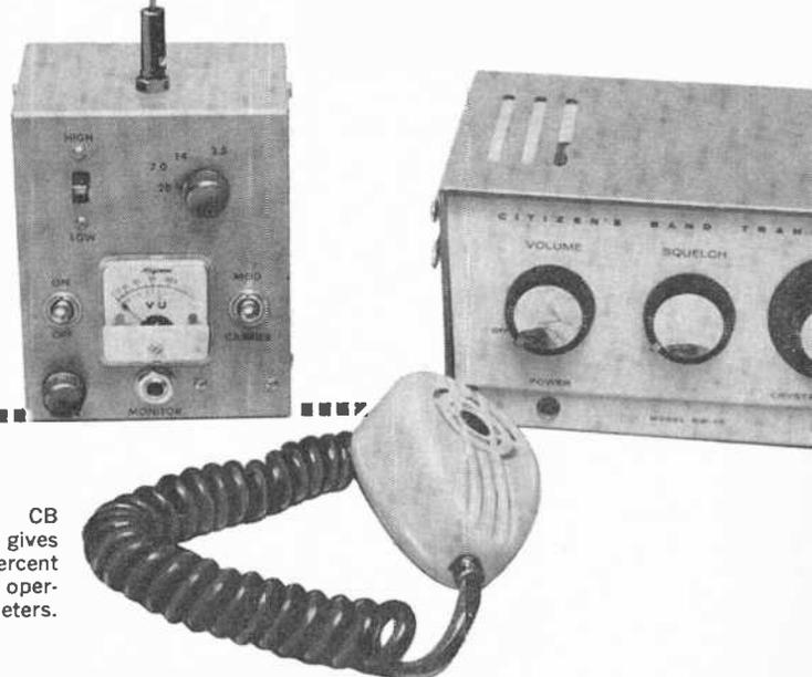
Particularly useful with CB rigs, the Monitor Meter gives continuous indication of percent modulation for transmitters operating between 80 and 10 meters.
