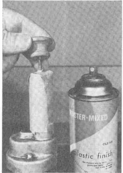
**5** Any rotary device, such as the electric drill shown here, can be a big help in spraying small parts evenly.
