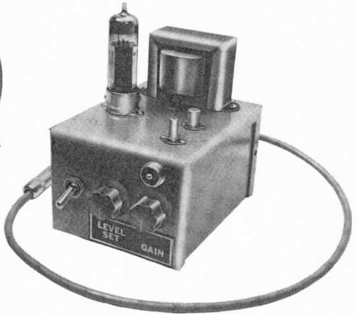
**H**ERE'S a simple modulator specifically designed for amateur transmitters whose plate current during c.w. operation is 120 ma. or less. Compact in size as well as easy to install and remove, it can be used with almost any small transmitter having a keyed final amplifier. Powering the modulator is no problem, since the entire unit—with the exception of the 6BQ5 heater—receives
