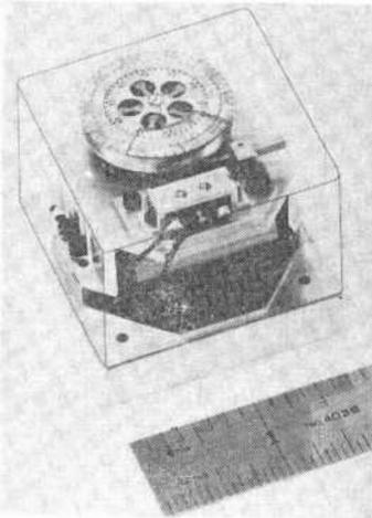
It worked—this time! The electronic timer built into Explorer VII failed to shut off the transmitter on 19.99 mc. in October, 1960. A similar timer installed in Explorer XI worked perfectly and switched the satellite to a new experimental program in late May. Explorer XI operates on 107.97 mc.
