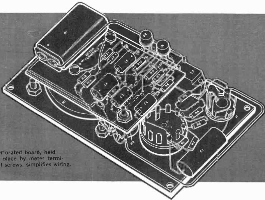
Perforated board, held in place by meter terminal screws, simplifies wiring.
