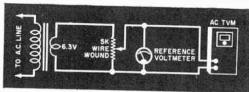
Suggested circuit for calibrating the voltmeter.
