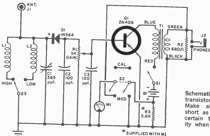
Schematic diagram of one-transistor Monitor Meter. Make all r.f. leads as short as possible, and be certain to observe polarity when wiring diode D1.
