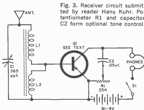
Fig. 3. Receiver circuit submitted by reader Hans Kuhr. Potentiometer R1 and capacitor C2 form optional tone control.
