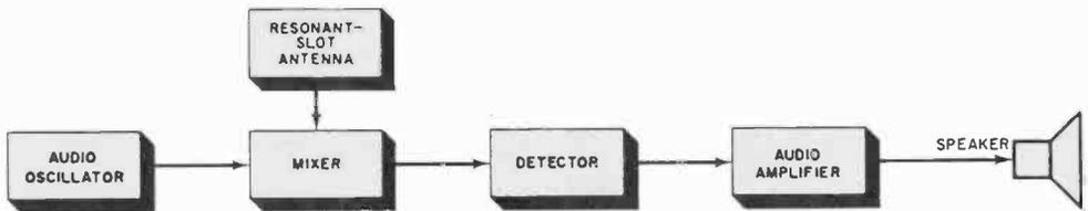
Block diagram of Sentry's circuitry. Audio oscillator (at left) is actually a square-wave "flip-flop" oscillator, which "chops" incoming signal approximately 700 times a second to produce an audible tone.
