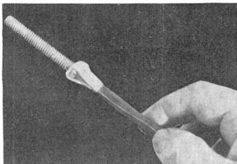
the size of the threaded part of the bolt or screw in a small strip of cellophane or masking tape, and pass the threads through the hole with the sticky side of the tape facing the head. Finally, draw the ends of the tape up and stick them to the blade;
