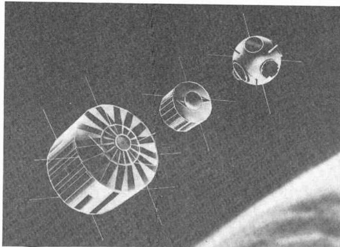
Power to operate four of the six transmitters in the June 29 launching comes from silicon solar batteries. Two transmitters on the Transit IV-A satellite are powered by a nuclear thermoelectric generator.
