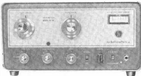
The HT-40K is Hallicrafters' first entry in the transmitter kit field. Covering six bands, the crystal-controlled unit is rated at 75 watts input on both c.w. and phone. Interior layout is neat, and the well-illustrated instructions are easy to follow.
