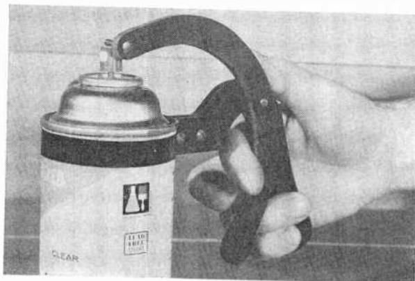
**2** Handle-and-trigger assembly removed from an old coffee maker enables you to hold and aim a spray can in "pistol-fashion."
