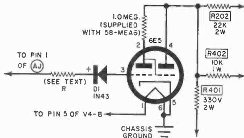
You will probably find it necessary to experiment with the value of the resistor ( $R$ ) which is inserted between diode  $D1$  and the antenna jack, terminal 1; it might range anywhere from 2700 to 270,000 ohms. If the eye closes too much, increase the value of  $R$ ; if it doesn't close enough, decrease the resistance. Strive for a  $\frac{1}{4}$ "-wide shadow when the CB-1 is tuned up and the antenna loaded. Modulation peaks should further decrease the shadow width.
