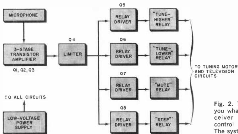
Fig. 2. This block diagram shows you what goes on inside the "receiver in the Zenith remote-control setup for home TV sets. The system uses eight transistors.
