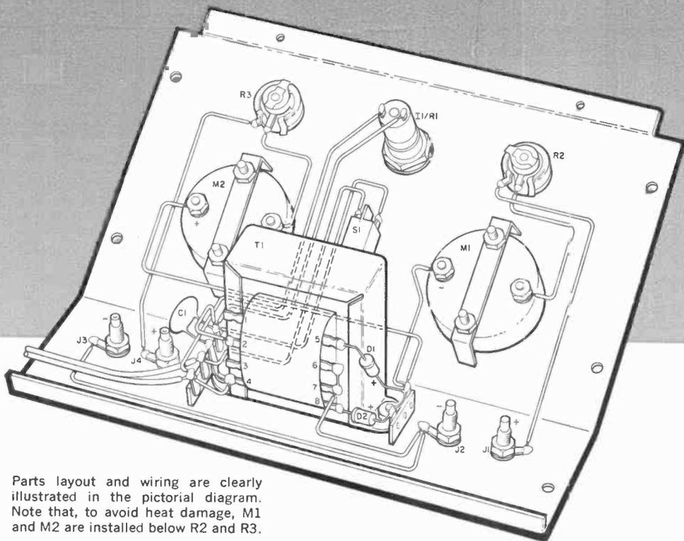
Parts layout and wiring are clearly illustrated in the pictorial diagram. Note that, to avoid heat damage, M1 and M2 are installed below R2 and R3.
