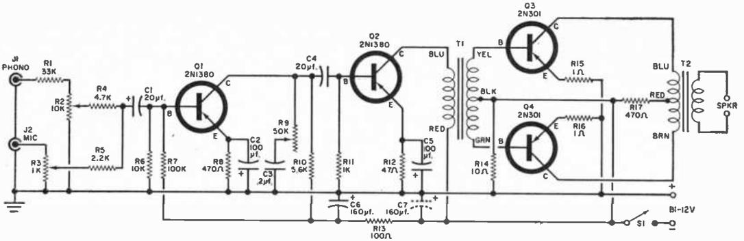
Fig. 4. Schematic diagram of amplifier. Capacitor C7 (shown dotted) mounts on underside of board; like other electrolytics, it should be rated at 15 v.w.d.c.
