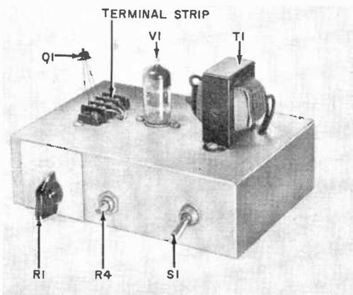
Fig. 2. Top view of thermostat. Transistor is connected to a barrier-type terminal strip.
