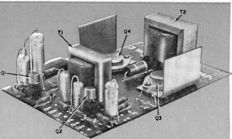
Fig. 1. You'll find construction a "snap" if you use the special printed-circuit board. Heat sinks for power transistors Q3 and Q4 can be cut out from an old aluminum chassis.
