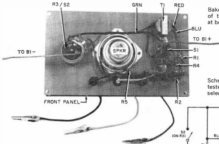
Bakelite front panel holds most of tester's parts. Three leads at bottom connect to transistor.
