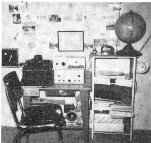
The listening post of Derrick Marston, WPE1DDY, Stamford, Conn. Derrick's receiver is a Heath AR-3, his antenna a 175' long-wire. Located above the AR-3 is a Heath QF-1 Q-multiplier and a preamplifier; a homemade "S"-meter is still in the construction stage. Derrick has accumulated 40 veries from 12 countries.
