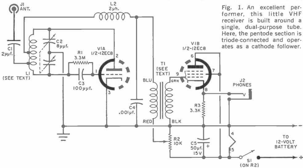
Fig. 1. An excellent performer, this little VHF receiver is built around a single, dual-purpose tube. Here, the pentode section is triode-connected and operates as a cathode follower.
