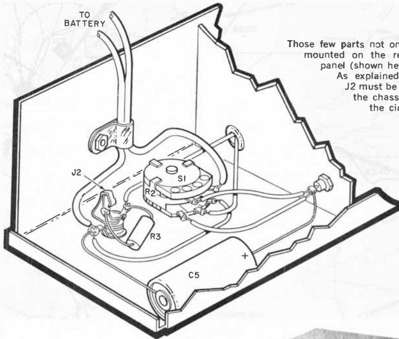
Those few parts not on the shelf are mounted on the receiver's front panel (shown here face down). As explained in text, jack J2 must be insulated from the chassis if you build the circuit in Fig. 2.
