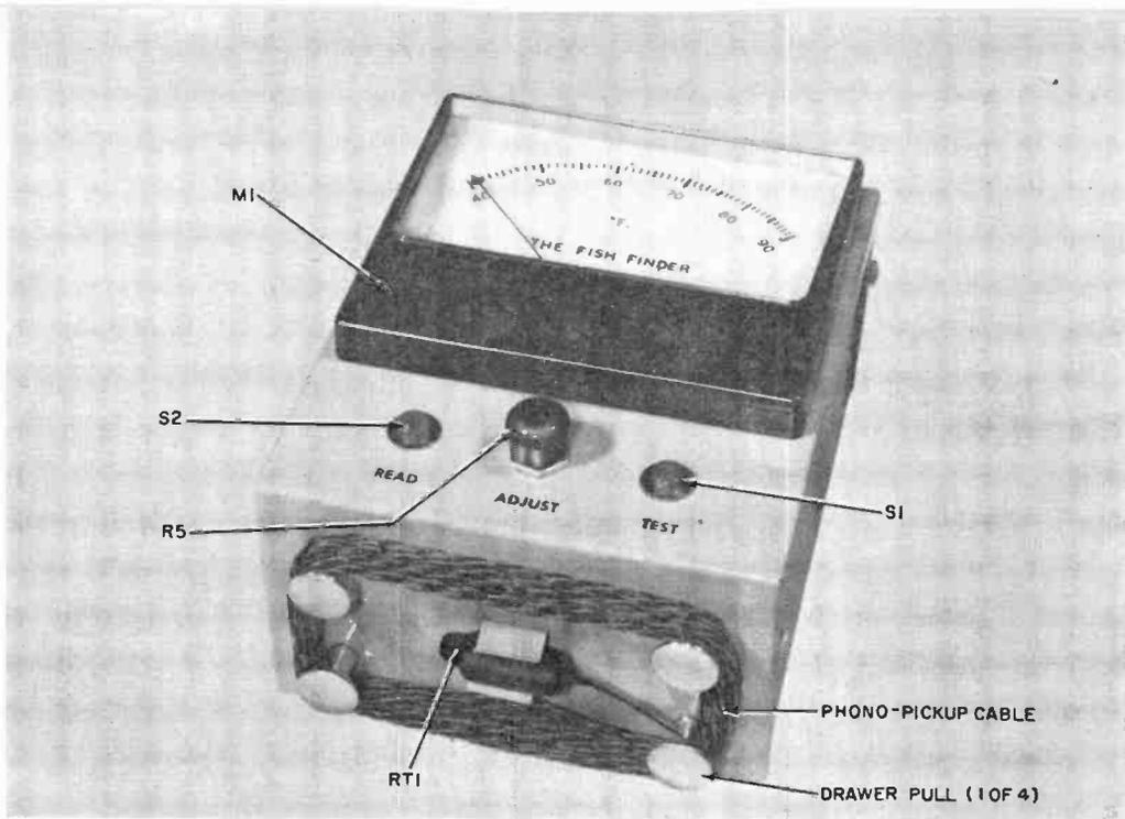
Completed "Fish Finder" is neat, attractive, and professional-looking. For protection against corrosion, apply a couple of coats of paint to box before mounting components.
