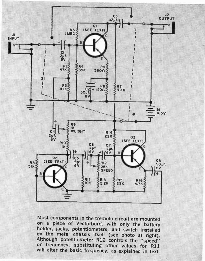
Most components in the tremolo circuit are mounted on a piece of Vectorbord, with only the battery holder, jacks, potentiometers, and switch installed on the metal chassis itself (see photo at right). Although potentiometer R12 controls the "speed" or frequency, substituting other values for R11 will alter the basic frequency, as explained in text.
