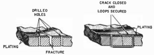
With one or two loops of fine wire and some cement, it's easy to repair cracked printed-circuit boards.
