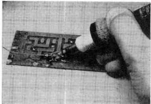
**SOLDERING.** Pass the leads from the new component through the loops, then solder them in place.
