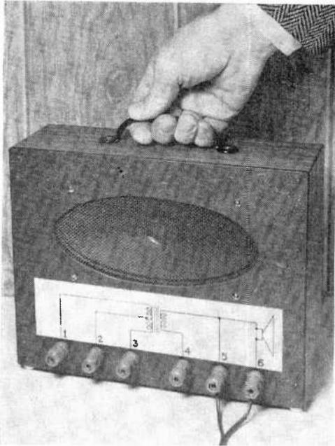
Designed for the serviceman, this Test Bench Squawk Box supplies for chassis under repair the missing audio circuit elements left behind in the customer's house.
