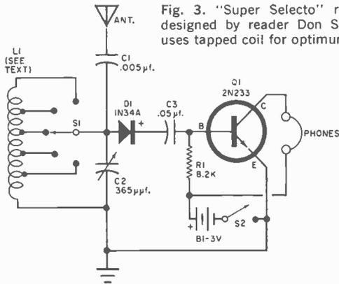
Fig. 3. "Super Selecto" receiver designed by reader Don Stovicek uses tapped coil for optimum "Q."
