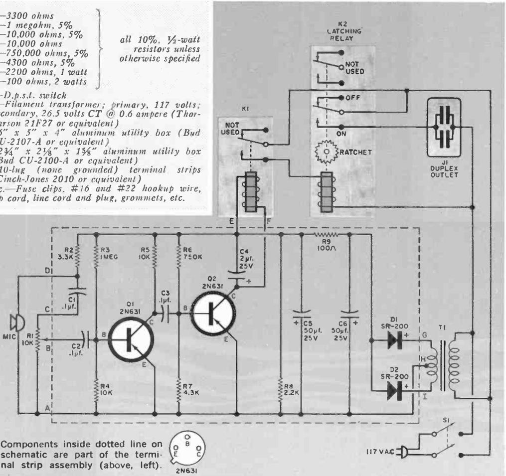
Components inside dotted line on schematic are part of the terminal strip assembly (above, left).
