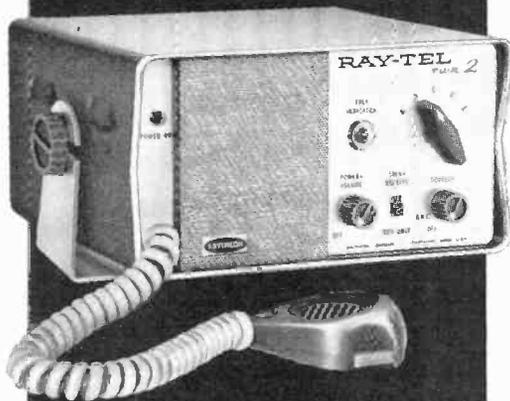
Other features — five transmit and receive channels with crystals ground to military specs; trim tabs for on-the-nose frequency control. Series noise limiter, adjustable squelch, pi-network output, automatic volume control, noise-free stand-by. 110 and 12 or 6 volt power supply. Plated chassis, heavy metal case, clamped tubes to withstand rough usage. Hand wired, no printed circuits, no re-ays.
