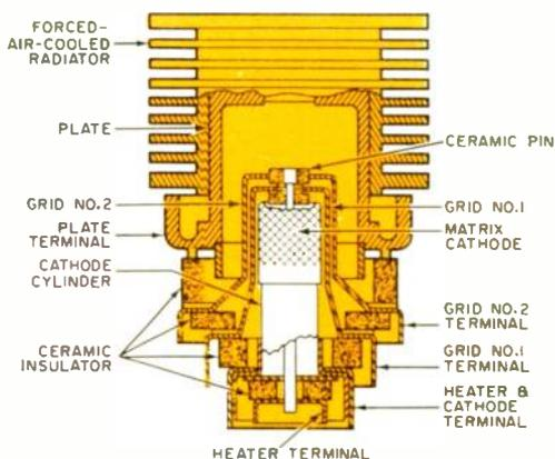
The light-house design raises the upper frequency limit for conventional negative-grid vacuum-tube amplifiers.
