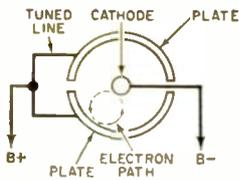
Magnetron operation depends upon interaction between the electron stream and a strong, constant magnetic field.
