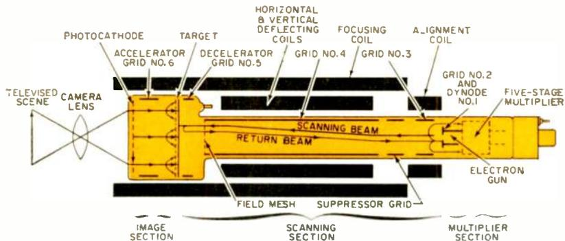
The image orthicon is one of the most complex, precise vacuum tubes in common use.
