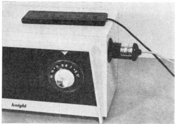
Two types of pickups are shown above. To couple to a radio, simply place a pickup in the strong inductive field of the speaker or the audio output transformer.
