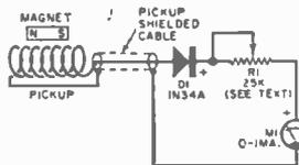
A circuit for reading relative rpm is shown at the left. A signal is picked up from rotating magnets on the engine or the motor.
