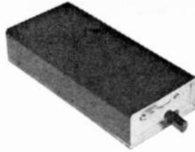
For mobile use; converts CB band to AM auto radio band (840-1100 kc.); self-contained mercury battery power supply; uses auto radio antenna.
