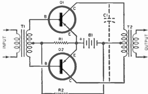
Fig. 4. Typical push-pull amplifier stage.
