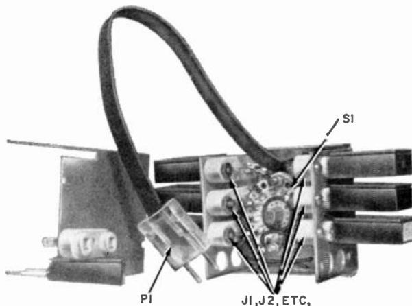
transmitter crystal to get out from under a strong interfering signal, or to move closer in frequency to a station he wishes to work. Unfortunately, even when the crystal socket is mounted on the transmitter front panel, it is not always easy to change crystals in a hurry, and when the crystal socket is recessed inside the transmitter, it is practically impossible. But by adding crystal switching to your transmitter, you can change crystals effortlessly.
