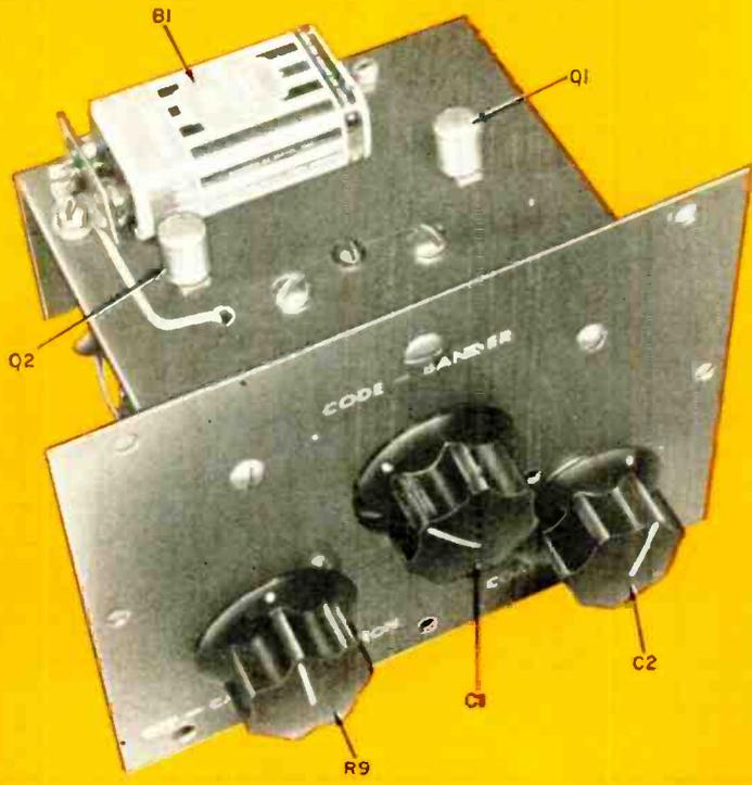
This top and front view of the Code Bander shows the general mechanical arrangement with the small chassis mounted to the front panel. Note that the transistors and battery are mounted on top of the chassis.
