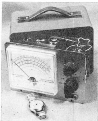
built in the POPULAR ELECTRONICS lab was assembled in 5¼ hours while 45 minutes were spent in calibration. Its accuracy was comparable to a factory-wired VTVM selling at the kit price.
