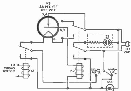
circuit causes constant recycling of K2 and K3 with the switch in manual position.
