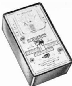
battery supply; can be used as crystal-controlled signal generator with tone modulation; built-in loop will detect r.f. fields near base of antenna; cable connections permit use as remote r.f. indicator; may also be used to check modulation; plate current, etc.
