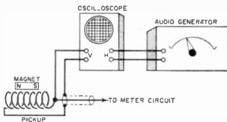
A pickup tachometer can be calibrated with an oscilloscope and audio generator. With a bit of work, a meter scale can be drawn which shows actual rpm.
