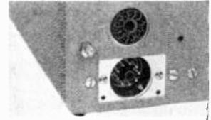
ACCESSORY SOCKET on rear panel (above power cord receptacle) for instant attachment of "Tone Alert".
