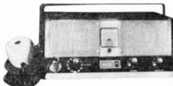
12-channel, crystal-controlled transmit and receive; universal power supply (117- and 12-volt); 10-tube performance superhet (1 r.f. stage and 1 455-kc. i.f. stage); noise limiter, adjustable squelch; ceramic mike; pi-network output; S-meter; 12 x 7 x 5 $\frac{3}{4}$ ; 15 lb.
