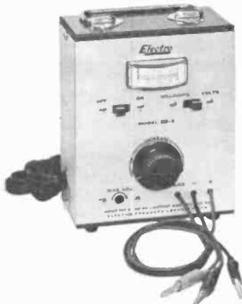
meter and can supply 0-20 volts of well filtered d.c. at currents of up to 150 ma. (or 24 volts at 100 ma.). The output voltage is continuously adjustable over its range. In addition, a separate adjustable bias output of from 0 to 6 volts is available. Model EC-3 is supplied with pre-attached clip leads.
