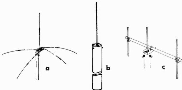
The ground plane (A) is probably the most common CB base station antenna. Consisting of a vertical radiator and four horizontal elements, it is easy to assemble and requires no tuning adjustments. A coaxial antenna (B) is also easy to assemble and has the advantage of not requiring the horizontal elements of a ground plane. The 3-element beam (C) is directional; unless you want to work only in one direction, it must be rotated.
