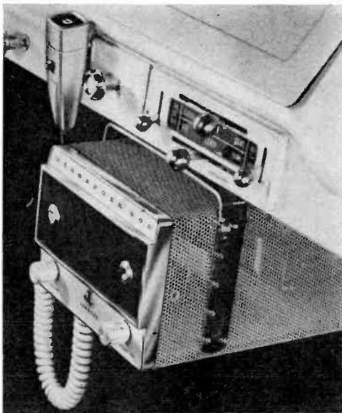
Some CB equipment manufacturers are also producing transceivers for the Business Radio Service. This is the E.F. Johnson “Viking 202,” suitable for BRS use between 25 and 50 mc. Sold for about \$200.00, it consists of a 10-tube AM circuit.
