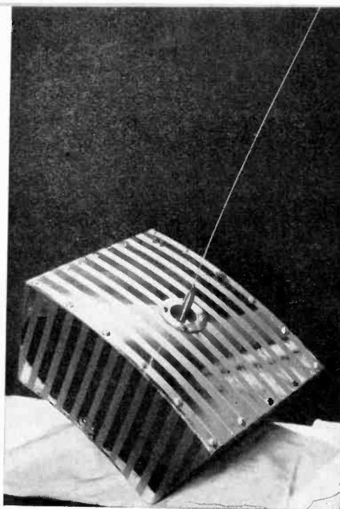
This is “OSCAR II,” the second satellite built by radio amateurs and launched by the U. S. Air Force (in conjunction with its “Discoverer” program). The 2-meter ham-band signals of the “OSCAR II” were heard by hundreds of listeners. The black-and-silver striping makes for better thermal control while the satellite is in space.
