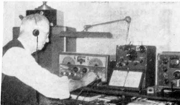
Most DX'ers use a pair of earphones to dig for that rare station down in the noise. Grady C. Ferguson, Charlotte, N.C., is no exception as he tunes his Hallicrafters SX-100 receiver. To the right of this receiver is a war surplus BC-221 frequency meter used to calibrate the receiver tuning dial and measure the frequency of new DX catches. Also on the right is a pre-World War II short-wave receiver, the Hallicrafters SX-28.
