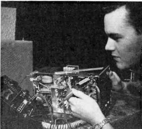
Both American and Canadian operators must have their transmitting equipment serviced by a properly licensed technician. Modest tuning adjustments by a CB'er are permitted, but under no circumstances should a transmitter's crystal oscillator be tampered with. CB'ers can be fined by the FCC for off-frequency operation and other offenses.
