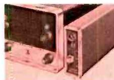
Plugs into the "Messenger Two"—easily attached to "Messenger" or other CB transceivers! Mutes speakers on your units until one calls another—then automatically, your stations hear audio note and indicator light flashes "on", remaining lighted until call is answered.
