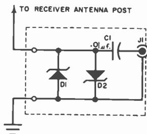
Muter mounts neatly to receiver terminals as shown in top photo. Author attached a piece of insulating material to *J1* (photo at left) and used it to hold *C1*, *D1*, and *D2*. Connection to receiver antenna is brought out through grommet in top of can.
