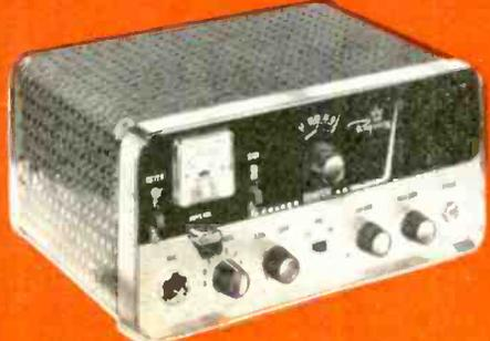
Here's where big savings are yours. Now with the Regency Romper, one crystal does the job of two—it both transmits and receives—reducing your crystal cost by one-half. No coil tuning is required—just plug in the crystals. Switch provides for variable tuned reception of all 23 channels or crystal-controlled operation.
