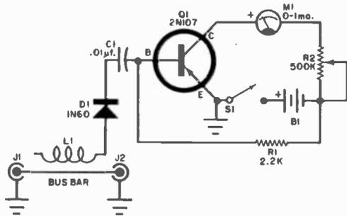
Fig. 2. The transmitter tune-up meter circuit submitted by reader William Halleron can be connected "in-line" between any low- or medium-power transmitter and antenna.
