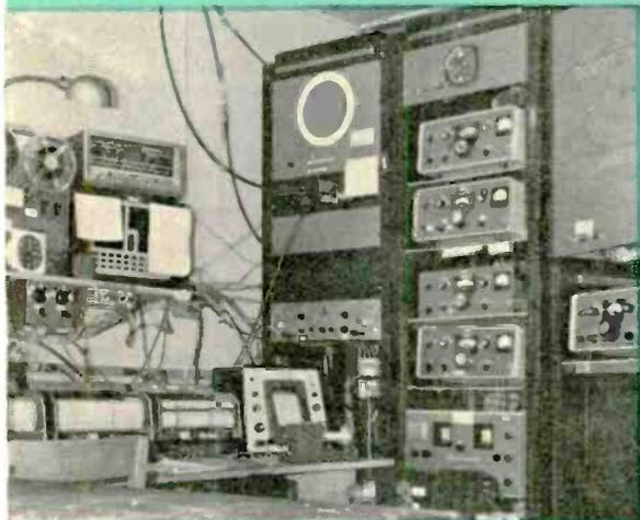
Collins and Hammarlund gear above—enough to delight any DX'er—is connected to antennas at left for monitoring Jupiter's emissions from 5 to 30 mc.; Hallicrafters unit monitors WWV. Other equipment shown: three paper recorders and a tape machine, all used to record Jupiter's signals for study.
