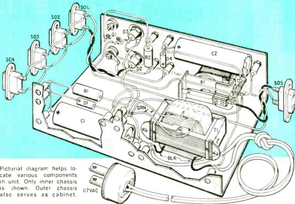
Pictorial diagram helps locate various components in unit. Only inner chassis is shown. Outer chassis also serves as cabinet.
