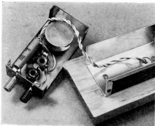
Keep all wiring as short and direct as possible, with all connections well insulated from the metal chassis and from each other. Wires to lamp sockets go under board.
