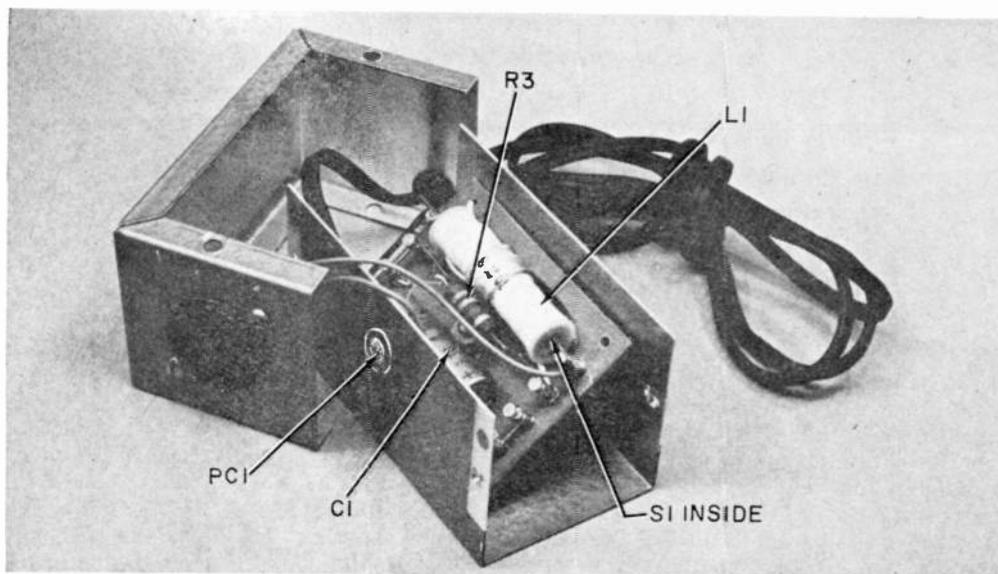
Parts location of author's "Nite Light" is shown above. Mounting board sets at angle.
