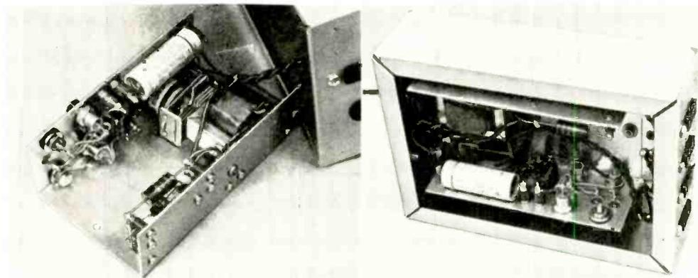
After wiring, subchassis (above, left) is installed in larger chassis and fastened in place.
