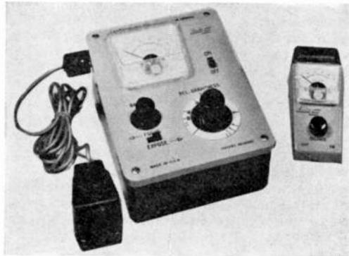
Fig. 1. The diagram shows the basic design of LogEtronics' "Focatron" electronic focusing meter for photographic use. Two models are available: a professional/industrial unit (at left, above), and a moderately priced semi-pro/advanced amateur unit (right).
