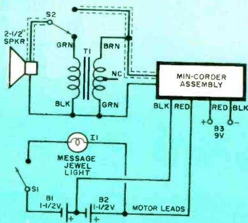
Loudspeaker also serves as a microphone. Diagram shows few parts needed.
