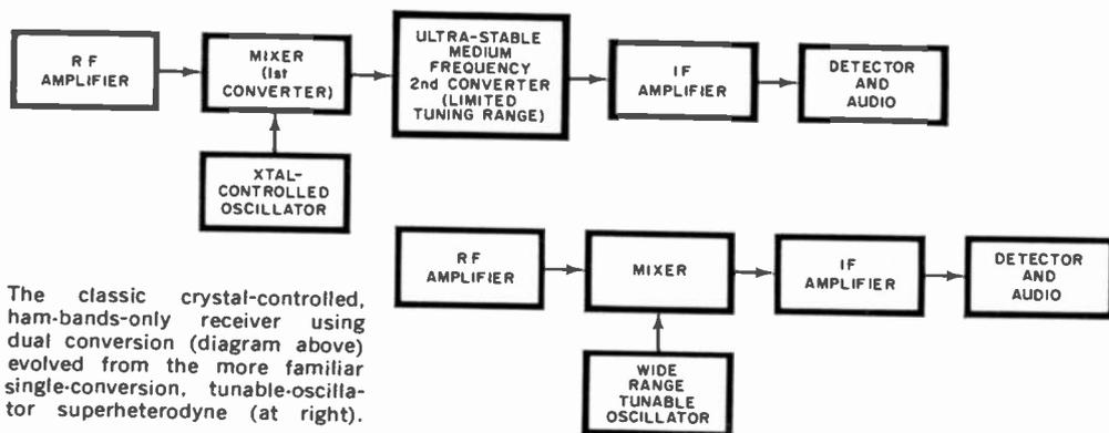
The classic crystal-controlled, ham-bands-only receiver using dual conversion (diagram above) evolved from the more familiar single-conversion, tunable-oscillator superheterodyne (at right).
