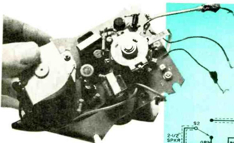
The Min-Corder comes assembled and ready to be put into the cabinet. It uses a continuous loop of tape with oxide on both sides.
