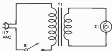
Simple circuit above is easily wired. Solder all connections and use tape or wire nuts over *T1*'s wires to insulate them.
