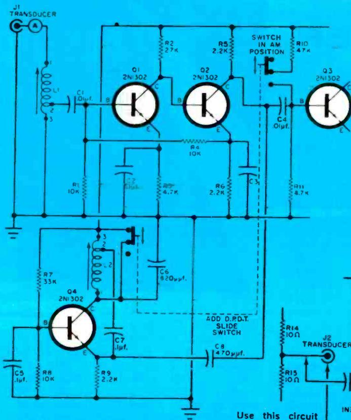
For better AM reception with the "Ultrasonic Sniffer," modify the circuit by adding a single d.p.d.t. slide switch as shown here.
