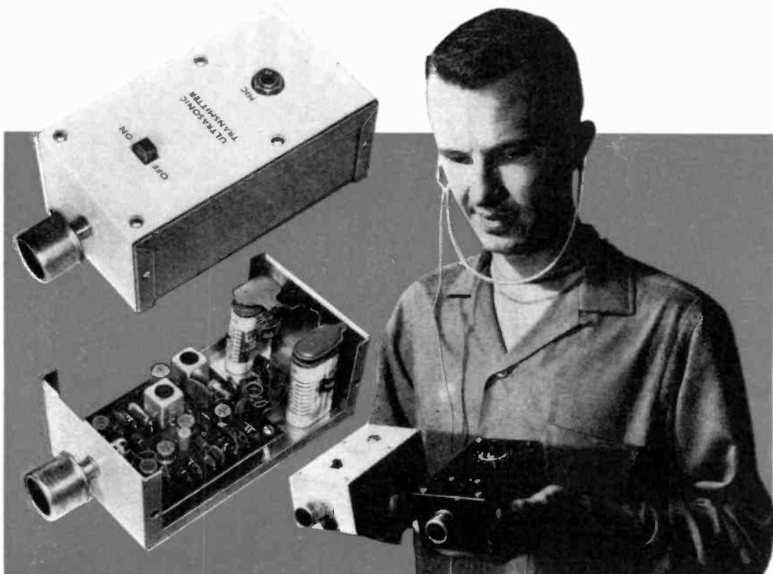
The ultrasonic transmitter is mounted in the same case as the Sniffer. The board is held by spacers and the batteries are clamped to the rear wall with spring clips.
