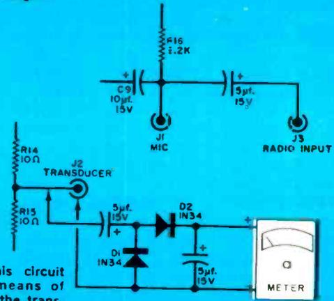
Use this circuit as a means of tuning the transmitter to 38 kc.
