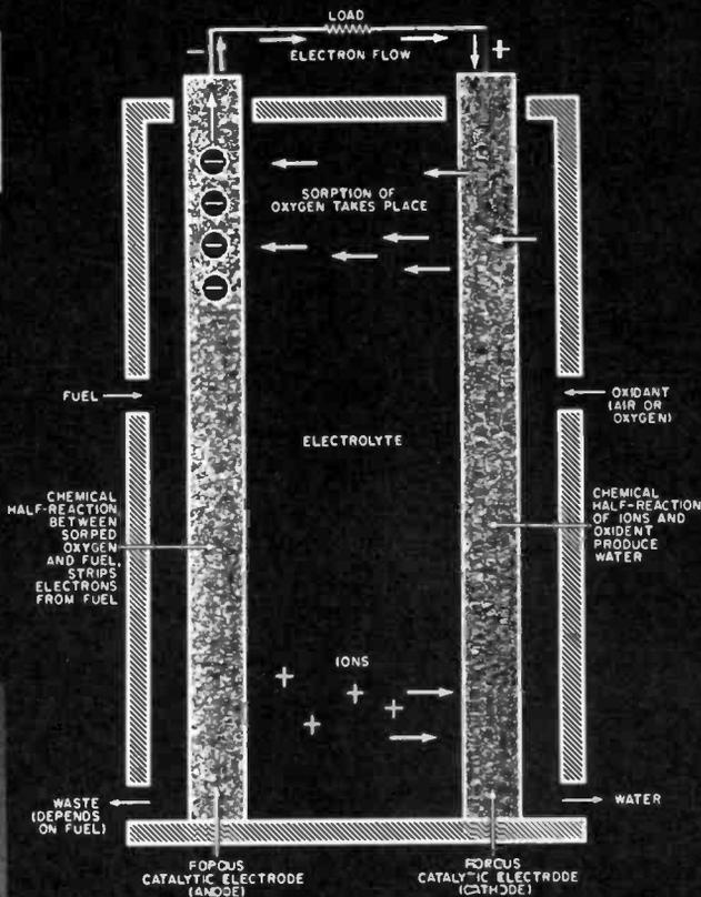
This generalized drawing shows basics of fuel cell operation. The electrolyte may be liquid, semiliquid, or solid; the electrodes can be carbon, plastic, platinum or nickel boride, typically in combination. Fuel depends largely on the type of electrode used; hydrogen reacts very easily, but inexpensive hydrocarbons are now being used thanks to improvements in cell electrodes.
