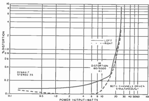
Intermodulation distortion as measured by the Hirsch-Houck Laboratories was below 0.5% for all output levels up to 17.18 watts output per channel.
