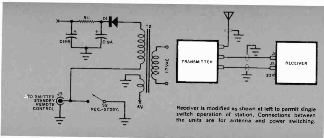
Receiver is modified as shown at left to permit single switch operation of station. Connections between the units are for antenna and power switching.
