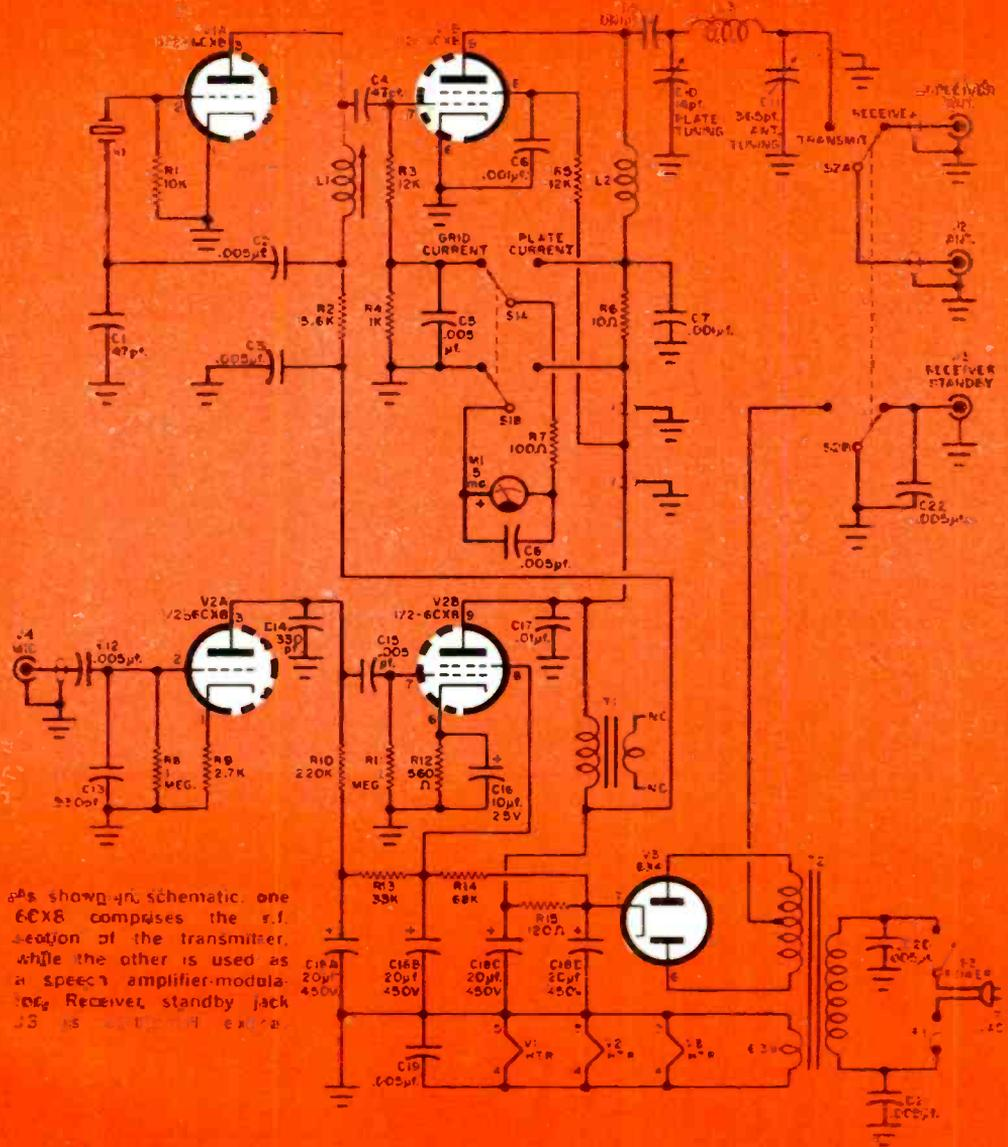
Fig. 1 shows schematic. One 6CX8 composes the r.f. section of the transmitter, while the other is used as a speech amplifier-modulator. Receiver, standby jack JS as shown in schematic.
