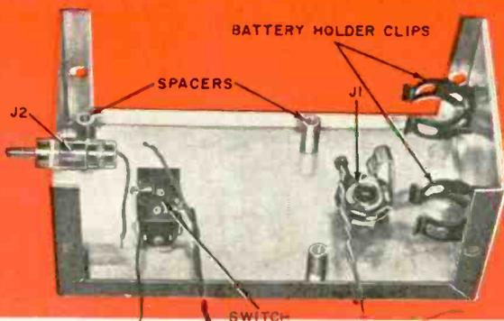
Prewire the jacks, switch, and battery clips before mounting the printed circuit board. Use metal spacers to hold the board over the on-off slide switch.
