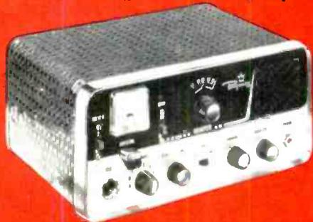
Here's where big savings are yours. Now with the Regency Romper, one crystal does the job of two—it both transmits and receives—reducing your crystal cost by one-half. No coil tuning is required—just plug in the crystals. Switch provide for variable tuned reception of all 23 channels or crystal-controlled operation.
