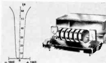
With CB channels only 10 Kc apart, selectivity is important! In the HB-500, ultra-sharp selectivity is achieved by means of a true mechanical bandpass filter in the 455 Kc IF section. At 10 Kc on either side of the center frequency, the filter provides 60 db of attenuation—an extremely high rejection ratio that assures complete adjacent channel rejection!
