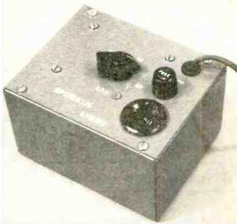
**Construction.** A prerequisite in building your "Spookin' Light" is to be absolutely sure that none of the components is in electrical contact with the aluminum box. A 1:1 isolation transformer would make this device safer, but if reasonable care is exercised in construction, the "Spookin' Light" will not present a shock hazard.
