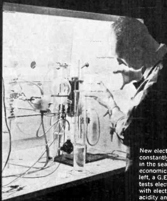
New electrode materials are constantly being evaluated in the search for reliable, economical fuel cells. At left, a G.E. researcher tests electrode material with electrolytes of varying acidity and alkalinity.
