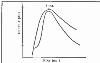
The steep curve represents low frequency sensitivity (measured in db.) at varying bias levels for many tapes. Note that you get good performance providing you have a
