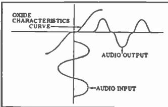
The slightly twisting curve at the upper left represents the oxide response. The lower curve is a pure, sine wave input. At the upper right we have the result of the response curve on the input . . . a mess.
