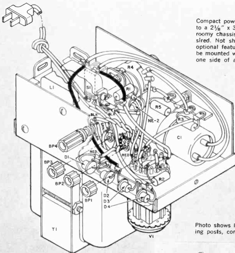
Compact power supply is built into a  $2\frac{1}{8}$ " x 3" x  $5\frac{1}{4}$ " box; more roomy chassis can be used if desired. Not shown is fuse F1, an optional feature. Fuse holder can be mounted where space permits, one side of a.c. line wired to it.
