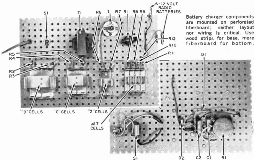
Battery charger components are mounted on perforated fiberboard; neither layout nor wiring is critical. Use wood strips for base, more fiberboard for bottom.
