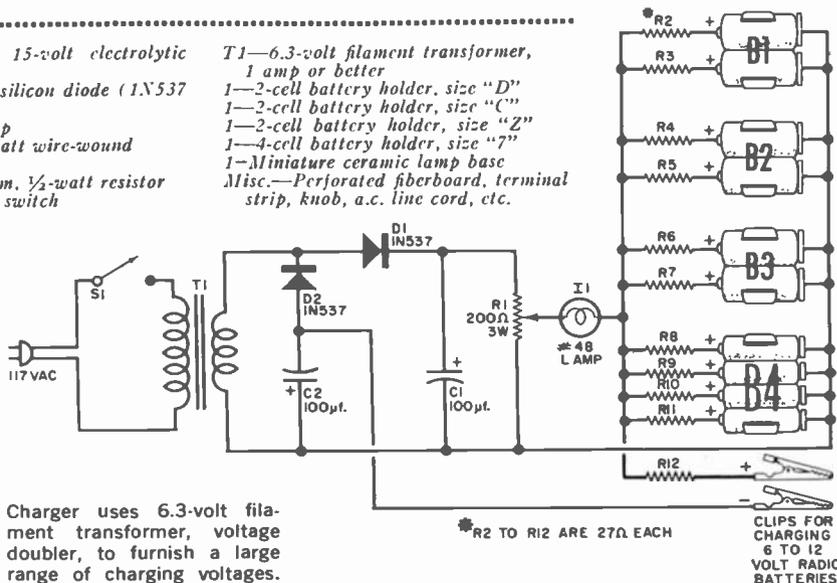
Charger uses 6.3-volt filament transformer, voltage doubler, to furnish a large range of charging voltages.
