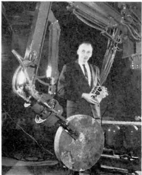
**SEA ARM**—An electronically controlled "robot," designed to pick up 500-lb. objects from the ocean floor, was recently attached to the Navy bathyscaphe Trieste. Electronics were designed by ACF Industries.
