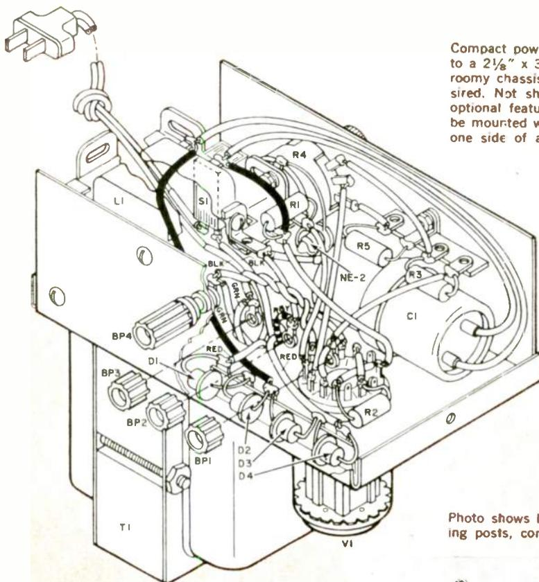
Compact power supply is built into a 2½" x 3" x 5¼" box; more roomy chassis can be used if desired. Not shown is fuse F1, an optional feature. Fuse holder can be mounted where space permits, one side of a.c. line wired to it.
