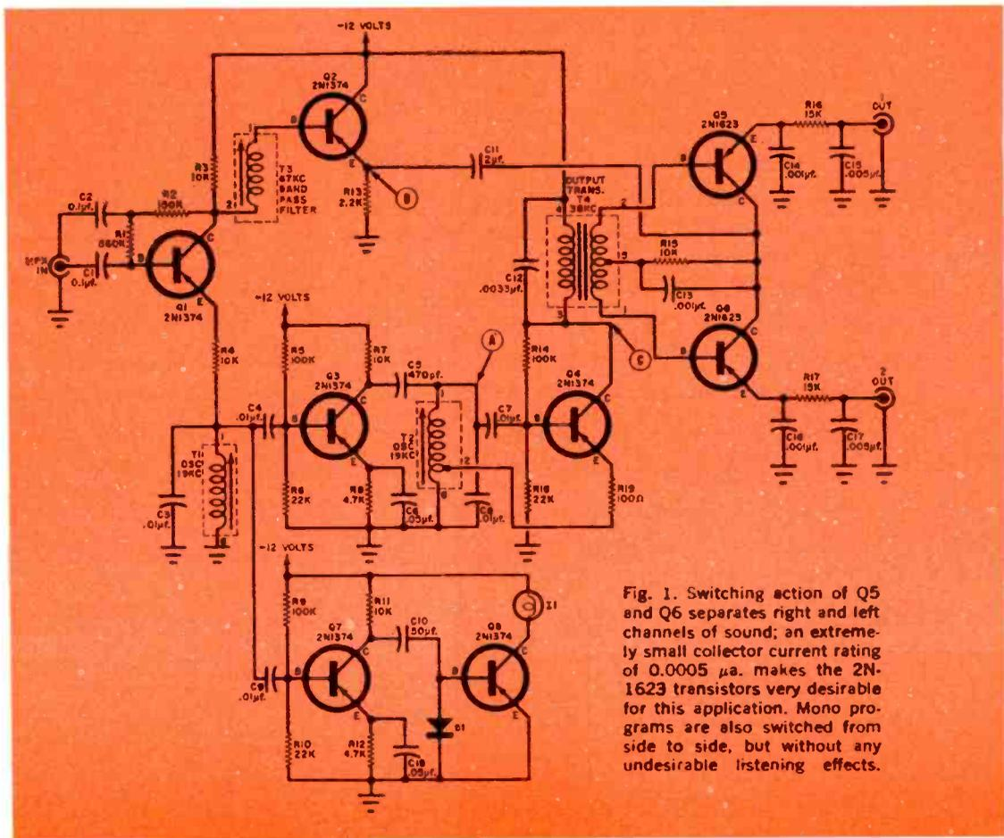
Fig. 1. Switching action of Q5 and Q6 separates right and left channels of sound; an extremely small collector current rating of 0.0005  $\mu$ a. makes the 2N-1623 transistors very desirable for this application. Mono programs are also switched from side to side, but without any undesirable listening effects.
