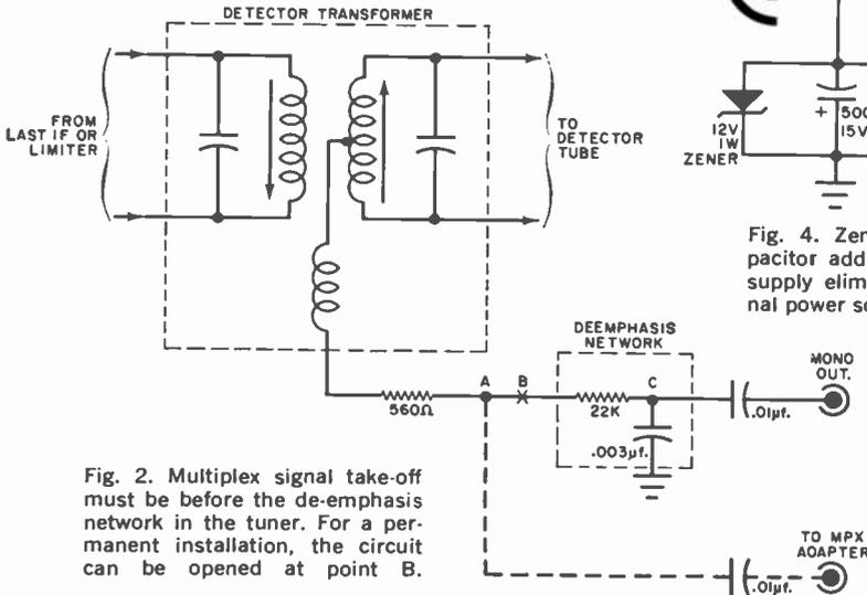
Fig. 2. Multiplex signal take-off must be before the de-emphasis network in the tuner. For a permanent installation, the circuit can be opened at point B.
