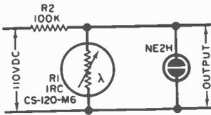
Simple oscillator can be powered by a bench supply delivering 110 volts d.c.; R2 is rated at  $\frac{1}{2}$  watt.
