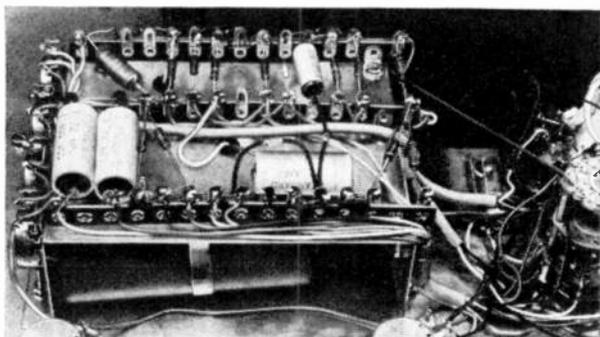
der cars and has two ranges—0-1200 rpm and 0-6000 rpm. Both ranges work from a transistorized Schmidt trigger pulse counter and can be attached to conventional and most transistorized ignition systems.
