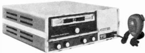
mitted frequency tolerance of  $\pm 0.003$ —well below the 0.005 required by the FCC. Other features include a low-noise nuvistor front end, a dustproof enclosed plug-in relay, and a pi-network with a two-stage TVI filter. The Guardian 23 utilizes a transistorized universal type power supply (12 volts d.c. or 117 volts a.c.), and the receiver is a dual-conversion superhet. Price, \$299.50.
