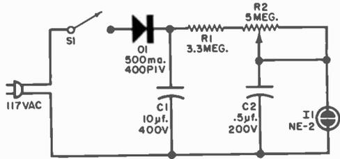
Flash rate of neon relaxation oscillator is determined by time constant of *R1*, *R2*, and capacitor *C2*.
