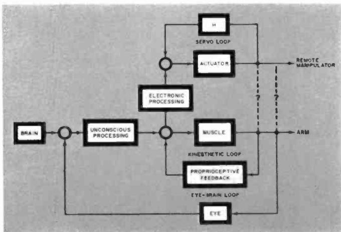
Use of electromyographic signals for control purposes was the purpose of a recent study undertaken by Philco's Bio Technology Laboratory. Block diagram shows how man and remote machine might be linked together.
