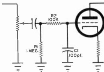
this type of interference is to reduce the value of the grid resistor (R1) in the first audio stage to 1 megohm, and install R2 and C1.
