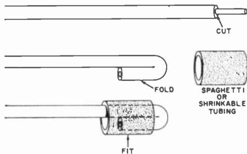
itself for a convenient but small distance. Although about 1/2" is usually enough, different thicknesses or stiffnesses of wire will require different size folds to make a neat finish. (Be careful to avoid accidental contact with metallic shielding when present.) Then slip a piece of spaghetti over the fold as shown in the drawing—it should fit snugly.
