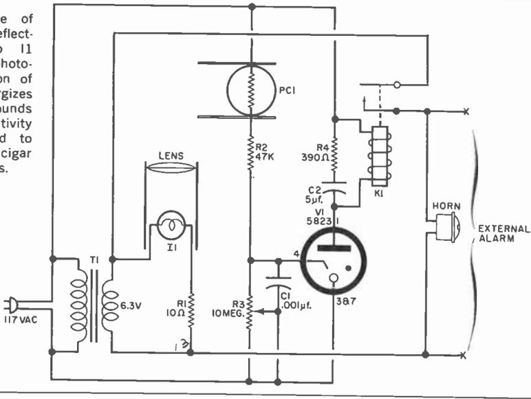
on the ceiling and build down. A room almost filled with smoke may have an area close to the floor that will allow a safe crawl space for escape. By the same token, if a smoke alarm were located near the ceiling, it would sound an alert long before a dangerous concentration of smoke accumulated. Here's a smoke detector you can construct complete with a built-in alarm for about \$10.00.
