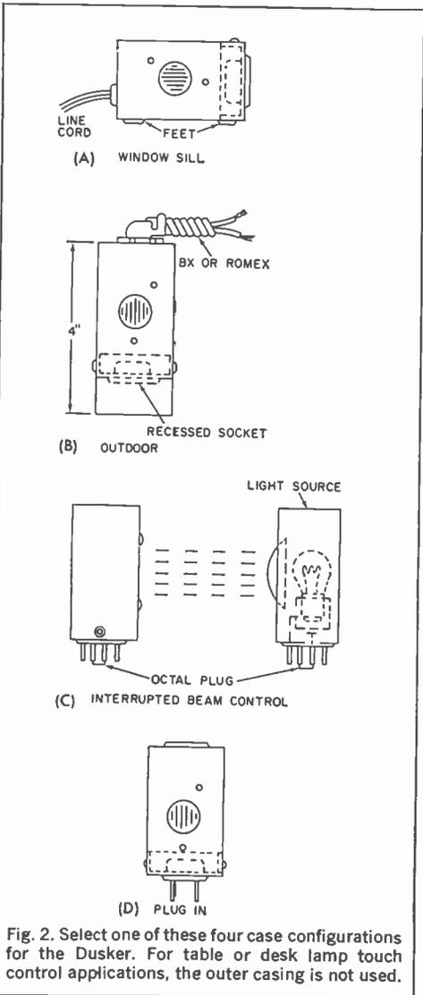
Fig. 2. Select one of these four case configurations for the Dusker. For table or desk lamp touch control applications, the outer casing is not used.
