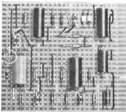
Fig. 9. Novel "Veroboard" has bonded copper strips pierced with a regular matrix of holes. Components leads are soldered directly to the strips.
