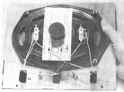
The input jacks on either side of S2 can be eliminated by connecting the test leads directly. Before mounting, check voice coil phase and wiring details.
