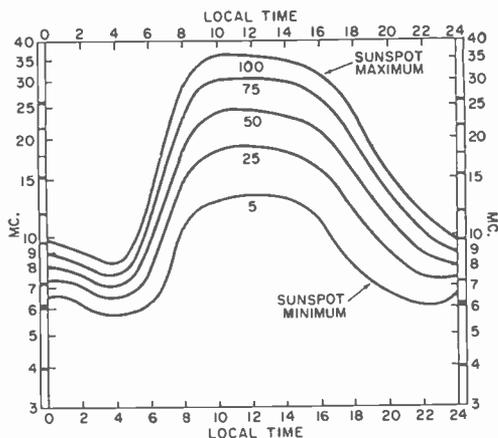
Maximum usable frequencies that the ionosphere will reflect in the fall in North America over a distance of 1200 miles during periods of high and low sunspot activity. Black bars along the frequency scale indicate the international broadcasting bands.
