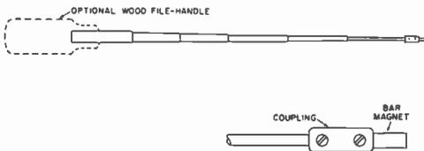
remaining antenna and a handle at the other end. The telescoping sections of the antenna enable you to extend your reach as needed. The magnet can be secured with a control-shaft coupler, string, or tape.
