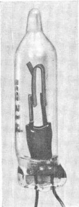
off can be realized, making the breaker quite suitable for temporary displays or exhibits. The short life, in this instance, is more than offset by the very low cost for the high current-handling capability.
