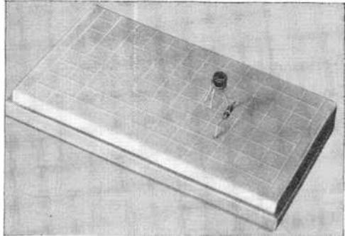
Fig. 14. Components are assembled on Vicon "Proto-Board" by inserting their leads into the soft material comprising the plastic base.
