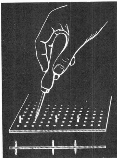
Fig. 4. These Vero connectors feature terminal pins with self-cutting serrations. A special tool is used to push pins down into the holes.
