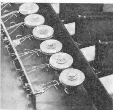
These heavy-duty springs are in the 13-note pedal bass manual. Builder assembles the contacts which are connected via a preassembled cable harness to the pedal keyer circuit board.
