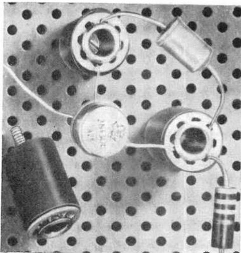
Fig. 7. Component leads are pressed into holes in top of ETA "Flexi-Klip" connectors.
