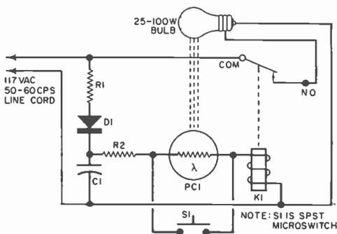
Fig. 7. This low-cost touch control circuit can easily be wired to any desk or table lamp by adding a microswitch across PCI. To turn on lamp, touch S1 gently. To turn off lamp, bring hand near PCI, shielding it from light. For proper operation, PCI must be shielded from other strong light sources.
