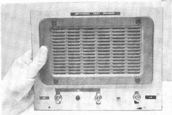
Install the speaker in any suitable enclosure, or wall-mount it behind a baffle. Simply flip the appropriate switches to obtain desired impedance.
