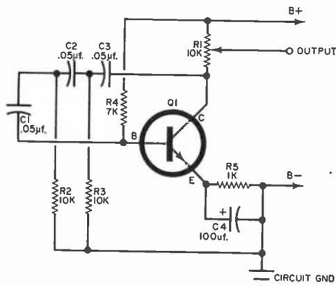
Fig 2 This phase shift audio oscillator modeled on Vari-L Develoboard closely approximates its circuit diagram layout.
