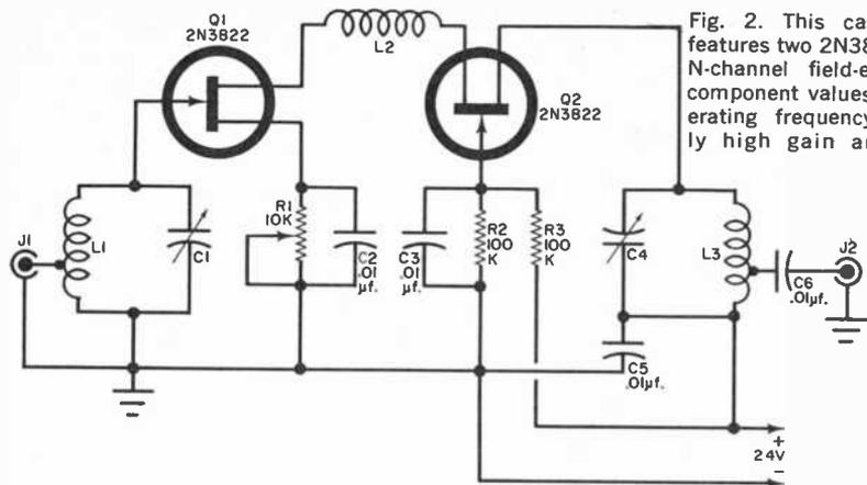
Fig. 2. This cascode amplifier circuit features two 2N3822 (Texas Instruments) N-channel field-effect transistors. With component values chosen for desired operating frequency, circuit has relatively high gain and low noise figure.
