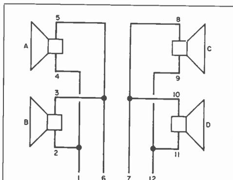
When speakers are in proper mechanical phase, they are not necessarily in proper electrical phase. One way to achieve optimum listening is to use a signal generator and phase the speakers in each enclosure and then phase the enclosures.
