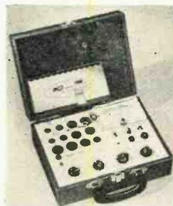
plished with the *B & K Model 606 "Dyna-Jet"* tube tester. It checks for shorts, grid emission (in a unique 100-megohm sensitive circuit), leakage, gas, and cathode emission under simulated load conditions for more accuracy. Each section of multi-section tubes is checked. The Model 606
