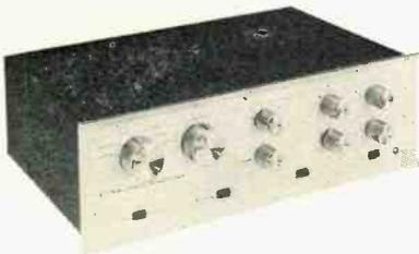
unit incorporate a tone control configuration which removes the phase and frequency controlling elements when the control is in the mechanical center of its rotation; advantages of both switch-type control and infinite resolution are claimed. Harmonic and IM distortion are guaranteed to be below 0.05% at 3 volts out in the range of 20 to 20,000 cycles, with up to 10 volts out at less than 0.15% distortion into as little as 10,000-ohm loads.
