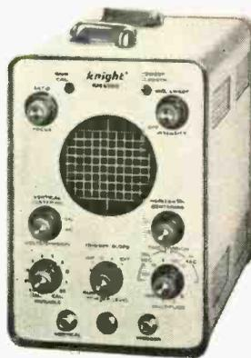
16 pounds. Identified as the Knight Model KN5005 scope, it boasts a flat frequency response within  $\pm 3$  db, from d.c. to 6 mc., and has a vertical sensitivity of 0.05 volt/division. Its horizontal circuit provides linear sweep from 1 microsecond/division to 50 microsecond/division,  $\pm 10\%$ , with a sweep as fast as 0.2 microsecond/division when its built-in multiplier is used.
