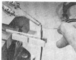
support two components or wires, two clothespins clamped back-to-back can be employed. If you don't want to use a vise to hold the clothespins, you can mount one or more pins on a small block of wood.—Robert E. Kelland
