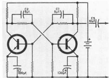
Oscillator, timing, and other tuned circuits, whose frequency of operation depend on controlled circuit values, call for stable low-loss units. In this regard, C2 and C3 are critical, whereas C1, C4, and C5 can vary considerably. Except for polarized types such as electrolytics, polarity is not a factor.
