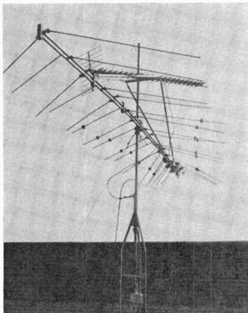
One of the important ingredients for topnotch tropo and E-skip DX is an antenna farm. The author used these high gain VHF and UHF rotatable antennas.
