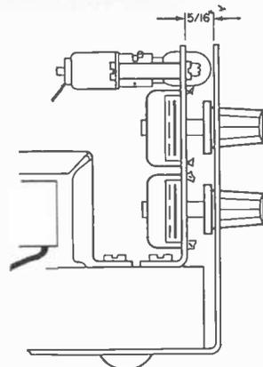
Fig. 7. Be sure to allow indicated spacing between aluminum bracket and instrument's front panel, to clear the pilot lamps.
