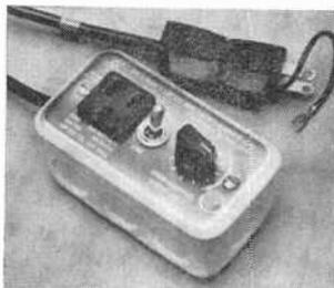
Mounted in a rugged, vinyl-coated, shock-resistant, steel, electrical "handy box," the SCR-1 controls the speed of universal type a.c./d.c. motors such as are found in many hand drills, Sanders, saws, stirrers, beat-
