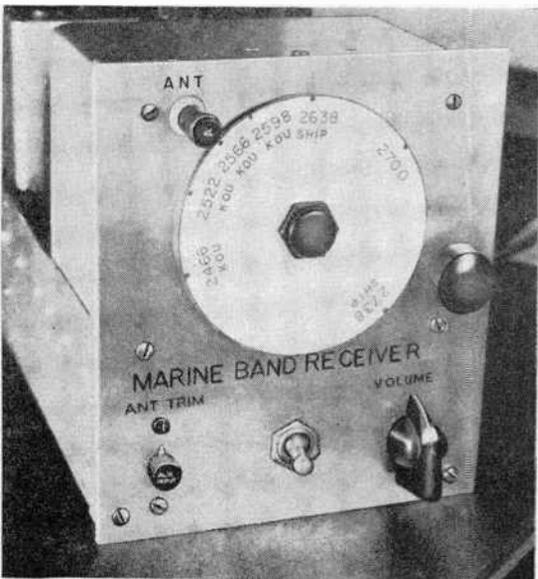
A dial was fabricated showing some of the more important maritime ship and shore frequencies used on the west coast. Listeners on the east coast should set their receivers so that WWV on 2.5 MHz is in the middle of the tuning range. The converted BC-454 makes an excellent "second" receiver for home use, or may be battery-operated in a small boat.
