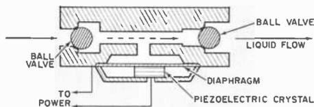
Fig. 3. The possibility of igniting flammable liquids is reduced by this motorless liquid pump assembly developed by Precision Chemical Pump Corp.
