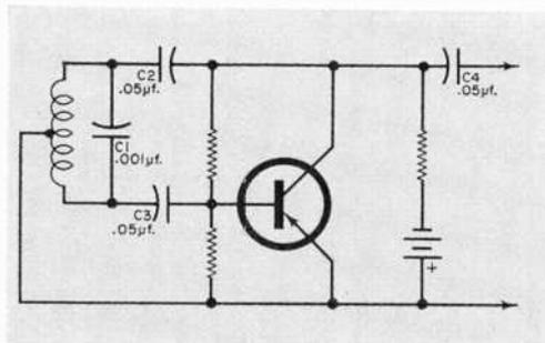
Value of C1 is critical here—both capacitor and coil determine the frequency of this Hartley oscillator. Capacitors C2 and C3 merely serve as d.c. blockers and should be high enough to offer very little impedance at the operating frequency. As with most coupling capacitors, C4 blocks d.c. and should be large enough to easily pass the signal.
