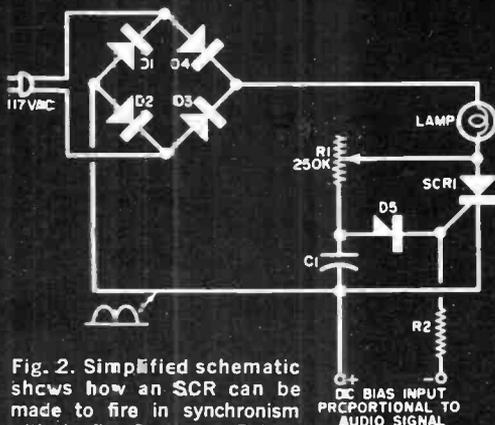
Fig. 2. Simplified schematic shows how an SCR can be made to fire in synchronism with the line frequency. Pulsating c.c. acts as trigger pulses.
