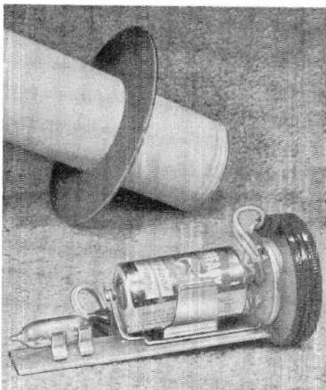
The author used a metal strap attached to the horn and battery holder to mount the mercury switch. The cardboard ring, which permits the alarm to roll, is simply press-fitted to the tubular container.
