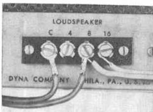
In this situation both speakers have the same impedance; the extra speaker is simply connected across the 8-16 ohms output taps.
