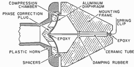
Fig. 2. Motorola's new loudspeaker driver employs the movement of a ceramic tube to drive an aluminum diaphragm, thus eliminating the voice coil.
