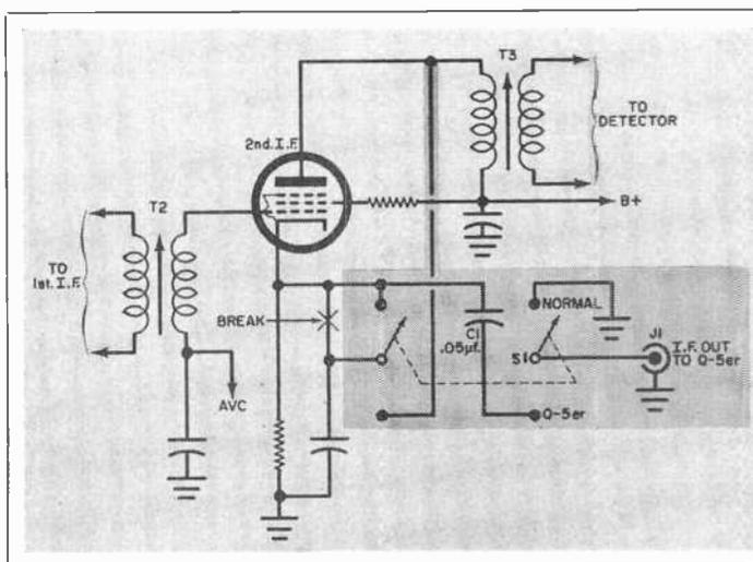
In the "Normal" position, the receiver operates as originally designed. In the "Q5-er" position, the output of the i.f. stage is bypassed to ground and the 455-kHz i.f. signal fed into the connection to the Q5-er.
