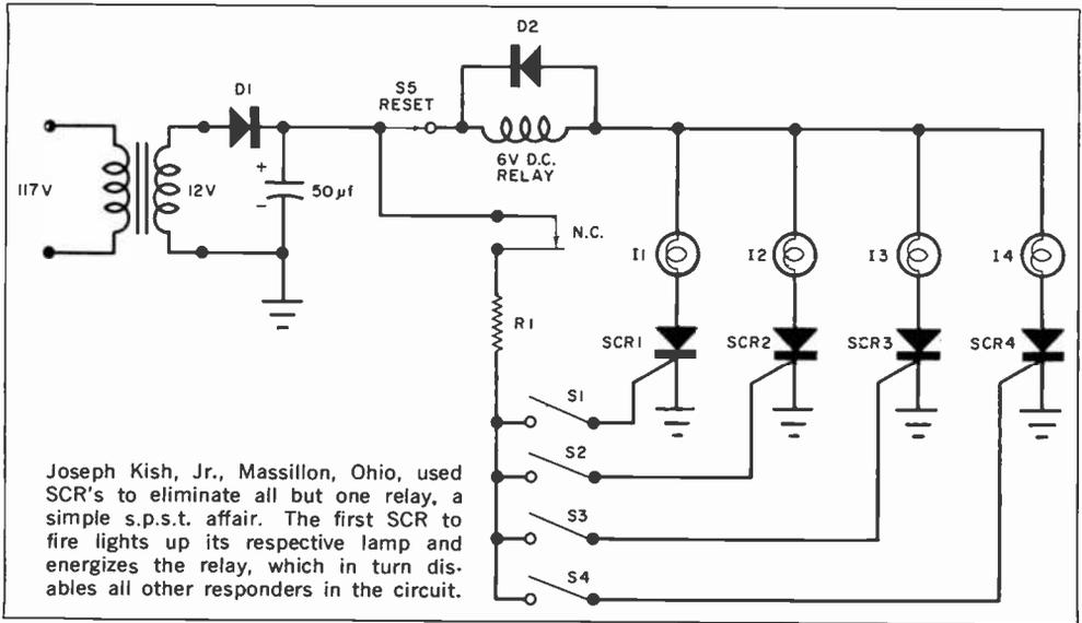
**Silicon Controlled Rectifiers.** Joseph Kish, Jr., of Massillon, Ohio, used silicon controlled rectifiers (SCR's) to replace the relays. The player who closes his switch first sends a pulse to the related SCR, triggers it into conduction, and causes the lamp to light. When this happens, the single relay energizes, and "disarms" the other players' switches.
