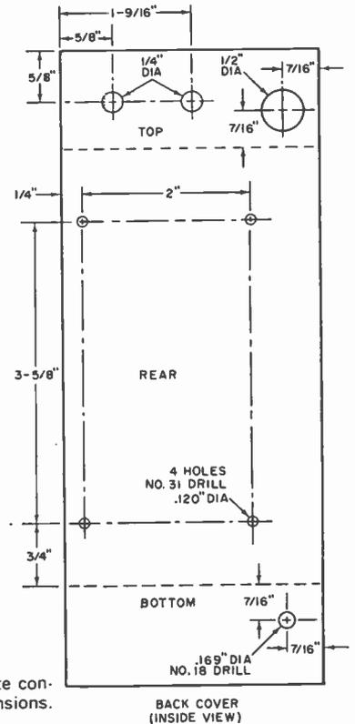
If you purchase an LMB aluminum box No. 139, you can duplicate construction of the receiver shown on the cover using these dimensions.
