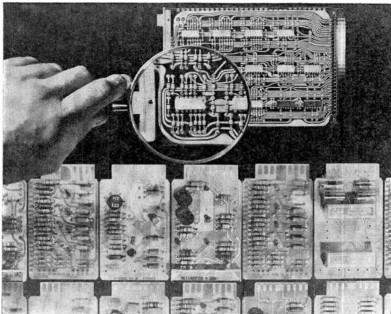
Monolithic integrated circuits, such as the one shown magnified above, are used in Sperry Rand's new UNIVAC 9000 series data processing systems. They perform the same functions as the large conventional printed circuit boards. One chip is the equivalent of 14 conventional printed circuit boards like the ones shown in the lower area of the photo.
