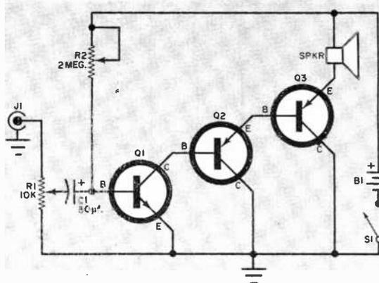
Fig. 1. Audio amplifier featuring input transistor *Q1* direct-coupled to Darlington pair *Q2-Q3*. Overall gain is product of the betas of the transistors.
