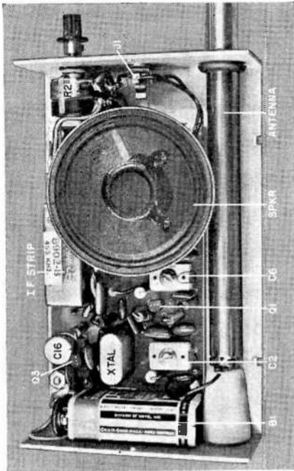
symmetry configuration. A 100-ohm speaker is fed from the audio output stage through closed-circuit phone jack *J1*. When headphones are plugged into the phone jack, the speaker is automatically disabled. Any impedance headphone can be used. The audio output stage delivers over 50 milliwatts of power.
