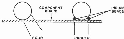
have wound up soldering the capacitor in an ungainly position, giving your project a "biased" appearance. To insure correct posture of the component, and an overall improvement in the project, slip a small-sized Indian bead onto each lead of the capacitor before soldering it.
