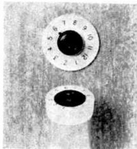
to take your next pill can also be used as shaft position indicators on your electronic projects. To make such an indicator, remove the pointer disc from the lid and drill a  $\frac{3}{16}$ "-diameter hole in the center of the cap. Then slice off the dial portion of the cap, using a sharp knife or razor blade. Slip the dial onto the potentiometer shaft and secure it in place with a nut. Now replace the indicator knob on the dial.
