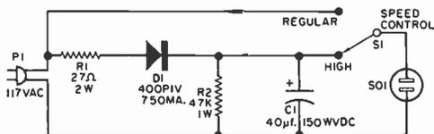
You can house this handy electric shaver adapter in a small metal box using an Amphenol 61-M-1 a.c. plug at *P1* and a chassis receptacle at socket *SO1*. Float all of the wiring, and make certain that none of the components accidentally shorts to the box.
