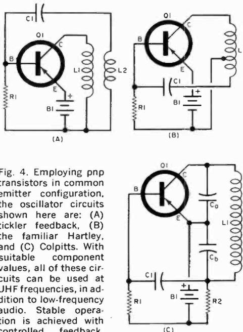
Fig. 4. Employing pnp transistors in common emitter configuration, the oscillator circuits shown here are: (A) tickler feedback, (B) the familiar Hartley, and (C) Colpitts. With suitable component values, all of these circuits can be used at UHF frequencies, in addition to low-frequency audio. Stable operation is achieved with controlled feedback.
