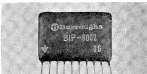
Similar in appearance to a packaged electronic circuit, this Burroughs' IC package features rugged dependability, making its use in electronic equipment subject to shock and vibration most desirable.
