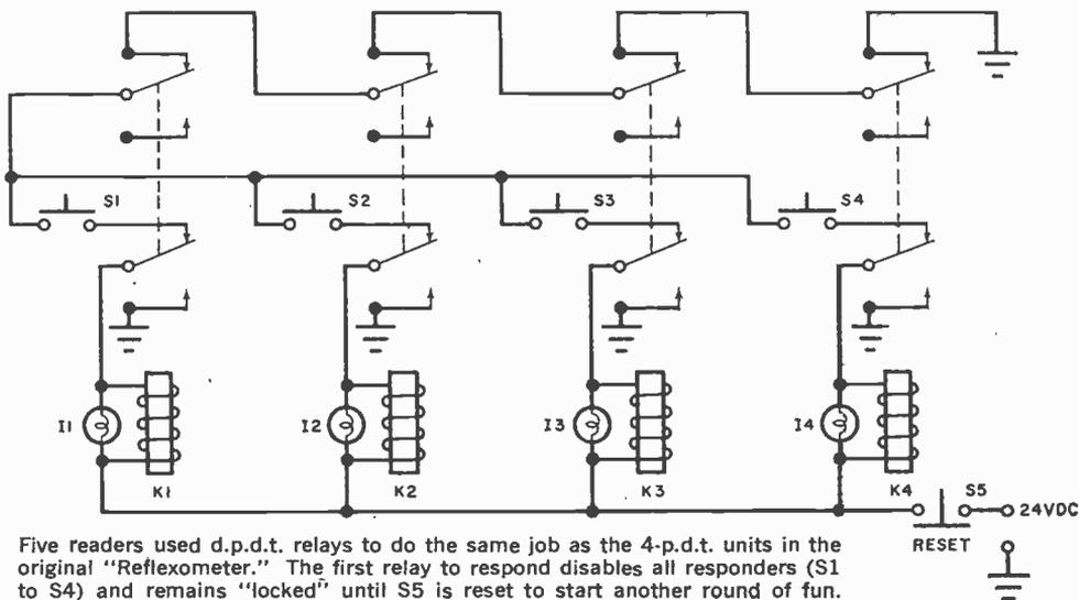
Five readers used d.p.d.t. relays to do the same job as the 4-p.d.t. units in the original "Reflexometer." The first relay to respond disables all responders (S1 to S4) and remains "locked" until S5 is reset to start another round of fun.
