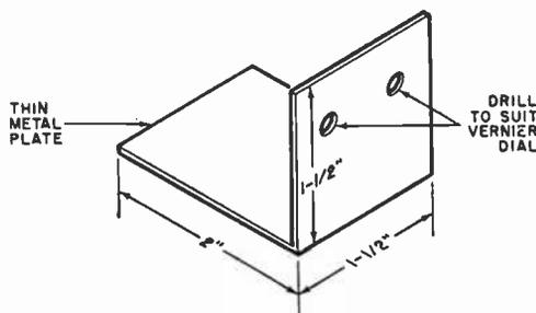
slipping the vernier dial over the bandspread or fine tuning shaft. You'll be pleasantly surprised by the change in tuning ease.
