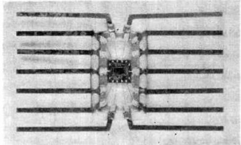
Ceramic flat pack is used when maximum miniaturization is required. It occupies less than half the space of a TO-5 transistor package. This configuration sometimes replaces as many as 50 components.
