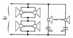
Hookup shown is for an amplifier's 8-ohm impedance tap. To maintain the proper phase, the top leads are connected to the terminal marked with a red dot.
