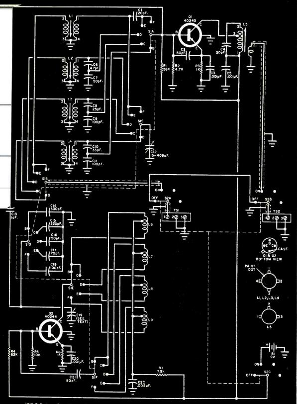
GC-2 Deluxe Converter uses two low-cost transistors in conventional circuit. Output is tuned to 3.5 MHz read barn band on the communications style receivers. Coverage is 200-400 kHz and 0.55 to 18.0 MHz.
