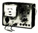
400, and also tests for transistor or diode leakage. It supplies a test signal for a.f., r.f., or i.f. circuits. In addition, it can be used as a signal tracer, measure supply voltages on a 20-volt scale, and measure circuit current drain to 100 mA. All types of transistors can be tested, in or out of circuit.
