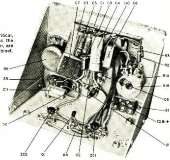
nal strip anchor the capacitors. Be particularly careful not to confuse the circuit by wiring S2 or R1 to IC1 improperly. If your project fails to operate, there's a good chance that you crossed the wires to these components. Follow the schematic and you won't have any trouble.
