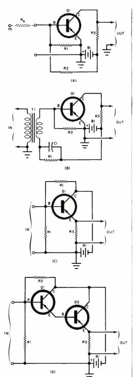
Fig. 4. Techniques that can be used to increase the input impedance of a transistor amplifier include: (A) input series resistor  $R_{\rm g}$ ; (B) step-down transformer T1; (C) a conventional emitter follower; and (D) a Darlington pair emitter follower circuit.
