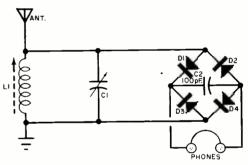
Fig. 2. Greater efficiency from full-wave detection of an AM r.f. wave is claimed by reader William H. Witt, who has submitted this TRF receiver circuit.
