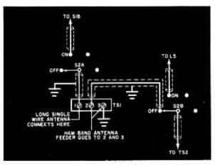
Alternative output switching arrangement will permit use of separate long-wire antenna for converter.
