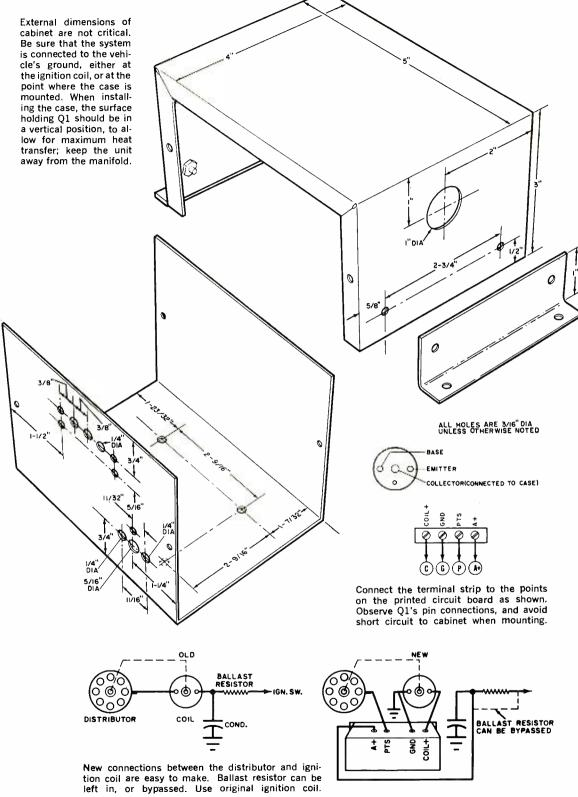
When the ignition points open, a positive pulse is applied to Q2's gate, and with the speed of a fast-acting electronic switch, typical of solid-state devices, Q2 conducts and the spark occurs. The positive pulse is developed simply enough, but the system's immunity to point-bounce is interesting.
