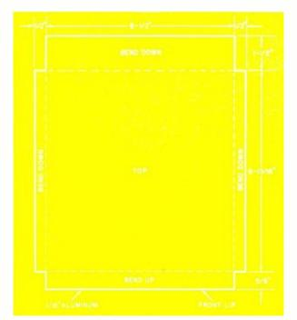
If you house the converter in the cabinet recommended by the author, a chassis must be formed from sheet aluminum as shown in the drawing above.
