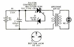
Battery-powered flashing circuit consists of only seven miniature parts. See photo on next page for layout of components. Transformer is rated with a 10,000-ohm primary winding and 16-ohm secondary.
