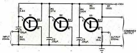
Fig. 3. Fully described in a recent application note from General Electric Company, this frequency divider employs cascaded interlocked unijunction transistor oscillator circuits (Q1, Q2, and Q3) to provide a 100:1 frequency division. Its natural operating frequency is determined by the R1, R2-C1 time constant.
