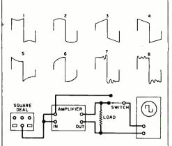
Basic waveforms. Ideal shape is shown on scope. Other shapes are: (1) loss of lows; (2) boosted lows; (3) low-frequency phase lag; (4) low-frequency phase lead; (5) combination of loss of lows and phase shift; (6) combination of loss of highs and phase shift; (7) ringing, with good damping; and (8) ringing, with poor damping.
