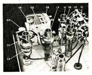
approximately 1/2" long that you can solder to after the coil is mounted. A liberal application of cement will prevent the turns from shifting, once the coils are wound.
