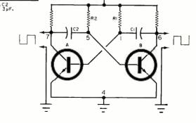
values of either or both of the capacitors or the resistors. In the actual circuit, capacitors C1 through C10 provide different frequency ranges in five decade steps from X 1 to X 10,000, and the ganged potentiometer (R1a and R1b) provides a continuously variable selection of frequencies within each range.
