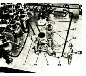
Construction. Since the large tuning dial makes it necessary to house the converter in a fairly big cabinet, there is room to spare for all components. Unfortunately, no company seems to manufacture a suitable chassis, so the builder must fabricate one from sheet aluminum. Its dimensions are shown on p. 43. Bend the front lip of the sheet aluminum upward, and the side lips and rear apron downward.
