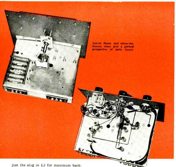
just the slug in L3 for maximum background noise. Tighten the lock nut on L3. The converter is now aligned for the broadcast band.
