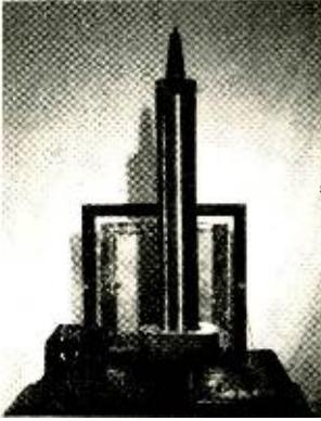
through insulator is a turned wooden piece with a large thread spool, minus the thread, placed on top of it.
