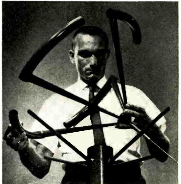
**"CIRCULAR POLARIZED LOOP VEE"**—A new type of space age antenna (photo above) has been designed and built for the U.S. Air Force by Electronic Communications, Inc. Together with its associated satellite communications terminal equipment, this odd-shaped antenna will be used in airborne applications. It radiates up to 1000 watts of power in an omnidirectional pattern to provide optimum near-horizon communications coverage.
