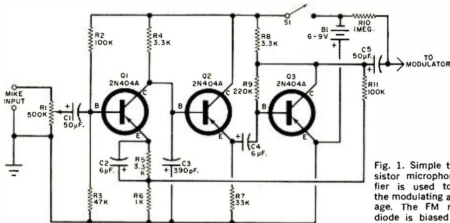
Fig. 1. Simple three-transistor microphone amplifier is used to provide the modulating audio voltage. The FM modulator diode is biased by R10.
