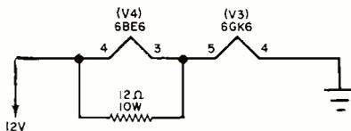
Fig. 2. Filament rewiring in NCX-3.
