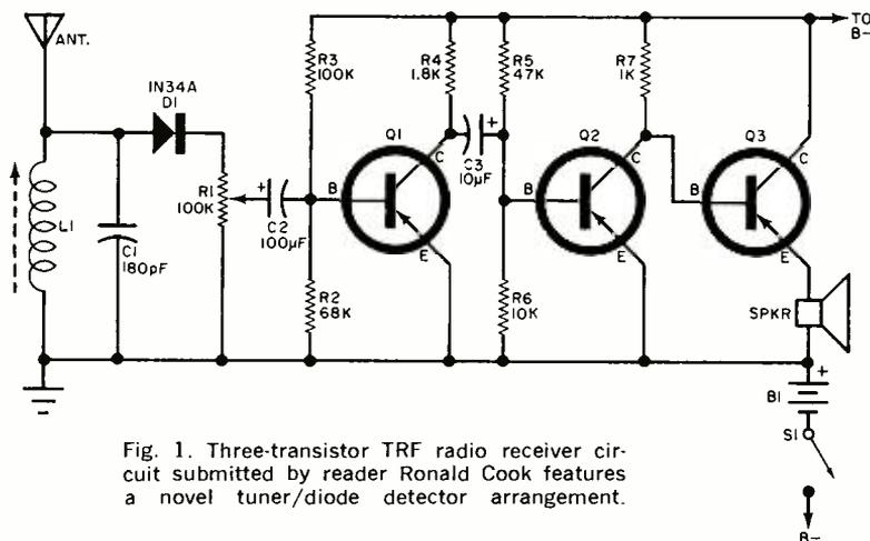
Fig. 1. Three-transistor TRF radio receiver circuit submitted by reader Ronald Cook features a novel tuner/diode detector arrangement.
