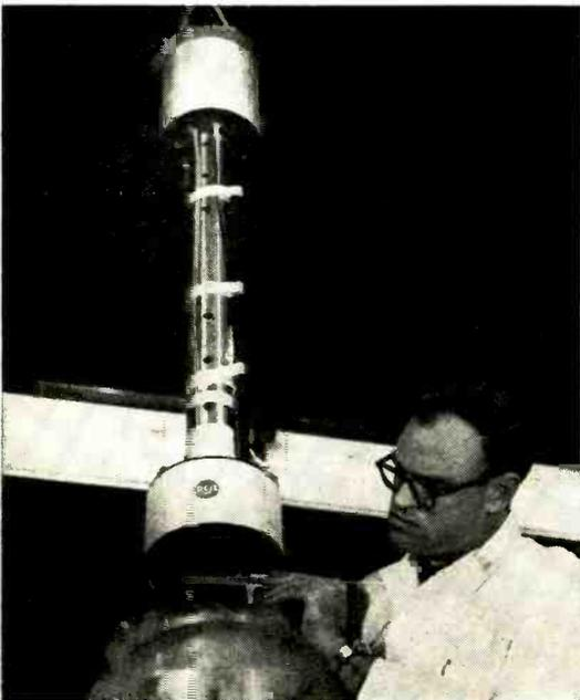
**SUPERCONDUCTIVE MAGNETS**—Pint-size magnets have been developed by RCA that can generate forces approaching those which bind matter together. The magnets are cooled in liquid helium to reduce the electrical resistance of their field windings to zero. Fields as high as 150 kilogauss are possible.
