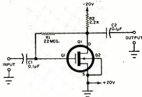
Fig. 14. Definitely not recommended for the experimenter, this single-stage preamplifier features an insulated-gate field-effect transistor (IGFET).
