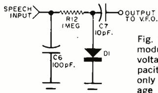
Fig. 2. Complete FM modulator, featuring voltage-variable capacitor D1, requires only a bias voltage for operation.
