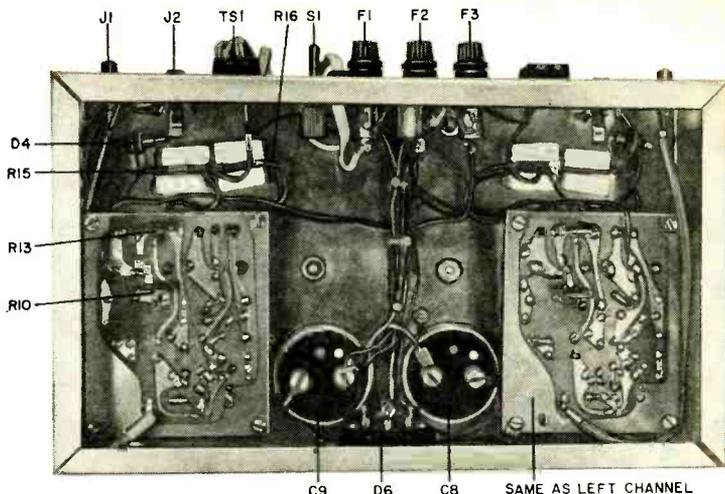
Fig. 7. If you cannot get the values specified for  $R15$  and  $R16$ , you can wire two resistors in parallel to obtain the desired wattage and resistance, as shown here. Note the almost mirror image of one channel to the other . . . they are identical.
