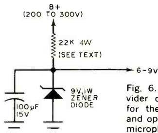
Fig. 6. This voltage divider can provide bias and operating power for the FM modulator, and microphone amplifier.
