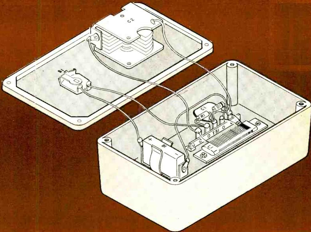
Housed in a plastic instrument case, the AMLIGNER can be assembled and wired in a matter of minutes. When wiring components to the terminal strip, be sure to observe polarity orientation of diode D1.
