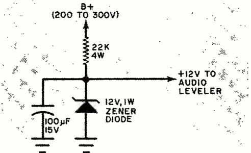
Fig. 6. This simple voltage divider can be used in a tube-type transceiver to obtain a 9-12 volt regulated output for operating the Audio Leveler.
