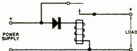
polarity, the diode conducts and causes the relay to energize, applying the full power supply voltage to the load. If the polarity is reversed, the diode doesn't conduct and the relay stays open. Use a sensitive (5-mA to 10mA), normally open s.p.s.t. relay whose contacts can handle the current drawn by the load.
