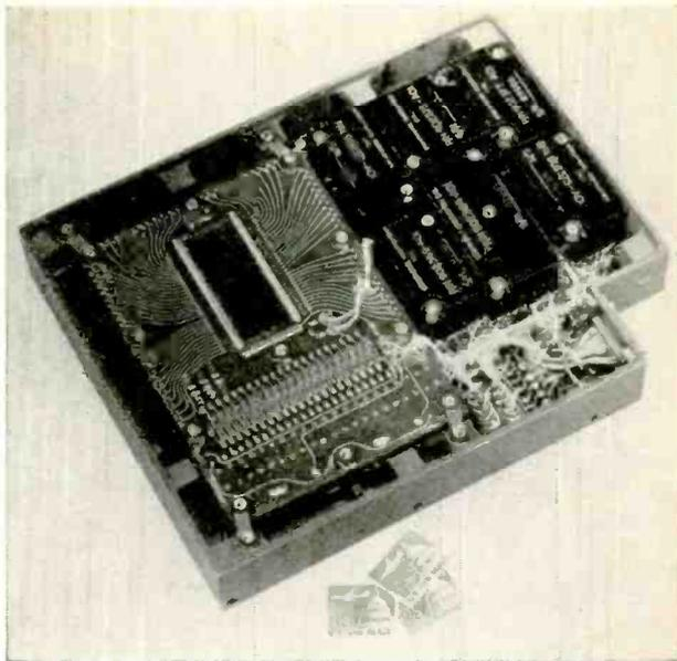
**LITTLE GUY WITH A B-I-G JOB—**A tiny memory unit built by Electronic Memories is hardly larger than 5 packs of cigarettes, yet it contains all the information needed to put Lunar Orbiter B into orbit around the moon, aim the cameras at the moon's surface and start them rolling. During Lunar Orbiter B's shuttle to the moon, the memory unit has the jobs of extending the antennas and solar panels, controlling the propulsion and attitude of the spacecraft, and starting the scientific experiments.
