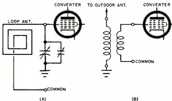
Fig. 2. In a standard BC receiver the loop antenna (a) or equivalent is replaced with a J. W. Miller r.f. coil as shown in (b). A suitable short-wave antenna must be hooked up to the coil primary for best results.
