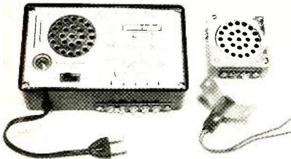
and suitable remote sensor/detectors. Designed for fail-safe operation, the unit can be employed as a burglar alarm, fire alarm, power failure alarm, or freezer failure alarm, depending on the types of sensors selected.
