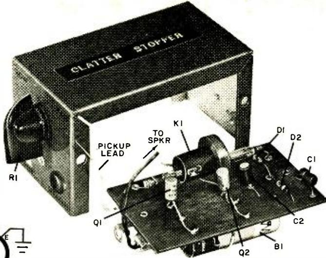
Fig. 2. Small size and few components make it possible to build "Clatter" Stopper on 2" x 3 1/2" board.
