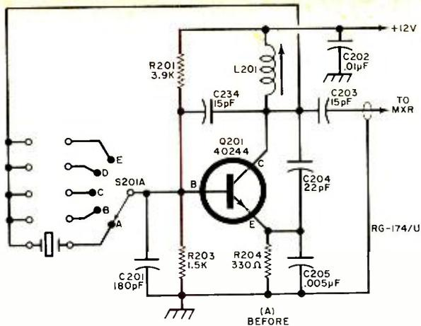
Fig. 17. These schematic diagrams show the Squires-Sanders S5S receiver oscillator before (A) and after (B) its modification from fixed to tunable service. The 22-pF capacitor (C204) and the 0.005- $\mu$ F capacitor (C205) are replaced by 5-pF and 180-pF silver mica capacitors respectively. Two other silver mica units (1 pF and 2.5 pF) are incorporated in the modified circuit.
