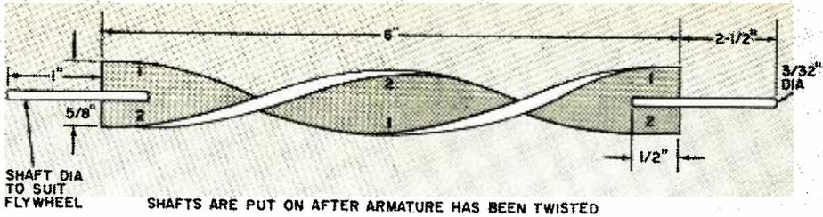
Fig. 4. The lengths of the shafts on each end of the soft iron armature should be long enough to accommodate the flywheel on one end (about 1"), and the cams and spacers on the other end (about 2½").
