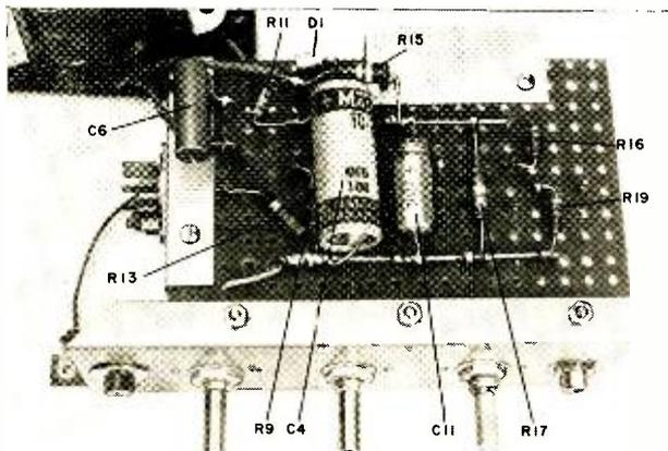
Fig. 3. Busbars eliminate the need for extra push-in solder terminals on underside of board. Solder the components directly to the busbars.
