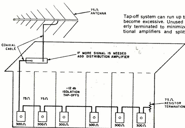
Tap-off system can run up to the point where losses become excessive. Unused outlets should be properly terminated to minimize standing waves. Additional amplifiers and splitters can be employed.
