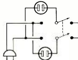
line (label this position *HI*), and in the other position both receptacles are in series (label this position *LO*), as shown. To use the speed reducer, plug the lamp or appliance into one receptacle and the power tool into the other. Set the switch to *LO* for reduced speed, to *HI* for full speed.
