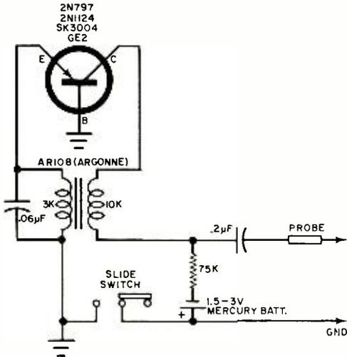
is not present when you build this circuit, simply reverse the secondary wiring connections of the transformer so that they are properly phased. This circuit is small enough to be mounted in a 35-mm. film can. The probe can be a single banana plug.
