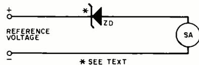
prohibits current flow until its rated voltage is exceeded. The Sonalert will sound off at any voltage from 6 to 28 volts d.c. and draws just a few milliamperes of current.
