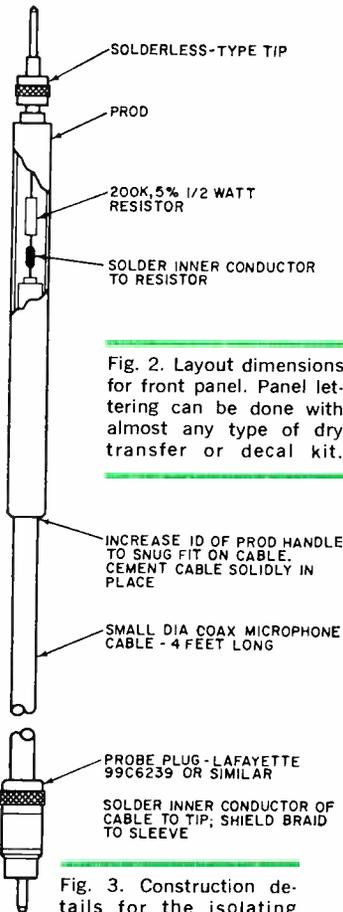
Fig. 3. Construction details for the isolating probe for use with the DCEV. These parts are not included in Parts List.
