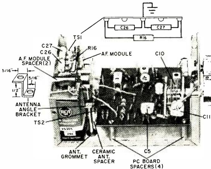
Fig. 5. Shown at left are construction details for the antenna mounting bracket and the parts arrangement on terminal strip TS1. Battery is held in place by a metal clamp.
