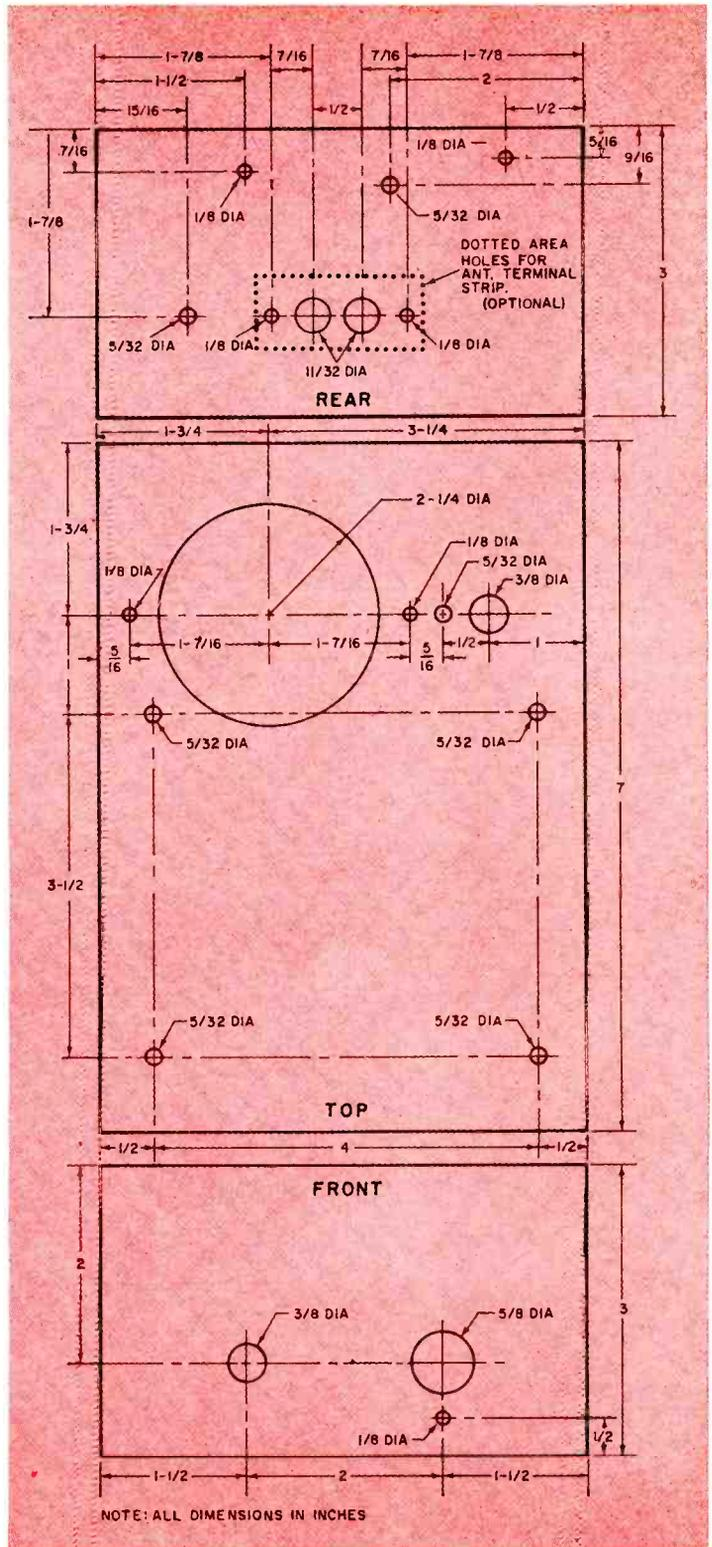
Fig. 3. To avoid unwanted interactions, mounting holes should be drilled to conform with dimensions and locations shown in the drawing (at right).
