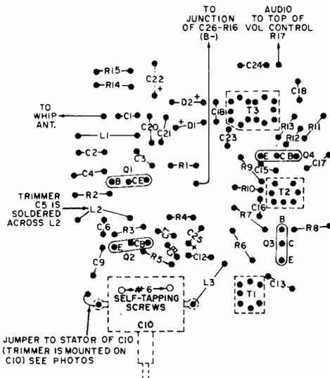
Fig. 7. When mounting capacitor *C10* on board, make good electrical contact between frame and foil.
