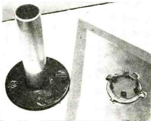
Fig. 4. Plug buttons soldered to metal plates that serve as antennas provide electrical coupling and mechanical support between antennas and pipes.
