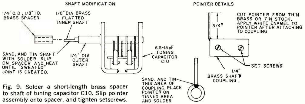
Fig. 9. Solder a short-length brass spacer to shaft of tuning capacitor C10. Slip pointer assembly onto spacer, and tighten setscrews.
