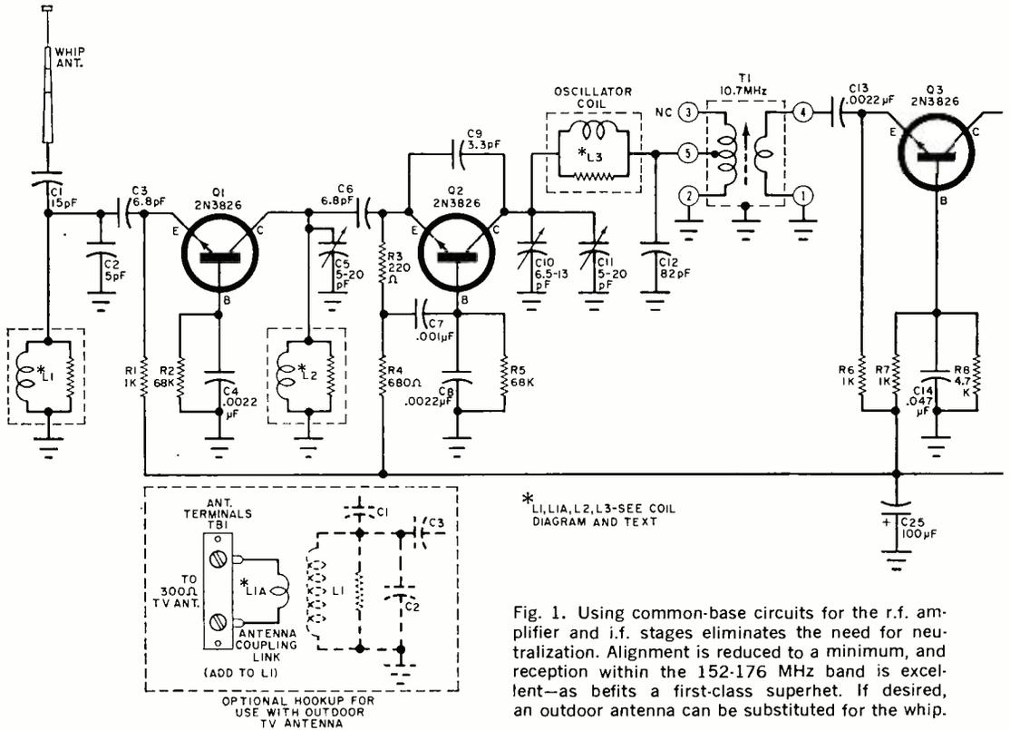
Fig. 1. Using common-base circuits for the r.f. amplifier and i.f. stages eliminates the need for neutralization. Alignment is reduced to a minimum, and reception within the 152-176 MHz band is excellent—as befits a first-class superhet. If desired, an outdoor antenna can be substituted for the whip.
