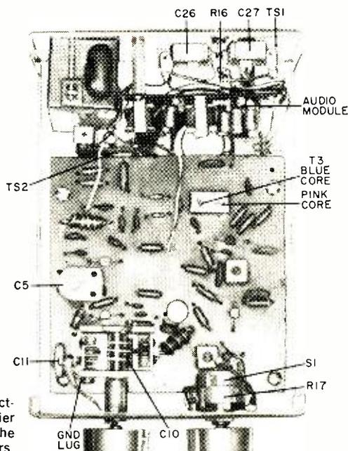
Fig. 6. Carefully orient detector transformer *T3* exactly as shown. Commercially available audio amplifier module should be mounted on the rear apron of the chassis using appropriate size hardware and spacers.
