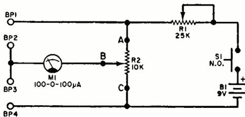
The circuit is essentially a Wheatstone bridge. Potentiometer *R2* must be set for the same voltage drop on both sides of point *B*; *R1* simply functions as a sensitivity control. Resistors to be matched are connected to *BP1*-*BP2* and *BP3*-*BP4*, respectively.
