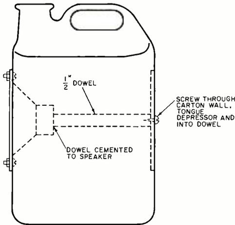
Dowel is cemented to speaker and screwed to rear wall of jug to insure maximum enclosure rigidity.
