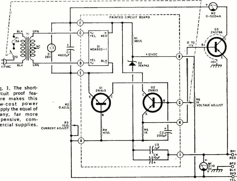
Fig. 1. The short-circuit proof feature makes this low-cost power supply the equal of many, far more expensive, commercial supplies.
