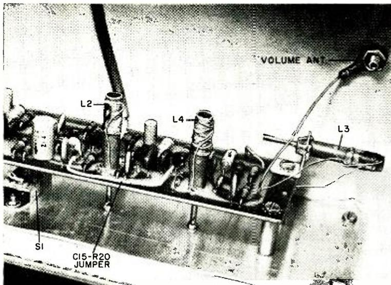
circuit consisting of  $L4$  and  $C22$ . The r.f. signal across this second tuned circuit is rectified by diode  $D1$  and applied to the base of d.c. amplifier  $Q5$ . Thus, the d.c. voltage level present at the collector of  $Q5$  is a function of the amount of r.f. present on  $L4-C22$ . This level is at its maximum when the  $L4-C22$  tuned circuit is at the same frequency as the  $Q4$  collector tuned circuit.
