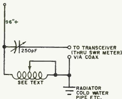
can be used (depending on frequency). Adjust the coil tap and tune the variable capacitor for lowest reflected power. A collapsible whip antenna can be employed, provided that it is 96 inches or longer. The coil is made of 30 turns of #14 wire, 8 turns per inch, 2 $\frac{1}{2}$ " in diameter.
