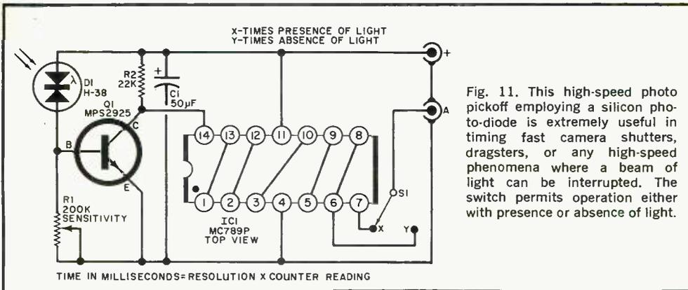
Fig. 11. This high-speed photo pickoff employing a silicon photo-diode is extremely useful in timing fast camera shutters, dragsters, or any high-speed phenomena where a beam of light can be interrupted. The switch permits operation either with presence or absence of light.
