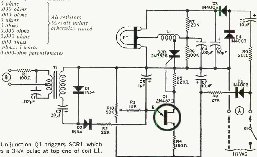
Fig. 1. Unijunction *Q1* triggers *SCR1* which produces a 3-kV pulse at top end of coil *L1*.
