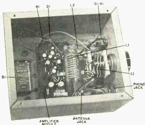
Use a metal chassis to house the monitor circuit and provide shielding against external noises and r.f. interference. Parts layout is not critical.
