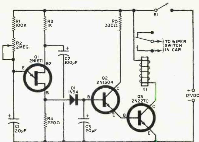
Each time relay K1 closes, it allows the wiper to make one full sweep, at full torque, before returning to its rest position.
