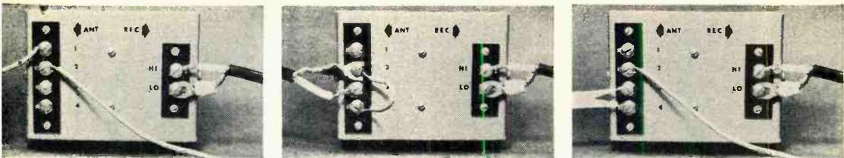
Fig. 5. The three methods of connecting an antenna to the preselector. At left, a single-wire lead-in is connected to ANT terminal 1 and a ground to terminal 2. In center photo, a coax-fed antenna is connected to terminal 3 and the shield connected to terminals 2 and 4. At right, a balanced 300-ohm twin-lead input is connected to terminals 3 and 4. A ground connection from terminal 2 is optional.
