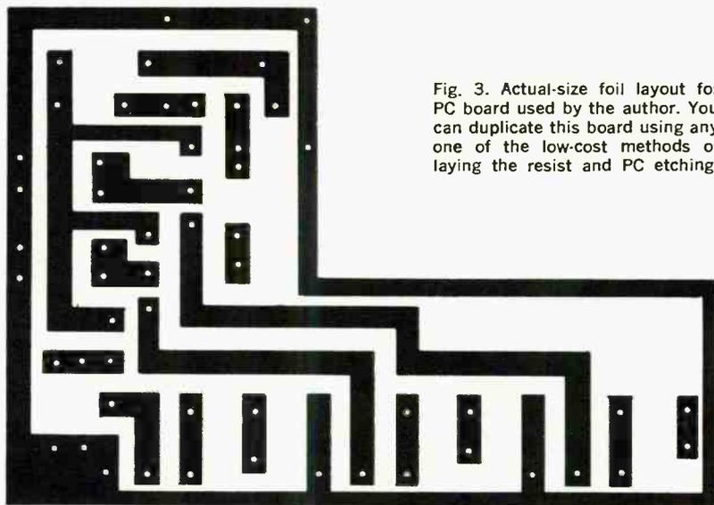
Fig. 3. Actual-size foil layout for PC board used by the author. You can duplicate this board using any one of the low-cost methods of laying the resist and PC etching.
