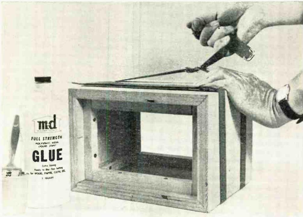
sets. One of the most convenient methods of applying pressure is to use two 48-inch canvas straps. When tightened, the straps force the sides into position for a perfect fit.
