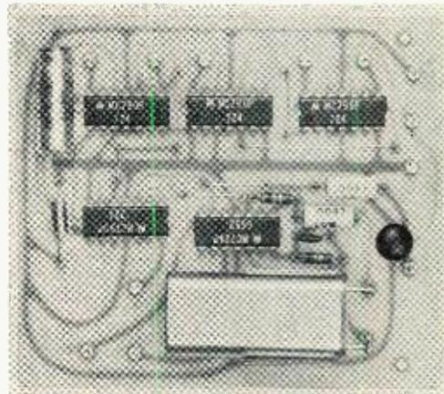
Top view of the timing module PC board with all components mounted. Connections to the board are made via the PC terminals affixed to the board.
