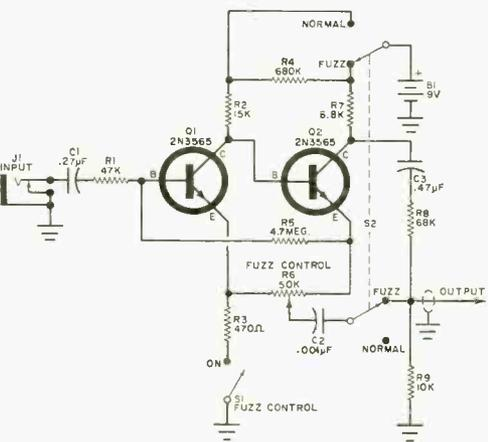
of *R6* and FUZZ/NORMAL switch *S2* should be broken and capacitor *C2* inserted as shown above.
