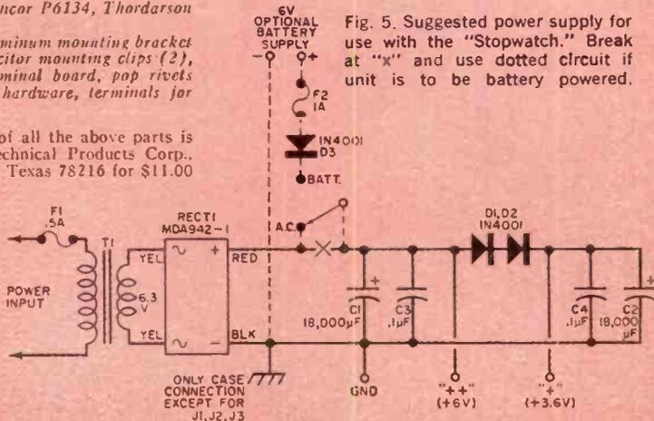
Fig. 5. Suggested power supply for use with the "Stopwatch." Break at "x" and use dotted circuit if unit is to be battery powered.
