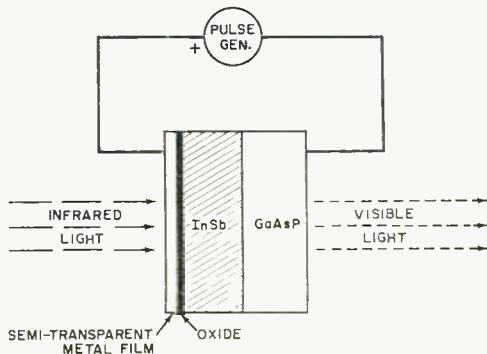
Fig. 2. This American development is a solid-state infrared-to-visible light converter that could lead to many new camera concepts, techniques and applications.
