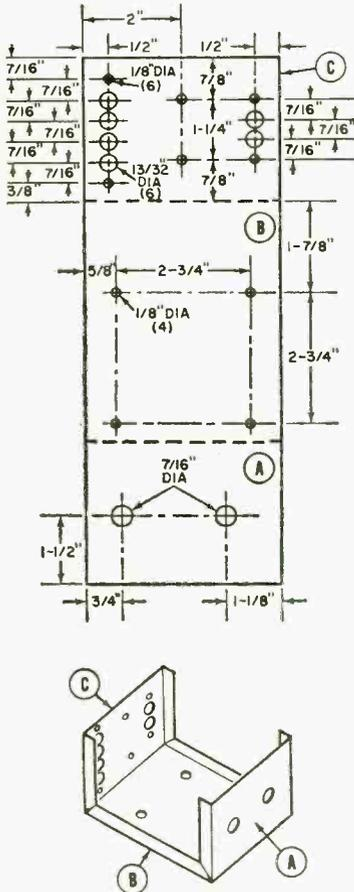
the solder lug to the box surface with a 4-40 screw and nut to make a solid ground connection to the box. Scribe a minus (-) sign near the bottom left
