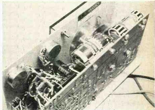
This less-than-\$20 transistorized VOM is expected to usher in a new era of portable test instruments. Test leads are permanently wired to the VOM—one lead for grounding, one for d.c. volts, a third for a.c. volts and ohms. The VOM is housed in special tough plastic case. Two batteries are required to power the solid-state circuit. Assembly takes about four hours. The IM-17 features a panel-mounted polarity-reversing switch.
