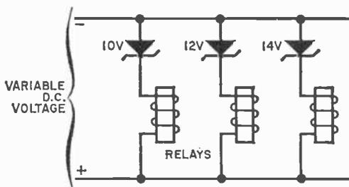
voltage goes up, each zener will conduct at its voltage and close its associated relay. You can select the zeners and relays for almost any range of d.c. voltage required.
