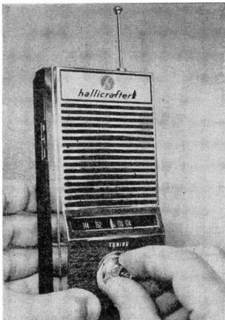
quency (police, fire, CAP, ham, weather, etc.). If this distinction between types of receivers is accepted, the user will find that the portable has many advantages. For example, frequency drift is eliminated, battery life is usually very long, and the handiness of taking the receiver with you (if only from room to room) cannot be denied.
