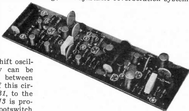
Transistor *Q6* is in a phase-shift oscillator circuit whose frequency can be varied (by speed control *R30*) between 4 and 15 Hz. The a.c. output of this circuit is fed, via level control *R31*, to the gate of *Q5*. Open-circuit jack *J3* is provided so that an external footswitch can be used to turn on the tremolo if desired.
