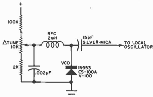
the variable capacitor diode used) may be necessary. Delta tuning is accomplished by varying the value of the 10,000-ohm potentiometer.
