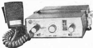
an illuminated "S"-meter and channel selector switch, p.a. function with separate jacks for p.a. and remote speakers with  $3\frac{1}{4}$ -watts of audio, a squelch control, and a noise limiter. Sensitivity is  $0.35 \mu\text{V}$  for 10 dB signal-to-noise plus noise at 40% modulation. Crystals for operation on all 23 channels are included.
