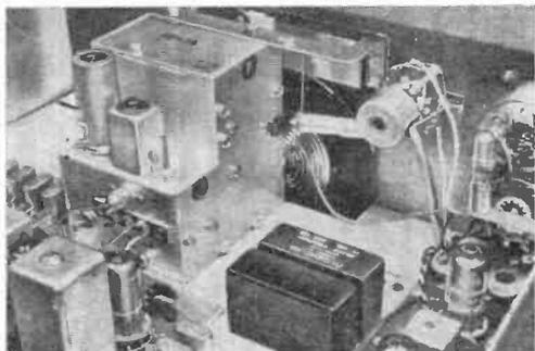
Inside the SB-310, the two black rectangular boxes are the special filters that permit optimum selectivity on both international broadcast and ham bands. Tunable linear oscillator is at upper left.
