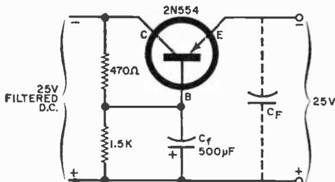
equal to  $C_f H_{FE}$ , where  $H_{FE}$  is the current gain of the transistor being used. In the example shown, the effective  $C_F$  is about 25,000  $\mu$ F.
