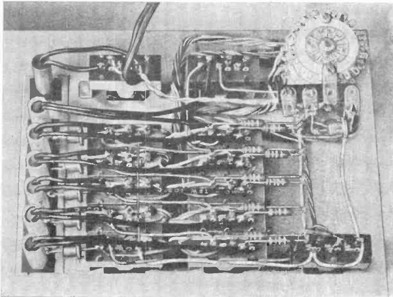
Overall interior view of the Binary Adder is shown at the left. The four photos surrounding this view identify the various components within the circuit. Note the alignment of each A and B Operand switch with its associated Result Register readout indicator.
