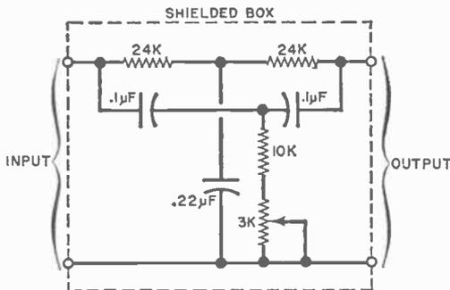
series with the signal lead and adjust the potentiometer for maximum 60-Hz rejection.
