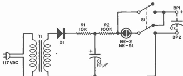
Fig. 2. Reader Eugene Richardson's capacitor tester has visual readout.
