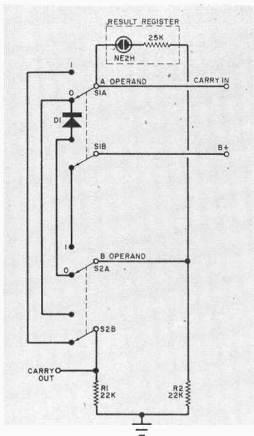
Fig. 1. This basic one-bit adder circuit shows how the Binary Adder operates.
