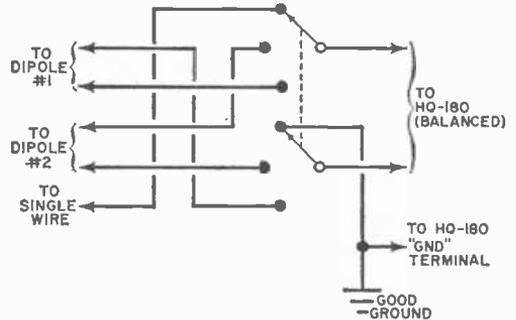
likely, we would suggest a 2-gang switch (it's easier to work with) such as the Malory Type 1325L. You will then have extra positions available in case you decide to add another receiver or another antenna to your setup. Wire the switch according to the diagram above (we are assuming that you have 300-ohm twin-lead dipoles).
