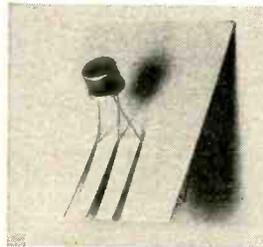
transistor being mounted (the prongs of the heat sink should clamp onto all three transistor leads simultaneously). However, if you design your own printed circuit boards and take care to maintain all transistor and
