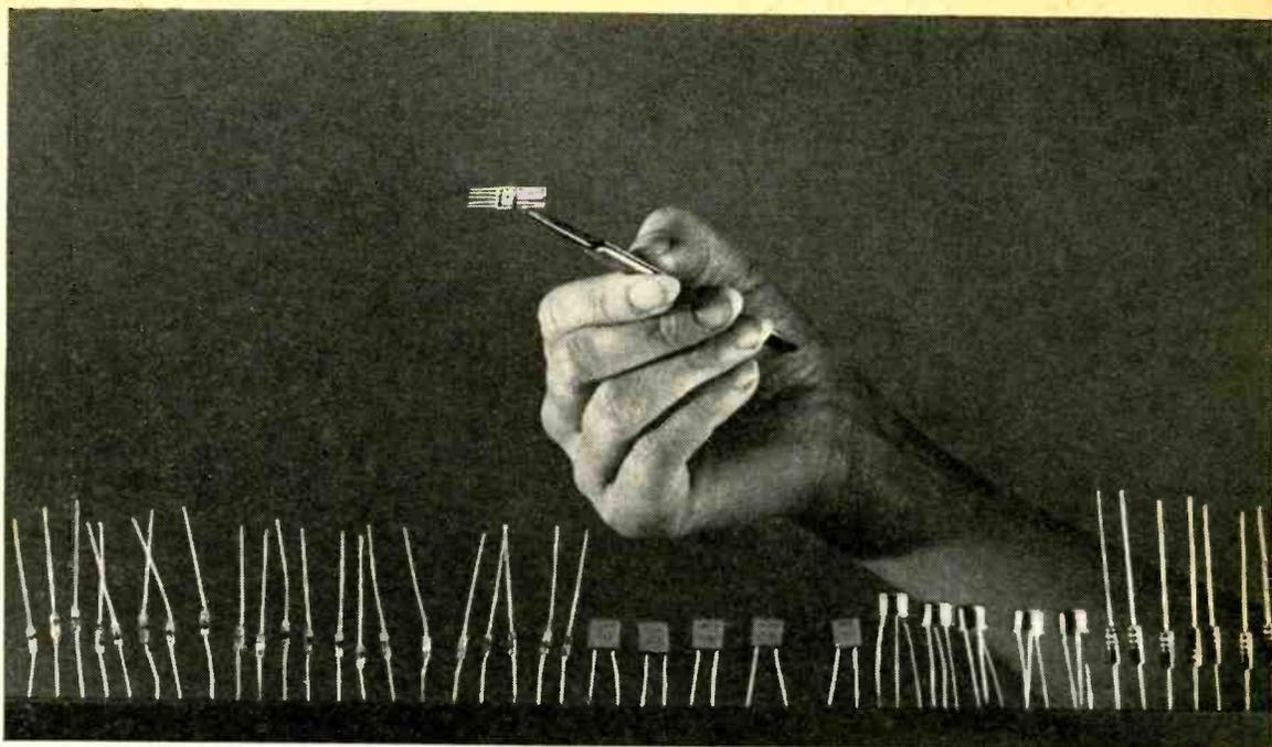
*50 functions in a single chip. The functions of 50 separate transistors, diodes, resistors and capacitors can now be formed by the tiny dot in the center of the integrated circuit held by the tweezers.*
