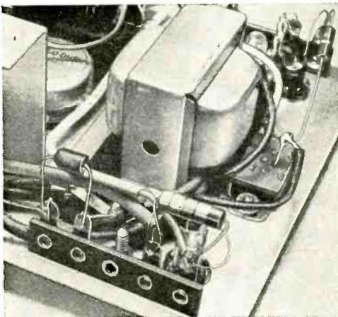
Terminal strips are used to support components and also act as tie points for the point-to-point wiring.
