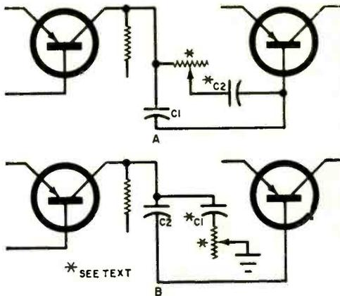
bass attenuation circuit and (b) a treble attenuation circuit. In circuit (a), the value of coupling capacitor  $C1$  is made much smaller than normal, and  $C2$ 's value can range from 1 to 25  $\mu\text{F}$ . The potentiometer value can vary from 2000 to 25,000 ohms. In circuit (b),  $C2$  is the normal value, but  $C1$ 's value can range from 0.02 to 1  $\mu\text{F}$ . The potentiometer for circuit (b) can be in the 3000- to 75,000-ohm range.
