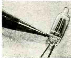
carefully examining the glass bases of the individual lamps, you'll find the lamp number on one of the flat surfaces (see photo); the other flat surface has the initials "GE" stamped on it,
