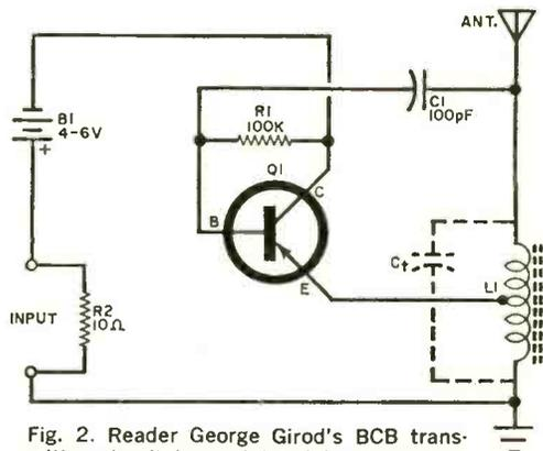
Fig. 2. Reader George Girod's BCB transmitter circuit is modulated by the output signal from a TV audio output transformer.
