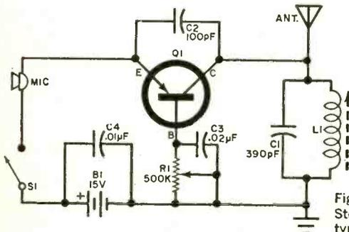
Fig. 1. The BCB circuit submitted by Steve Trospser is a common-base Colpitts-type oscillator, modulated by a carbon mike.
