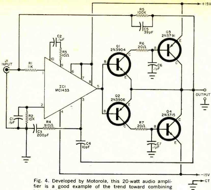
Fig. 4. Developed by Motorola, this 20-watt audio amplifier is a good example of the trend toward combining integrated circuits and discrete power output transistors.
