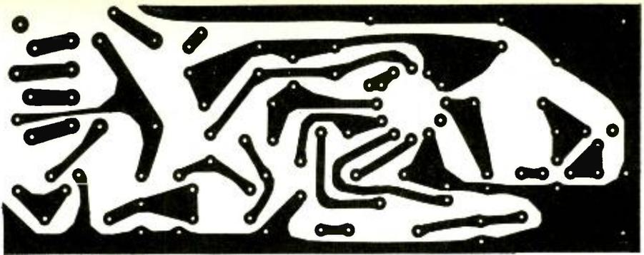
Fig. 2. This actual-size PC board foil layout should be made on a glass-epoxy board, rather than paper-phenolic, to reduce the possibility of poor operation due to stray leakage paths.
