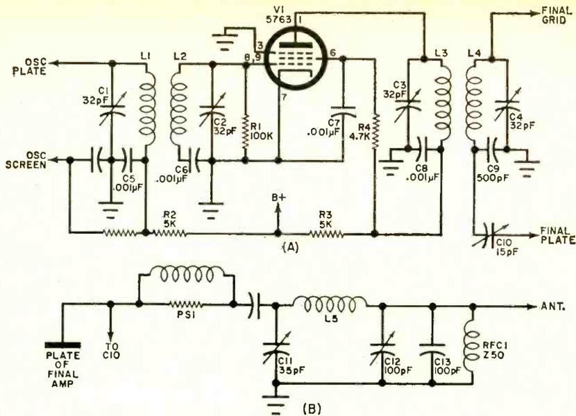
Fig. 1. Circuit (a) is added between oscillator and final. The new output network appears at (b).
