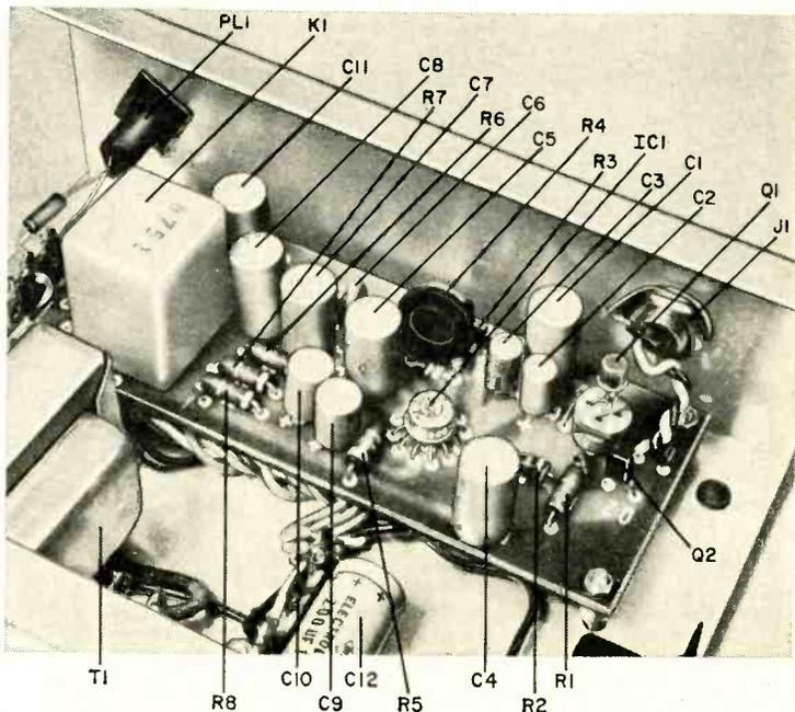
The neat layout within the device contributes to its excellent operation. Unidentified resistor at far left is the current-limiting resistor selected for operation of the neon lamp (PL1). The relay shown here is a Price Electric 226-24P (furnished with kit), although any other 12-volt, 40-mA coil d.p.d.t. relay can be used with external wiring from the PC board.
