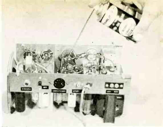
The next step is to remove oxide scale from switch contacts and dirt from inside potentiometers. This can be accomplished by spraying a good quality contact or pot cleaner into the respective devices and rotating the shafts several times to make sure good electrical contact is obtained. Repeat this process several times to obtain desired results.
