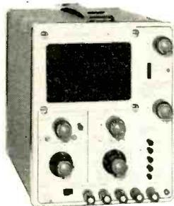
"Telequipment" oscilloscope line designed and manufactured in England. Triggered sweep is one of the most important features of the S54, and calibrated vertical voltage and horizontal time are accurate within 5%. The S54 has a 6-cm. x 10-cm. rectangular CRT, P31 phosphor, and 4-kV ac-
