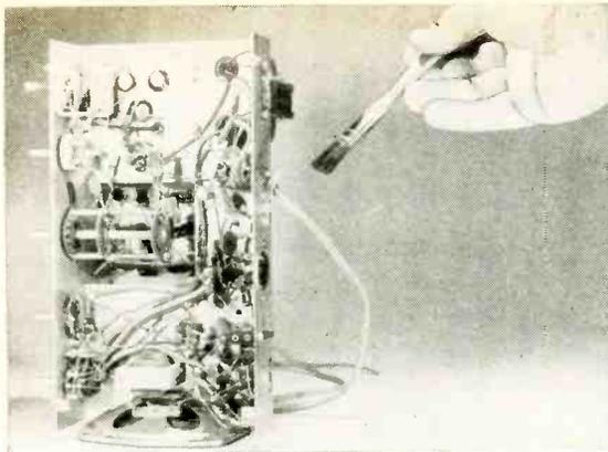
Restoration begins with a thorough cleaning of the chassis, using a small brush and/or vacuum cleaner. Stubborn dirt, grease, and capacitor electrolyte are easily removed with carbon tetrachloride—pitch with kerosene or benzene. While cleaning the chassis, be on the lookout for heat-scarred and broken components, frayed wires, and cold solder connections.
