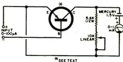
10,000-ohm potentiometer is adjusted for transistor gain variation. Beginning with a few divisions above zero, the accuracy of the microammeter will be close to 3% if the milliammeter is a 2% unit. Transistor types that can be used are: 2N408, 2N109, 2N270, or 2N407.
