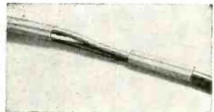
slip pre-cut lengths of plastic soft drink straws over the bundle of wires. Depending on how much flexibility you require from your homemade harness,
