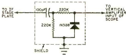
stage just before the detector in your set. A demodulator probe you can use is diagrammed here.
