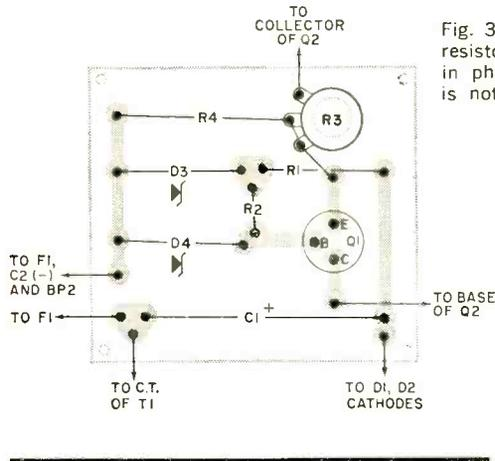
Fig. 3. Parts layout on the PC board. The 10-watt resistor R4 is suspended by its leads and is not in physical contact with the board. This resistor is not called out in photo, but is clearly visible.
