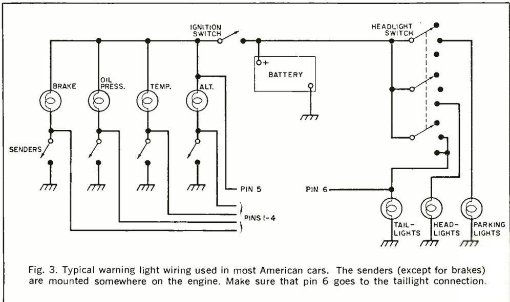
Fig. 3. Typical warning light wiring used in most American cars. The senders (except for brakes) are mounted somewhere on the engine. Make sure that pin 6 goes to the taillight connection.
