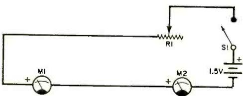
Fig. 3. When checking linearity of converted meter, pointers of both meters should move proportionally.
