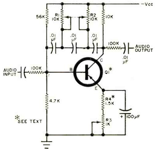
and base of  $Q1$ . With the values shown, the frequency can be "tuned" a hundred cycles or so around 650 Hz. Other values will produce a different tuning range. Make sure that  $R1$  and  $R2$  are ganged. Emitter potentiometer  $R3$  determines the sharpness of response curve. Any transistor having a beta greater than 50 can be used. Select a value for  $R4$  so that the circuit will not oscillate when  $R3$  is set for minimum bandwidth (sharpest tuning).
