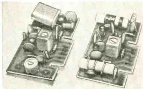
Plug-in printed circuit "cards" contain the r.f. circuits fixed-tuned to various frequencies. Card at left is set for CHU on 7.335 MHz and the card at right is tuned to the weather 162.55-MHz channel.
