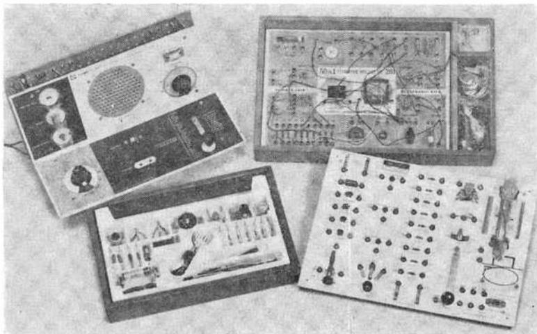
Most of the projects in the instruction manual are radio receivers or radio-oriented circuits. Projects are set up with the aid of a plastic frame and individual component cubes. All cubes (except one large block containing a tuning capacitor and loopstick antenna) measure  $\frac{3}{8}$ " on a side. Component symbols and number
