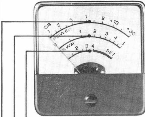
1. Built-in SWR bridge lets you tune your antenna for maximum output.
