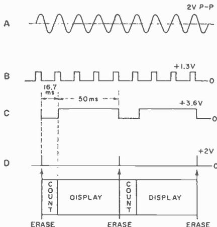
The 0, 1, overrange counter, IC5, has two flip-flops. One is a binary divider; the second is a latch that goes on when full scale is reached, regardless of how many more counts arrive. This counter takes the output of the ten's DCU and converts what would be an 0-99 display into an 0-199 plus overrange capability.
